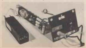
Veropins are used for mounting the components in position and small holes should be drilled where indicated to accommodate these pin's.
