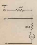
Fig. 1. A two range voltmeter. The numerical value of the current (in milliamps) gives the voltage value being measured.
