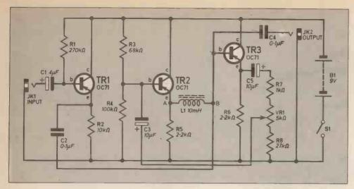
Fig. 2. The complete circuit diagram of the waa waa unit.
