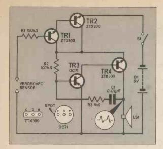
Fig. 1. Circuit diagram of the rain warning alarm.
