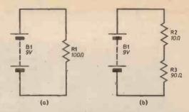
Fig. 4. The power dissipated in R1 is greater than in each of R2 and R3, but the total power dissipated in each circuit is identical.
