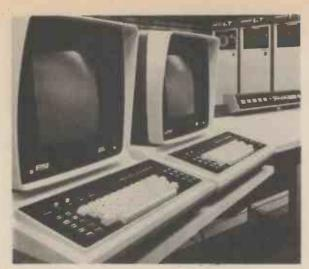
A pair of visual display units are shown here against a background of magnetic tape drives. Information is shown on the face of a cathode ray tube, as in a television set. (Burroughs Machines Ltd.)
