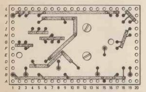
Fig. 3(b). Positioning of Cir-kit wiring on underside of board.
