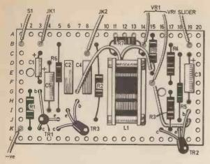
Fig. 3(a). Component layout on top side of board.
