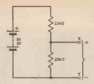
Fig. 2. Circuit for demonstrating voltmeter sensitivity.
