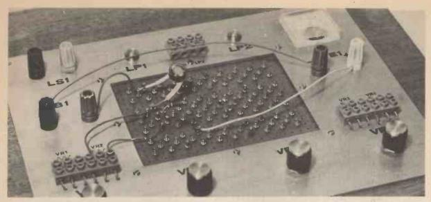
meters so now we will use the Demo Deck to make a simple version of this. Fig. 8 shows the circuit. It is a simple ohm meter where the ORP12 is a resistor whose ohmic value we shall be constantly observing.
