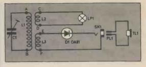
Fig. 1. Complete circuit diagram of the Radio Control Monitor.
