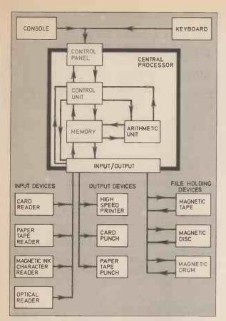
This illustrates the general organisation of a typical computer system. Major data and control paths are indicated. A system may use some, or all of the input and output devices, and in the case of the file holding devices, the system may utilise a number of each type.
