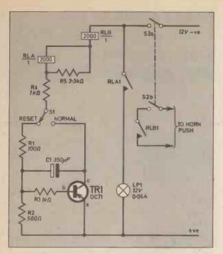
Fig. 1. Complete circuit diagram of the Auto Alert. S1 is the push button or footswitch that resets the unit.
