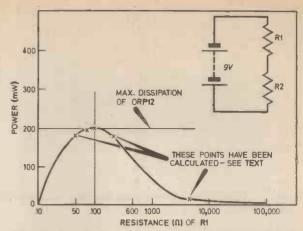
Fig. 7. Graph showing the power dissipation in R1 for various values of resistance with R2 held constant at 100 ohms. This is a maximum when R1 = R2.
