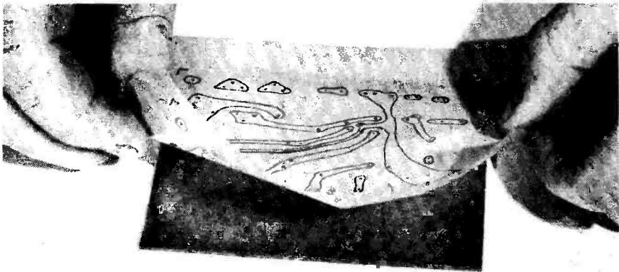
Fig. 4. Place the film down on the copper side of the p.c. board.
