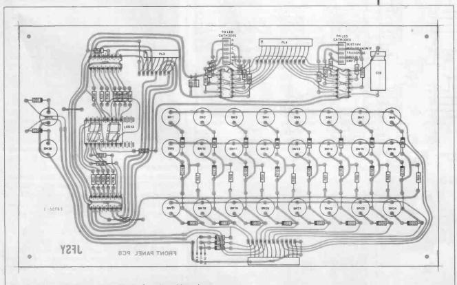
Fig. 10 The component overlay for the front panel board
