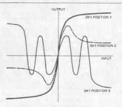
Fig. 1 The three selectable input/output characteristics of the Hyper-Fuzz
