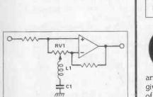
Fig. 2 An example of the type of filter element used in many graphic equalisers
