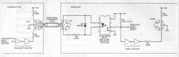
Fig. 5 The major circuit elements of a MIDI transmitter and receiver
