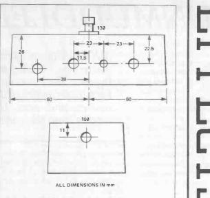
Fig. 3 Drilling the case for the Hyper-Fuzz
