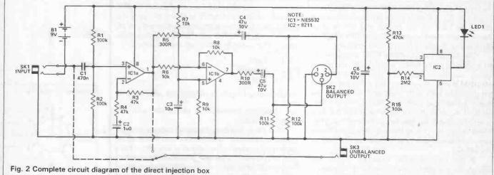
2 can be achieved by making a few component changes. The unit operates from a single 9V battery and powers up automatically when a jack plug is inserted into the input socket. In addition, a lowvoltage detector is included which lights an LED when the battery needs replacing.
