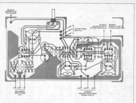
Fig. 12 Component overlay of the input stage and main signal path PCB
