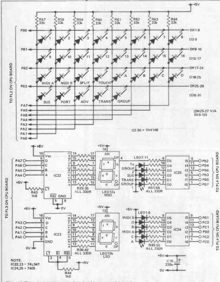
Fig. 12 The circuit diagram for the front panel board
