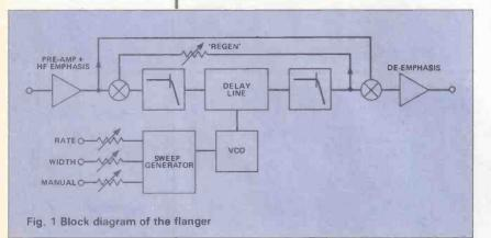
requires clock frequencies in the range 19.69kHz to 356kHz. Again there is a low-pass filter both before and after the BBD to deal with harmonics and noise.
