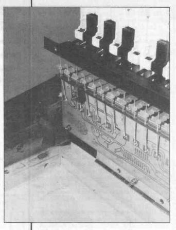
the three PCBs in place. The stand-off height of the PCBs is important since it affects the keyswitch action. In the prototype, the stand-off height was about 8mm (see Fig. 5 for details of assembly) but a different height may be required depending on the dimensions of the keyboard mechanics.
