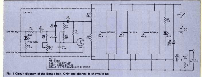
drum output is mixed to a common volume control and taken to a standard <sup>1</sup>/4in jack socket for connection to an amplifier.
