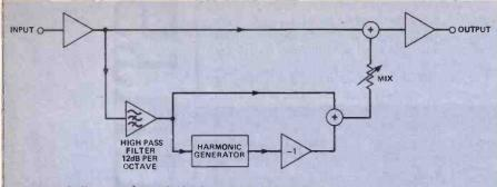
Fig. 3 Block diagram of practical enhancement arrangement
