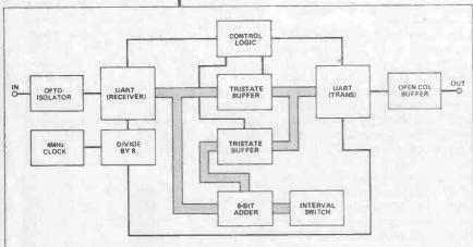
Fig. 1 The block diagram of the harmoniser
