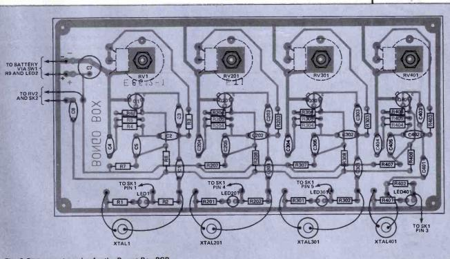
Fig. 2 Component overlay for the Bongo Box PCB
