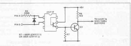
Fig. 7 CNY17 opto-isolator arranged as a non-saturated current switch for optimum performance
