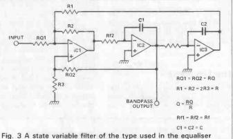
is the *parametric*. This is an equaliser in which the three main parameters — amplitude, frequency and Q — are continuously variable.
