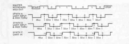
Fig. 6 Timing diagram of a single MIDI byte through a chain
