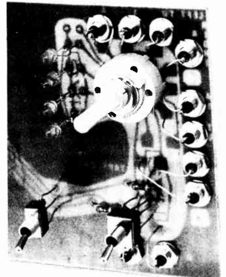
This photo shows how the input sockets are wired into the pcb.
