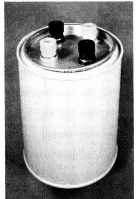
ETI-155a 4, 8 or 16 ohm dummy load (50 or 100 W) using 98 390 ohm 1 W resistors.
