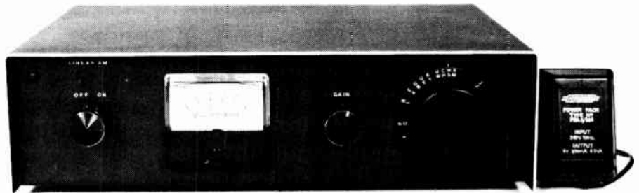
The tuner is housed in a simple, yet attractive, case. A plugpack is used to power the unit.
