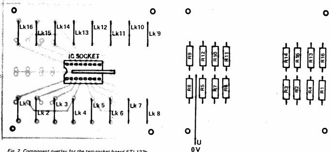
Fig. 2. Component overlay for the test-socket board ETI-123b, non-copper side.
