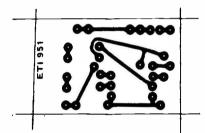
Fig. 2. The pcb design.
