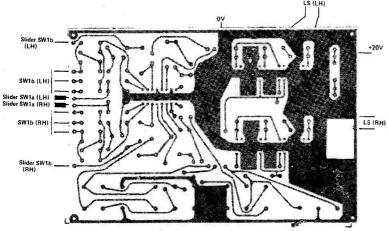
Fig. 4. The component overlay and connections to and from the circuit board.
