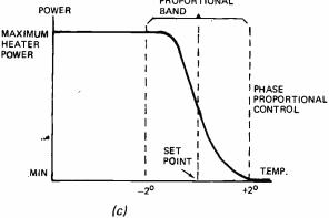
Fig. 1a. In straight on/off control the heater is ON when the load is below the set point temperature and OFF when it is above. 1b. In zero-crossing proportional control the heater power is varied linearly over a small temperature range known as the proportional band. 1c. In phase-proportional control the same proportional band is used but the control curve follows a cosine law. (Power proportional to phase angle of firing point).
