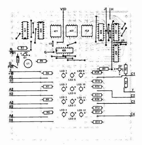
Fig. 9. Component overlay for display board.
