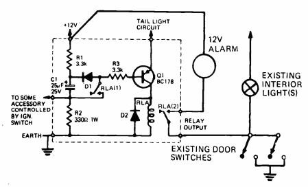
Fig. 3. How the warning circuit is wired into the vehicle's electrical system.
