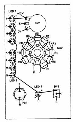
Fig. 3. Front panel wiring details.
