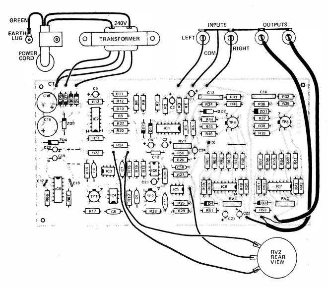
Fig. 2. Component overlay (not full size)
