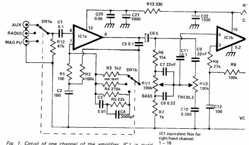
Fig. 1. Circuit of one channel of the amplifier. IC1 is quad op-amp, CA3052, and the lead-outs for the other channel are different as shown. R13, R14, C20, C21 and C22 are common to both channels.
