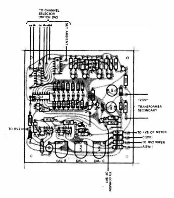
Fig. 3. Component overlay.
