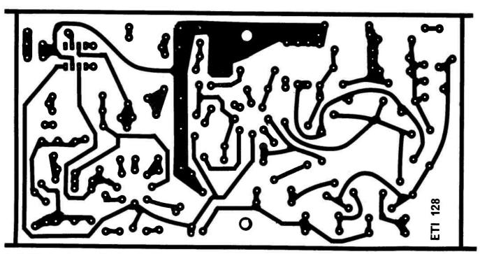
Fig. 5. Printed circuit layout. Full size 170 x 87 mm.
