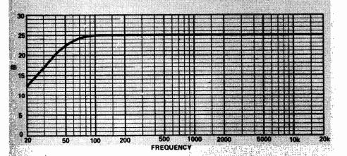
Fig. 4. Response of charge amplifier. Roll off at low end is designed to compensate for tains response of cartridge in this area.
