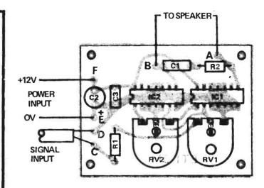
Fig. 3. Component overlay.
