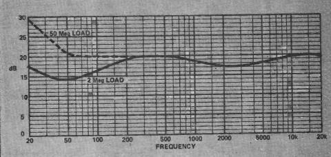
Fig. 2. Response of Decca Deram showing effect of terminating impedance at low and and of mechanical equalization at top end.
