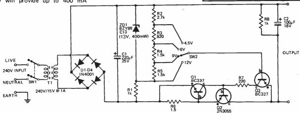
Fig. 1. Circuit diagram of the regulated power supply.
