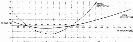
Fig. 7. Comparison of errors for copper/con and iron/con thermocouples calibrated at ambient and 100°C.
