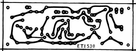
Fig. 7. (Above) Printed circuit board, common to all controllers described, has full size dimensions of 120 x 41mm.
