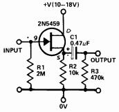
Fig. 7. Circuit of FET follower used to obtain the responses shown in Fig. 2.
