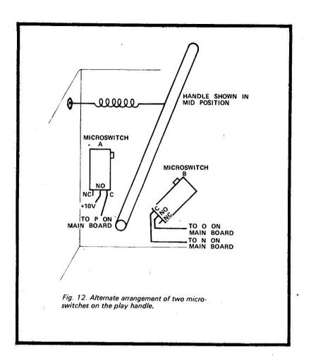
The play handle may be fashioned from a piece of 6 mm metal rod, formed into an 'L' and fitted with a wooden handle (a file handle is just right). The handle should be passed through holes drilled in either side of the box and held in position by split pins or small collars and grub screws.
