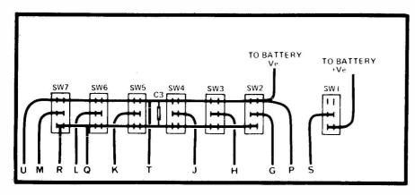
Fig. 5. Switch interconnection diagram. Note that C3 is mounted across one of the switches.
