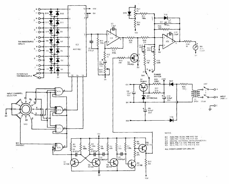
Fig. 1. Circuit diagram of the thermocouple meter.
