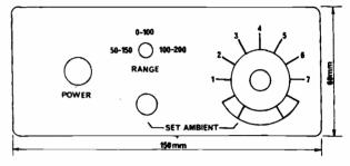
Fig. 4. Front panel artwork (half scale).
