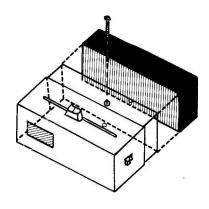
Fig. 10. How the meter is held together —
