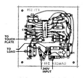
How the components are positioned on the board.
