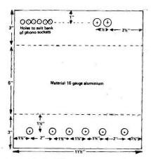
Fig. 7. Metalwork details. The front panel holes are standard %in as are the holes for the bank of phono sockets. %in holes are needed for the DIN speaker sockets.
