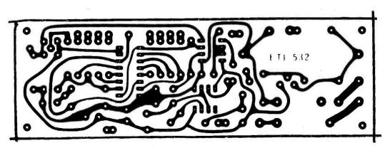
Fig. 4. Printed circuit layout. Full size 133 x 44 mm.
