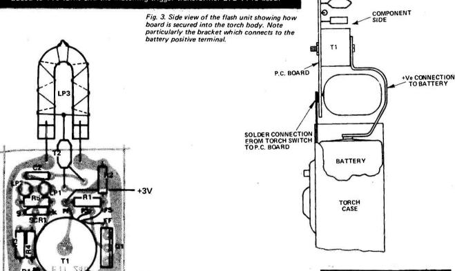
Fig. 2. Component overlay. Note copper wire spiral around flash tube.
