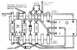
Fig. 2. How the components are connected
