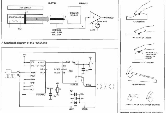
A final system implementation of the FC15A140 directly connected with the ADC, and using the rule "one clock stroke, one data". Future versions will integrate to ADC on the chip
