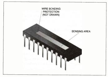
The FC15A140 FingperchipTM dil chip showing the sensing area
