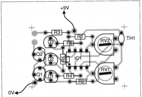
exhibit a higher forward voltage drop of around 2.5 - 3 volts. In this case, the LED will either not light or it will glow only very faintly and no other components should be required. This is a point to bear in mind should you want to build the circuit using a cheaper yellow or amber LED for D1.
