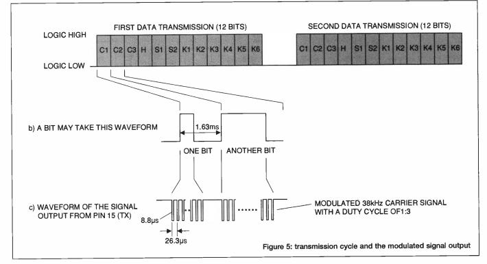
If the external resonator is 455 kHz, the period for one bit is 1.62 millisecond (a = 405 micro second). A serial data 0 and 1 are represented by different duty cycles. 0 has a 1/4 duty cycle and 1 has a 3 /4 duty cycle (**figure 6a**). As an example, if an encoded data 010100100100 is to be transmitted, the serial
