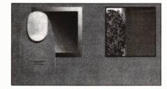
The quality of the image is analysed. Error codes flag problems like incorrect image position, no finger present or fingers that are too wet or too dry
