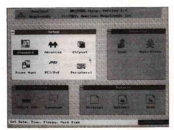
The modern AMI Setup programs can be controlled using a mouse. The "Standard" sectionis the one used to set the time, date, and so on
