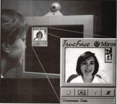
A monitor-top camera sends the image to Trueface recognition software
