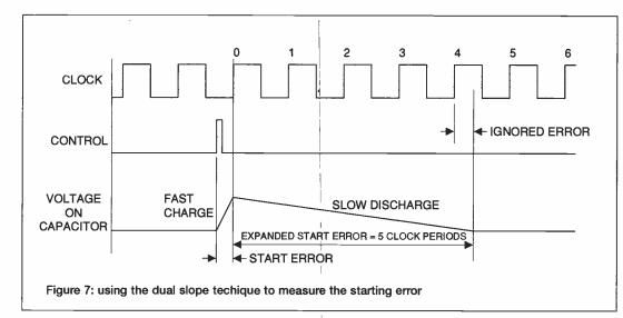
timing period the error can be ignored. The general aim for high precision timing is to make the clock period as short as possible and use a long counting chain.
