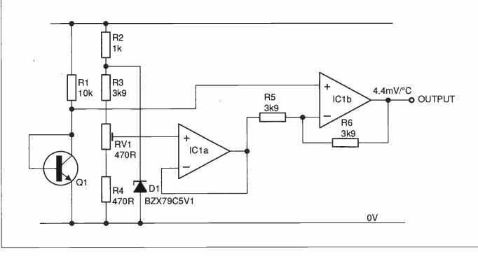
Figure 3: using a transistor as a good, low-cost temperature sensor
