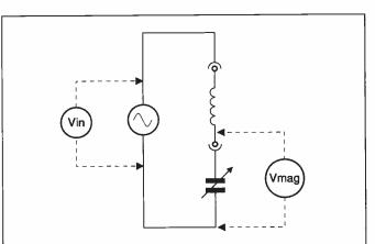
A diagram showing the basic arrangement is given in figure 1.
