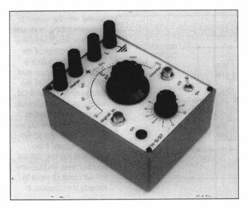
and if there are no signals present (other than the test signal from the generator), its Q can be measured while it is operating. The adapter imposes a minimal loading on the coil under test, and it is possible to observe the rise in Q with increasing amounts of positive feedback in regenerative circuits.
