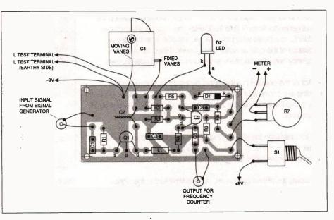
Figure 5: the front panel layout used in the prototype, approximately real size
