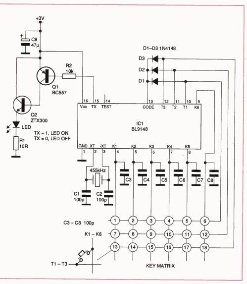
Figure 4: the circuit djagram of the remote control transmitter
