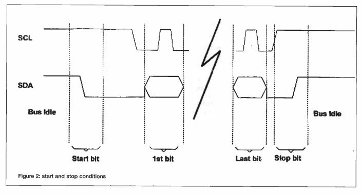
access. The slave checks the address, and if it is correct responds as defined by the master. In any transfer there will be eight bits and one acknowledgement bit sent. The acknowledgement bit is always sent by the device which is reading from the bus: if the master is transferring to the slave, the slave device acknowledges; if the slave is transferring to the master, the master acknowledges.
