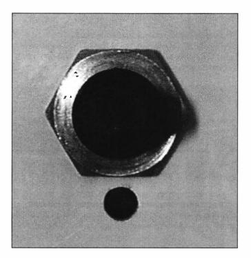
the potentiometer from rotating in use if the fixing nut worked loose and the control knob was turned hard to its limit (as happens al too easily). The whole body would then turn, and this could even result in the connecting wires breaking off. Unsecured pots work loose quite easily, and it really spoils the look and feel of a construction to have a "free floating" pot on the front panel.
