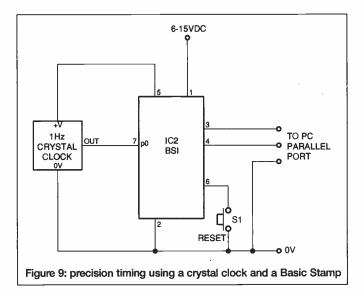
We use PULSIN to measure the length of the flash by measuring the length of the pulse received at pin p0 (**table 3**). This is a very basic Basic program with plenty of scope for expansion. To use this program the Stamp must be connected to a PC, using the special lead provided in the Stamp kit. The syntax of PULSIN is:
