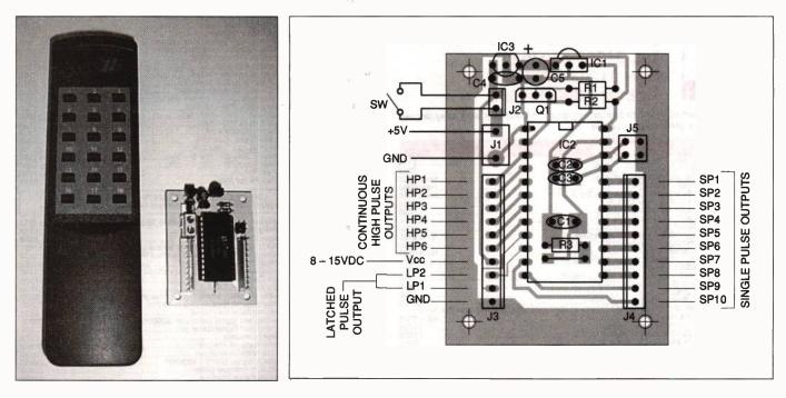
Figure 9: the handset unit with the Receiver PCB Figure 10: the component layout of the remote control receiver board
