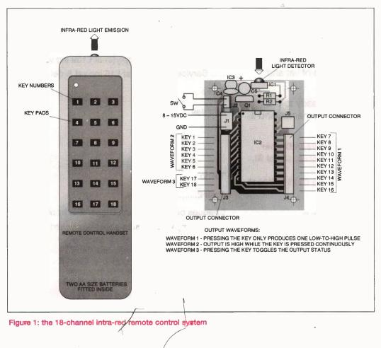
Six channels among have a *continuous high pulse* output waveform (CP, key 1 to key 6). When a button on the handset is pressed continuously, the handset repeatedly produces the infra-red emission cycle. On the receiver side, the corresponding output goes from logic low to logic high state and stays high as long as the button is pressed.
