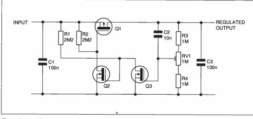
Figure 1: a very low power mosfet voltage regulator
