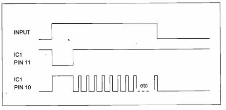
Figure 6: timing diagram given by the circuit of figure 5
