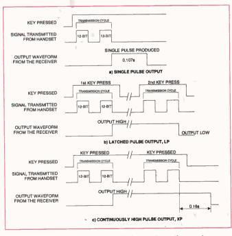
Figure 2: waveforms of the controlled outputs on the receiver board
