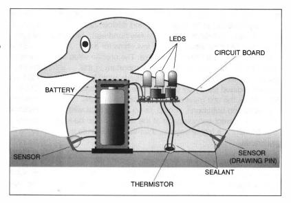
Figure 3: a suitable internal arrangement in a duck
