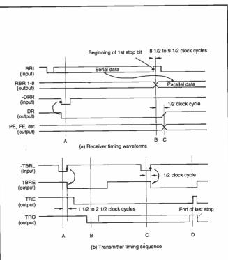
Figure 8: (a) receiver timing sequence and (b) transmitter timing sequence
