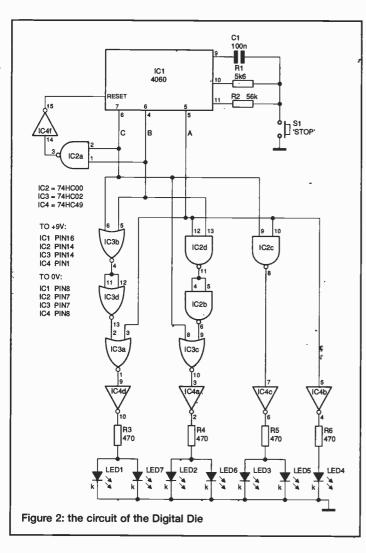
and 7 always come on together, so we can control these from a single buffer. The same applies to LEDs 2 and 6, and LEDs 3 and 5. LED 4 operates on its own. The table shows that LED 4 is to be on when digit A is low. This makes the logic very simple; the buffer for LED4 (4b) is connected directly to the A logic line.
