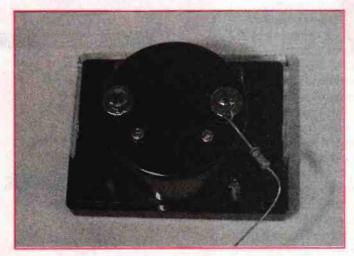
A single resistor, used to make the meter read in volts
