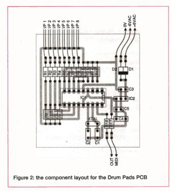
microcontroller which scans the inputs on RB0 to RB7. When a high is detected the software transmits the equivalent noteon ( and then the MIDI note-off after a short delay) for the required drum sound on the MIDI output on RA0.
