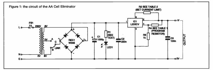
connected in series, that is, by connecting C to B as shown) or 6V (with the link connecting C to A instead - this uses only one secondary section). For equipment designed for two cells, the latter is used. For three or four cells, both secondaries will be needed. The mains earth wire is connected to the case and also runs through to the negative (OV) output terminal.
