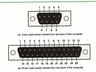
Pin functions of the RS232 connectors
