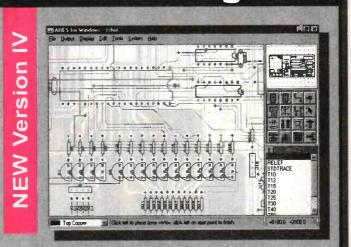
•Automatic Component Placement. •Rip-Up & Retry Autorouter with tidy pass. •Pinswap/Gateswap Optimizer & Backannotation. •32 bit high resolution database. •Full DRC and Connectivity Checking. •Shape based gridless power planes. •Gerber and DXF Import capability.
