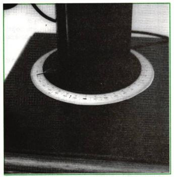
Detail of the stand showing the circular protractor and a hardboard pointer disc at the base
