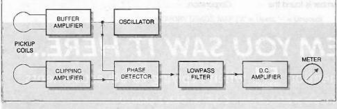
Figure 1: the block diagram of the cable detector
