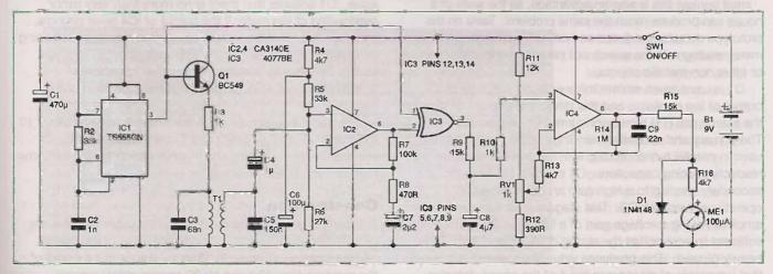
Figure 3: the full circuit diagram for the cable detector
