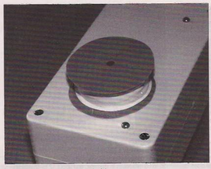
The search coil mounted on the back of the case.
