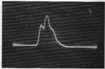
The trace produced by a 2.6 kHz ceramic filter and its matching transformers with the probe gain set high and probe used with the wobbulator. The comparisons suggested confirm the linearity of the probe when its gain is set high and also reveal the way in which the shape of the IF passband is largely determined by any filter elements.
