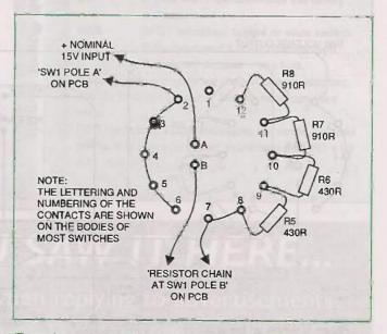
Figure 3: connecting the wires and resistors to SW1
