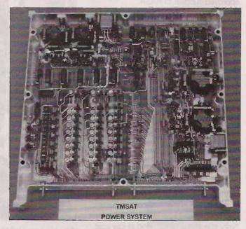
A typical single satellite module built into a chassis of standard dimensions:
