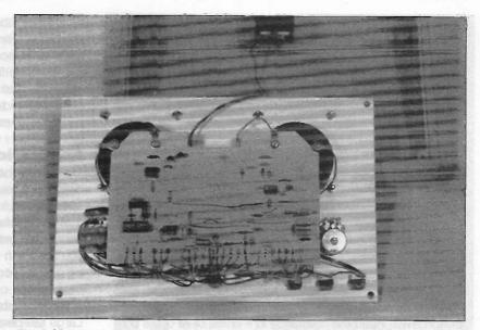
The PCB bolted down to the front panel meters and ready to be cased
