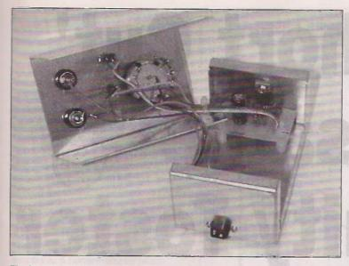
The board and offboard components mounted in an aluminium case
