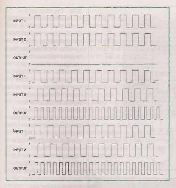
Figure 2: example waveforms for the phase detector
