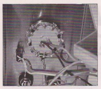
The resistors and wiring mounted on rotary SW1
