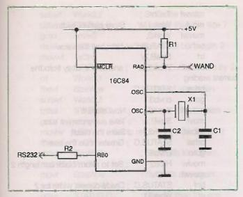
Figure 4: the circuit diagram of the interface
