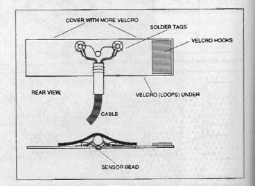
Figure 5b: construction of temperature probe
