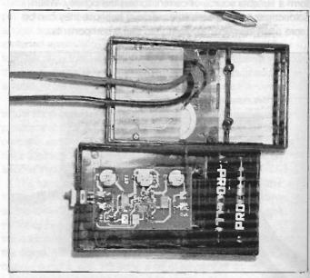
The continuity tester (left) and power supply (right) boards mounted into a case with batteries and a single on/off switch. If other types of batteries or power supply are used, chose a different case to suit
