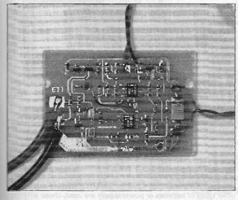
The surface mount board made up and with the wires installed
