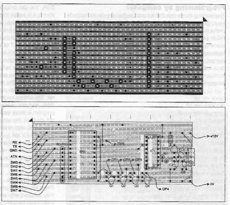
Figure 3: the component layout. This board replaces Boards 1 and 2 of last month's circuit. (Please note that C3 should go to 0V, not to pin 9 as in the photograph.)
