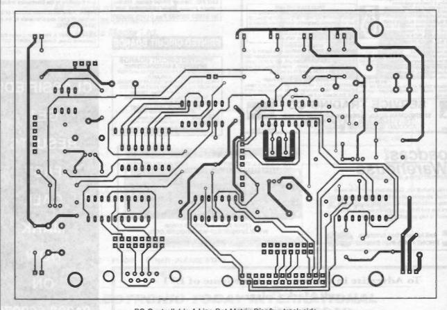
PC-Controllable 4-Line Dot Matrix Display: track side
