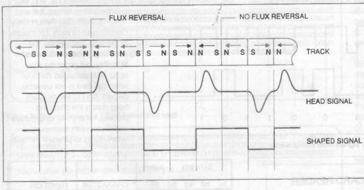
Figure 2: Reading a magnetic track
