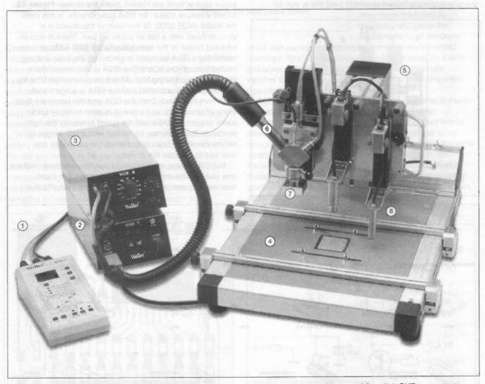
Figure 13: The Weller WQB 2000 BGA/QFP, an industrial solder reworking system for ball grid array and fine pitch SMT components. Difficult repair processes: desoldering, printing a new solder paste layer, component placement and resoldering are carried out on a preheated base table. Exact repositioning of the component is achieved with a vacuum pick-up nozzle that lifts and lowers the new component before and after the solder paste printing process.
