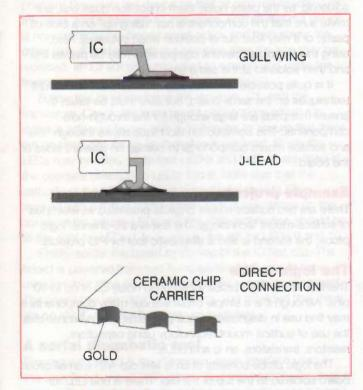
Figure 4: chip connections.
