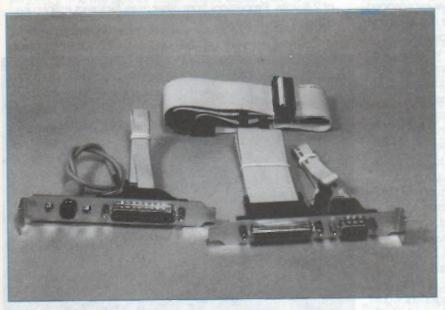
Modern motherboards have integrtaed parts of various types. Make sure th board is supplied complete with a basic set of matching cables
