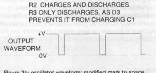
Figure 3b: oscillator waveform: modified mark to space
