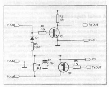
Figure 8: the diagnostic serial interface circuit
