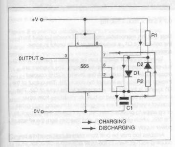
Figure 1: a pair of diodes are used with the 555 ic for obtaining mark:space ratios of 1 or less
