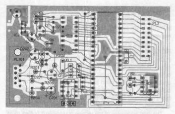
Figure 11: the pcb layout of the 16C74 development board
