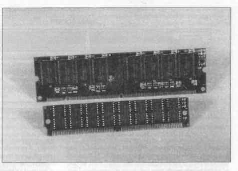
SDRAM in the form of 168-pin DIMMS (top) are now replacing 72-pin EDO SIMMs (bottom)
