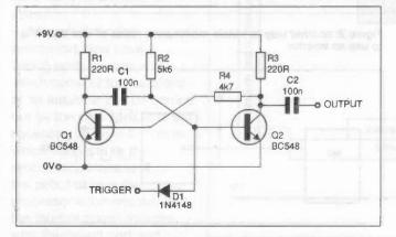
Figure 5: cross-connected transistor switches are used to build a monostable
