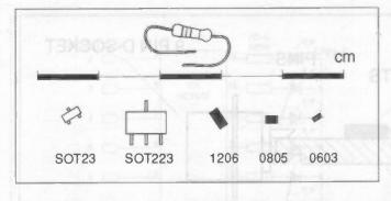
Figure 12: Life-size surface mount SOT23 and SOT223 transistors plus 1206, 0805 and 0603 resistor packages. The 0603s can be soldered by hand - but we don't recommend it for first timers
