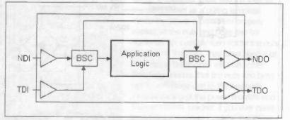
Figure 1: the principle of Boundary Scan
