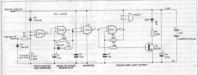
Figure 1: the circuit of the Aquaprobe. The probe sleeve and tip apply if a jack plug is used as the probe.
