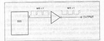
Figure 2: another way to obtain mark:space ratios of less than 1 is to use an inverter
