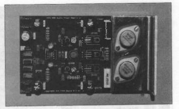
Photo 1: the 100W power amplifier built on a manufactured printed circuit board
