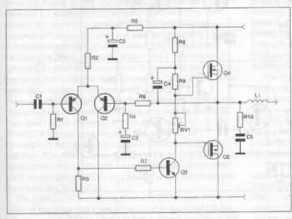
Figure 1: a simple discrete-component power amp
