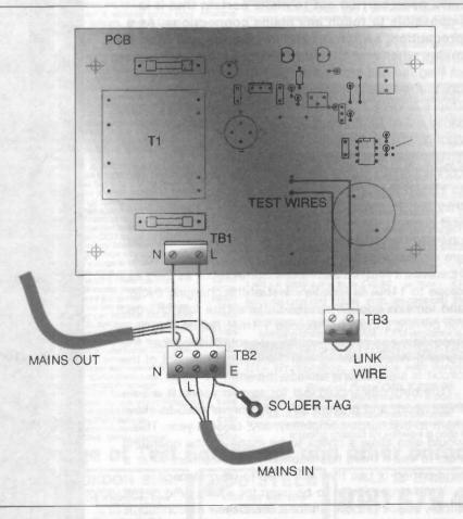
Figure 3: wiring connections to the mains
