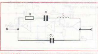
Figure 10: this network is the electrical equivalent of a piezoelectric crystal
