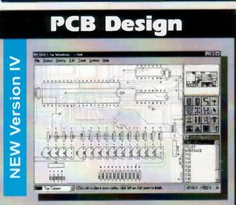
•Automatic Component Placement. •Rlp-Up & Retry Autorouter with tidy pass. •Pinswap/Gateswap Optimizer & Backannotation. •32 bit high resolution database. •Full DRC and Connectivity Checking. •Shape based gridless power planes. •Gerber and DXF Import capability.
