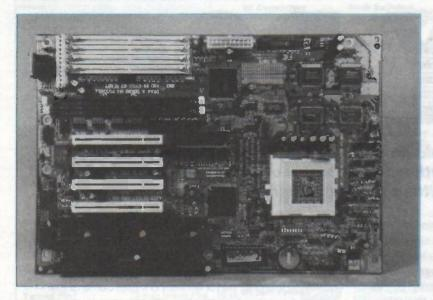
This gigabyte motherboard uses the standard AT layout. The large ZIF socket is for the CPU.
