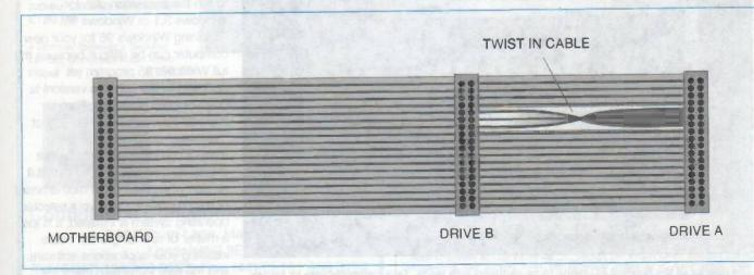
Figure 2: a twist in the data cables determines which floppy disk drive is A, and which is drive B.
