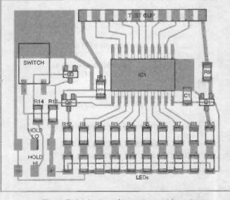
Figure 7: the logic probe component layout
