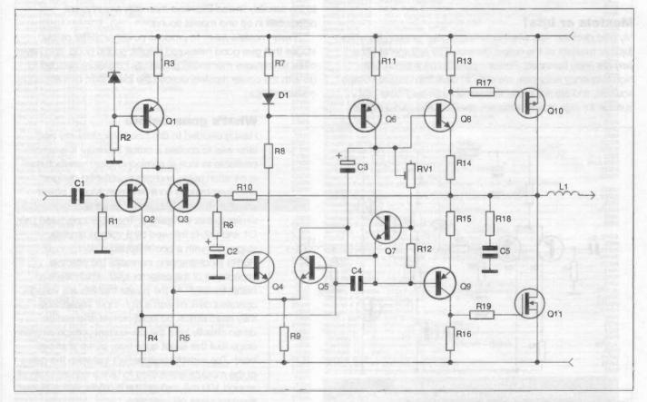
Figure 2: an improved discrete-component power amp
