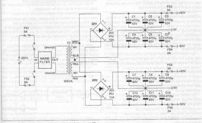
Figure 6b: a suitable power supply circuit for dual power amplifiers
