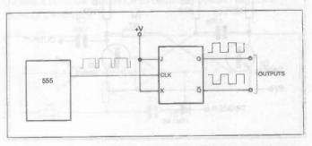
Figure 3: a flip flop converts a signal with any mark:space ratio to a signal at half the frequency and a ratio of exactly 1
