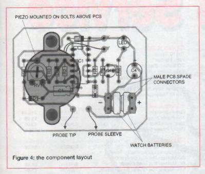
consume power and with two small hearing aid batteries we have a limit on the length of time this can be maintained. The solution is to pulsate the outputs; if a 1:1 mark to space output was used the outputs would be off for as long as they were on (in dry conditions only), effectively doubling the active output life. The trouble is that even this would not be enough, so a duty cycle of around 40:1 is used. This increases the output life approximately 40-fold.
