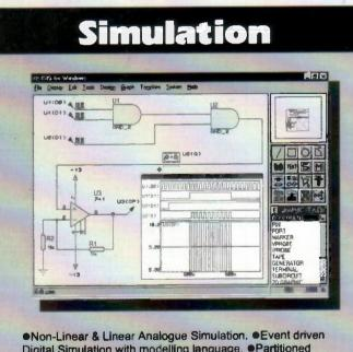
Non-Linear & Linear Analogue Simulation. Event driven Digital Simulation with modelling language. Partitioned simulation of large designs with multiple analogue & digital sections. Graphs displayed directly on the schematic.
