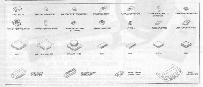
Figure 11: component types used with the Panasonic Panasert NM2544/2545 component placement machine
