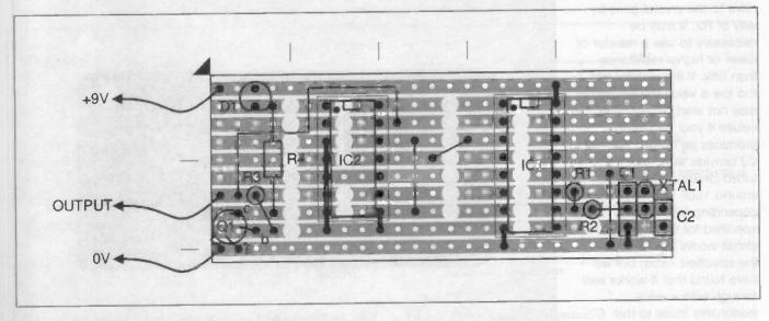
Figure 13: the stripboard layout of the clock module
