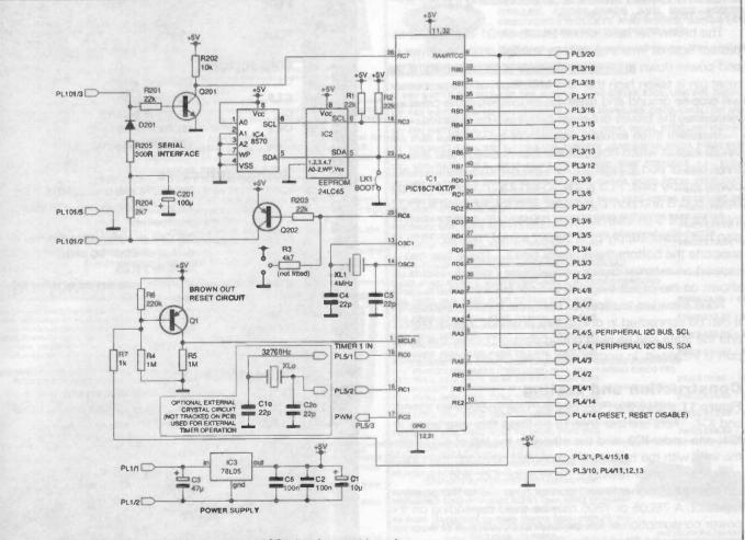
Figure 10: the circuit diagram of the 16C74 development board
