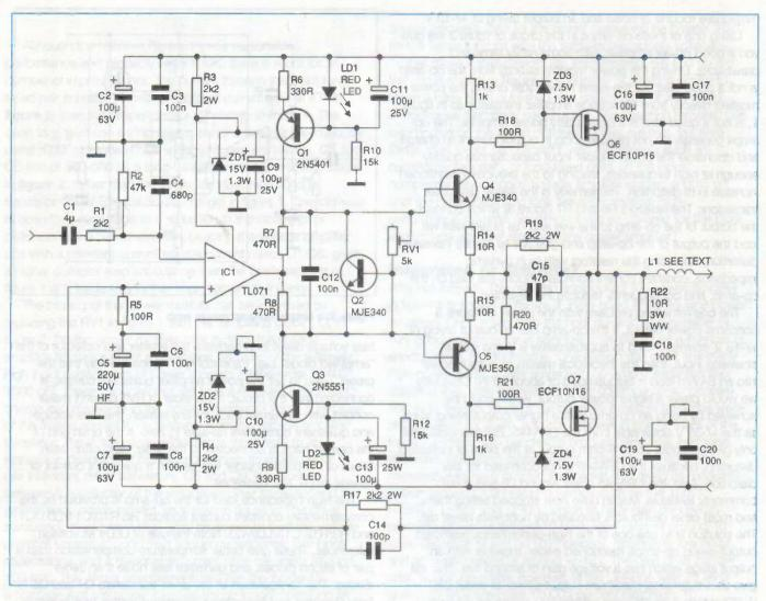
Figure 4: the final op-amp power amp circuit
