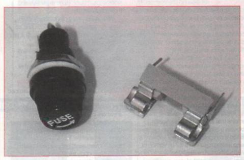
On the left is a panel fuseholder, mounted through a hole in the case and changeable without opening the case up. On the right is a pcb-mounted fuseholder.
