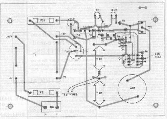
Figure 2: the component layout for the Mains Monitor
