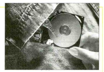
Another IBM 2.5 in disk drive with MRX head technology sets a new density record, storing the most data per square inch of any disk drive: 2.64 billion bits. The Travelstar 4GT is only half an inch (12.5 mm) thick and it destined for new ultraportable laptops. The 4GT is also designed to be the most rugged 2.5 in disk drive, based on its non-operational shock rating. (This is the measurement of how much force is applied to the drive before it no longer functions fully.)
