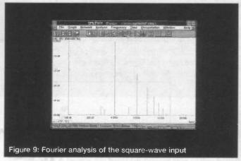
Further along, the 9kHz signal shows attenuation of -22dB. There are also signals at 2f, 4f, 6f etc. in the square wave, but of these only the 2f signal is above the -50dB level in the filtered signal. The output spectrum is dominated by the odd harmonics, which is typical of a triangular wave.
