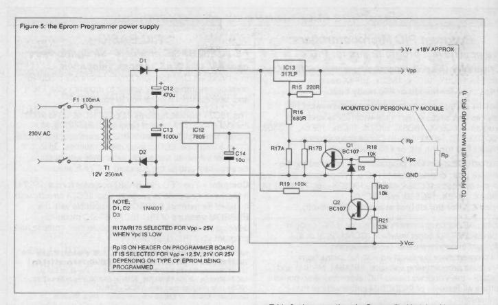
required for a particular eprom. Resistor values for the common programming voltages of +12.5, +21V and +25V are given in Table 2. Use 1 percent or 2 percent resistors.
