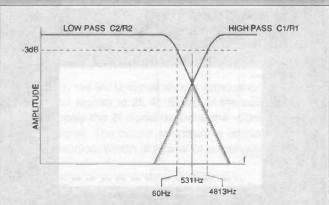
Figure 3: overlapping responses of the low-pass and high-pass sections of figure 1 produce a sharply peaked band-pass response
