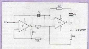
Figure 2: an alternative Wien oscillator that can be tuned by varying the value of R1
