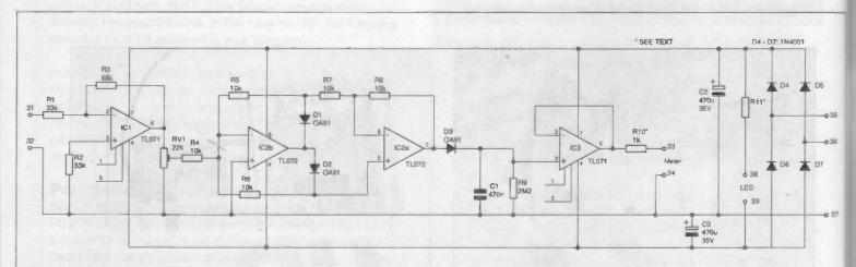
Figure 1: the circuit of the Peak Reading VU meter with power supply
