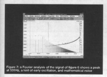
The Fourier analysis also displays the phase of the signals, using small square symbols. In figure 7 the phase of the 1kHz output signal is +9.81 degrees. Owing to the way the analysis is calculated, this is with respect to the input plus 90 degrees, so at 1kHz the output is 99.81 degrees ahead of the input, as already shown in figure 2.
