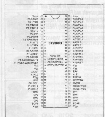
Figure 14: 8 x 930Hx USB hub/peripheral controller pin-out (64 pin package)
