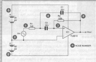
Figure 1: last month's Problem - the filter circuit
