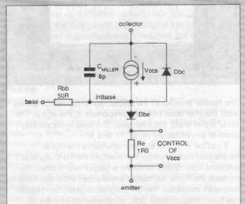
Figure 11: the 'npn' translator model is basic but quick-running
