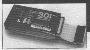
access time standard, with 35 ns optional; DOS-based PC software tools; compact size in a rigid case; power-off backup circuit and 28- and 32-pin dip eprom adapters included (with PLCC adapters as optional).
