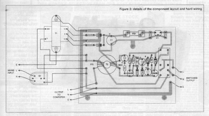
from the mains supply. T1 is the step-down and isolation transformer in the power supply unit, which is a conventional 12 volt stabilised design. D1 and D2 provide full-wave rectification, and C1 is the smoothing capacitor. IC1 is a small (100 milliamp) voltage regulator, which is more than adequate in this application where the
