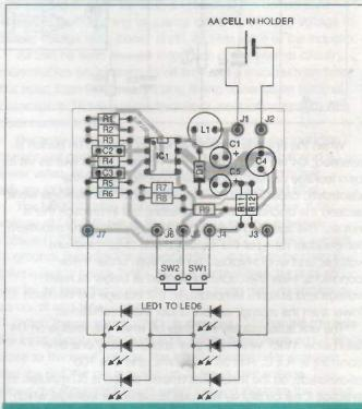
Figure 4: the component layout and offboard wiring
