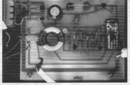
is turned on. The decay time is relatively long at around two or three seconds, which ensures that any minor glitches on the mains supply do not result in power to the peripheral units being completely switched off for short periods.
