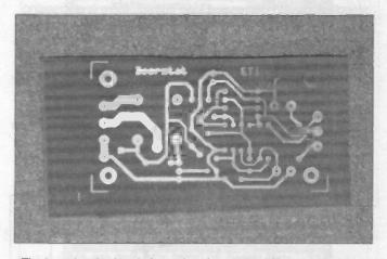
The board etched and cleaned and ready to drill. It may not be quite as "sharp" as an industrially-produced board, but the results are good nevertheless - and much cheaper.
