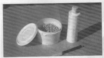
The P-n-P Stripper, marker and ferric chloride etchant. Press-n-Peel now supply colourless sodium persulphate/sodium bisulphate etchant.
