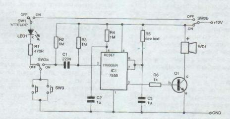
Figure 1: the circuit of the Caravan Movement Alarm
