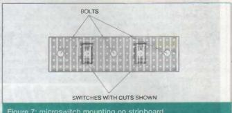
Figure 7: microswitch mounting on stripboard note the track cuts
