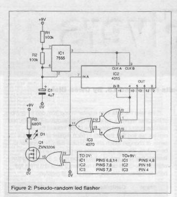
255 states and, clocking the register at 1Hz it takes over 4 minutes before the sequence repeats. It is almost impossible to distinguish between this repeating sequence and a non-repeating truly random one.
