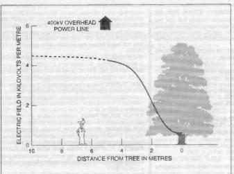
Figure 8: Reduction of electric fields by presence of trees
