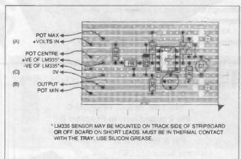
Figure 2: the Phantom Board. Note the 11 track cuts, including the one under R4
