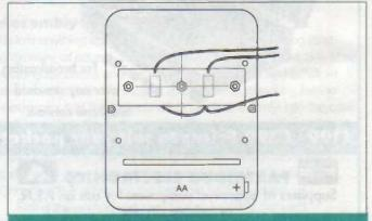
Figure 9: Inside of the the case lid, showing the approximate position of the Veroboard supporting the microswitches, the wiring to the switches, and the bolts securing the board to the case lid.
