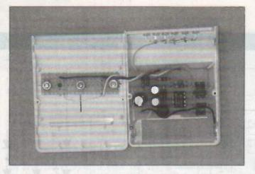
The interior of the Light, showing the Verostrip supporting the microswitches. (The battery compartment cover is shown removed).
