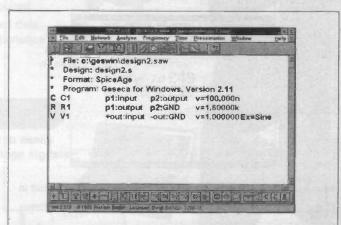
Figure 3: the netlist generated for the circuit by SpiceAge
