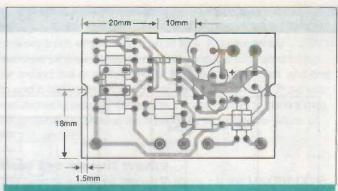
Figure 3: a guide to the cutouts to be filed in the pcb if using the case specified
