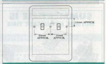
Figure 8: the top of the specified case, showing the position of the microswitches and 6nm bolts screws. See text. The Veroboard fitted inside the lid must clear the taller components on the PCB
