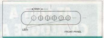
Figure 5: guide to drilling the LED holes - 3mm diameter - in the front panel
