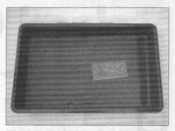
A single board in the P-n-P etching tray.
