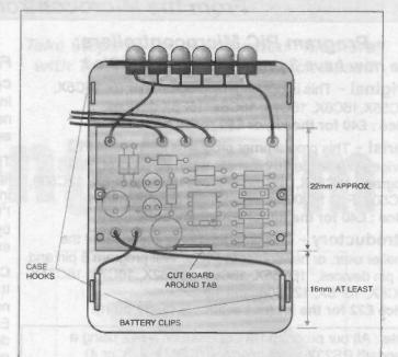
Figure 10: the layout of the PCB, LEDs and wiring inside the case. The battery clips have small loops to solder the wires to. The tab at the edge of the battery compartment separates the PCB from the compartment, and helps to retain it in place. See text.
