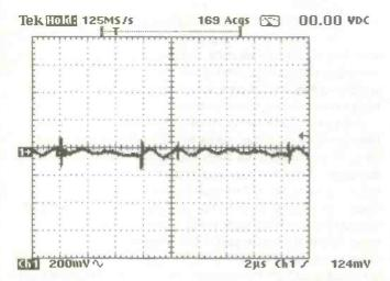
Figure 7: interference on the input terminals
