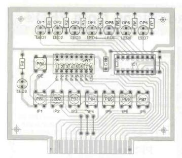
Figure 4: the component layout for the software test board
