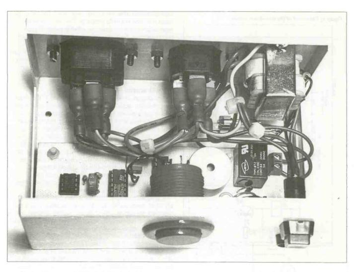
12 will also be low. The output of IC3c - pin 10 - will then be high (shown by line 2). If IC3a output is high, pin 10 will be low (shown by line 8). The pulses obtained from IC3c pin 10 then operate buzzer, BUZ1. At the lower clock speed there will be a rapid bleeping. At the higher one the pulsing will be so fast that the buzzer will produce a warbling tone.
