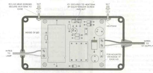
Figure 15: layout of the pcb in the lid, and assembly into the box. Note that the pcb lies upside-down in the box. Either tubular or flat grommets are suitable, so long as they protect the wires from fraying
