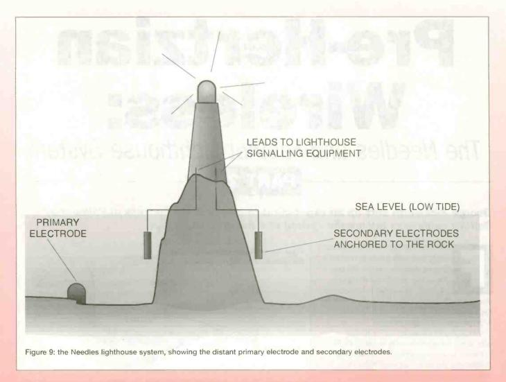
where it came ashore. Poor visibility frequently prevented signalling with lamps or flags, often at those times when communication was most urgent, so, in 1892, the Needles system was adopted. According to Fahie, the shore end of the cable came ashore near Galley Cove, a few miles from Crookhaven Post Office, while the distant end terminated at a 500-pound mushroom-shaped copper electrode lying under 11 fathoms of water 100 feet from the rock.
