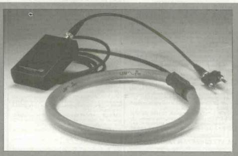
durability. Standard models are available in lengths of 61, 91 and 122 cm, with dual ranges of 0-30/30-300A, 0-300/\$CC-3000A and 0-60/600-6000A. Flexible air-core toroidal current transformers have overcome the limitations of iron-core current transformers, particularly with regard to rigidity.
