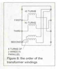
direction as the other two windings. Then solder the wires to the pins, making sure that the solder contacts the wire through the self-fluxing insulation. A hotter-than-normal soldering iron temperature is desirable for this process. In
