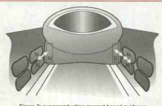
Figure 2: superconducting magnet based guidence
