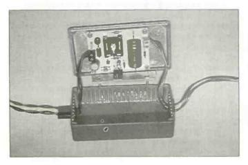
a voltage-boosted flyback converter configuration.
