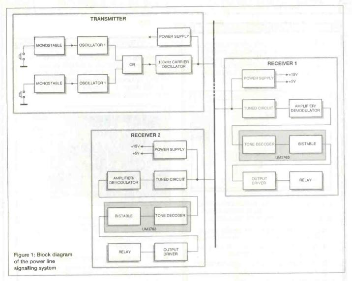
The best frequencies to use seem to be between about 80 and 150kHz and this system runs at approximately 100kHz. The normal domestic supply consists of three wires: Line (or Live), Neutral and Earth. In theory, the signals could be sent between any two of these.
