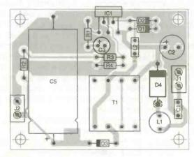
Figure 11: the component overlay
