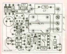
Figure 3: The receiver PCB and component Jayout
