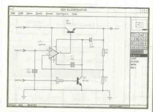
The schematic drawing module of CADPAK, ISIS Illustrator, enables you to create circuit diagrams like the ones in the magazines.
