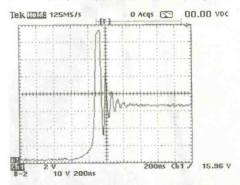
Figure 4: the switching waveform expanded to show a switching spike
