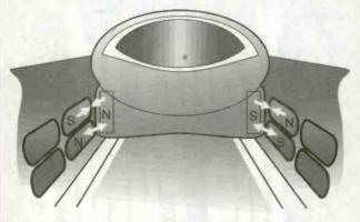
Figure 3: superconducting magnet based propulsion
