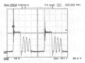
Figure 5: the switching waveform on IC1 pin 4 but without the ferrite bead
