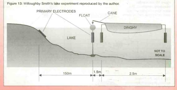
obtained when the secondary circuit was energised and the meter connected to the lake-side end of the primary circuit; this demonstrated that the system could be used for two way communication.
