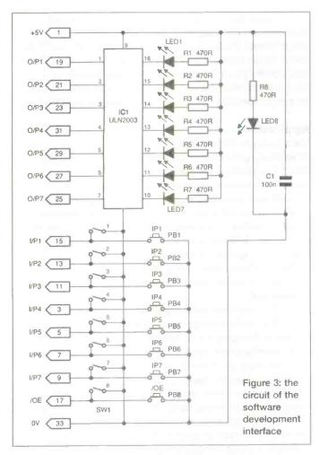
you must place the jumper link JP1 on the main controller in the EXT (right hand) position. With the switch closed or pressed the LED indicators are enabled. When the switch is open or released the LEDs are disabled.
