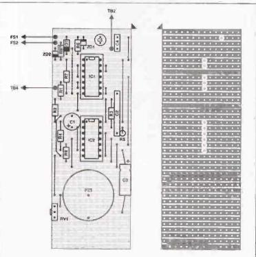
Component layout on stripboard and track cutting positions
