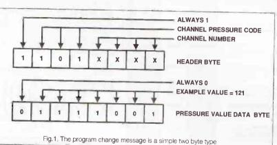
of message very rapidly, making it possible to use program changes midsequence. This is a form of channel message and it is therefore possible to individually change the sound of each voice of an instrument operating in mode 4 or a multi-mode. This may still
