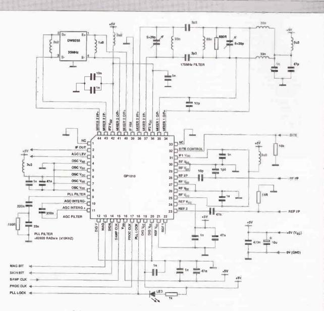
Basic circut for the heart of a GPS receiver based on the GEC Plessey GP1010
