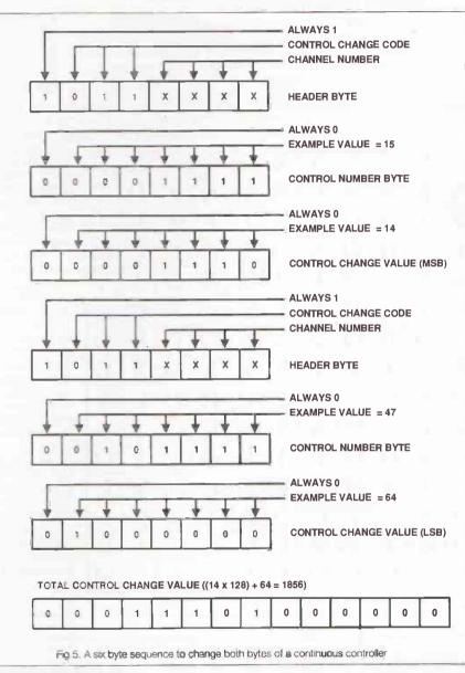
bytes. Control 0 is paired with control 32. control 1 is paired with control 33, and so on through to control 31 which is paired with control 63. This works in a manner that is similar to the way in which the pitch wheel message provides 14 bit resolution. However, the pitch wheel change message carries the two 7 bit bytes in one message, whereas they are in separate messages for a control change.
