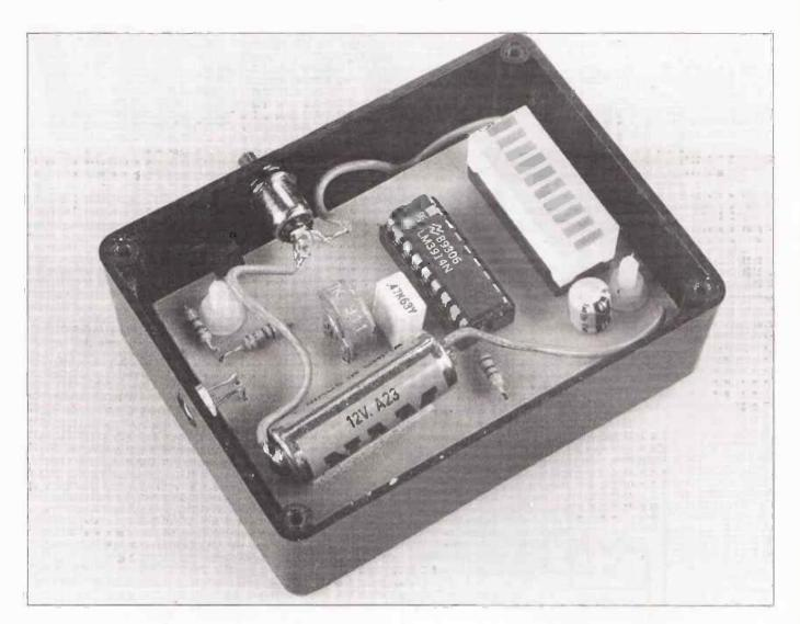
voltage provided by Q1 collector needs to be divided by four. This is achieved when VR1 wiper is at approximately midtrack position. However, the voltage at the wiper may be adjusted through wide limits. This provides the adjustment for the correct operating levels and will be made at the end of construction. Capacitor C1 promotes stable operation.
