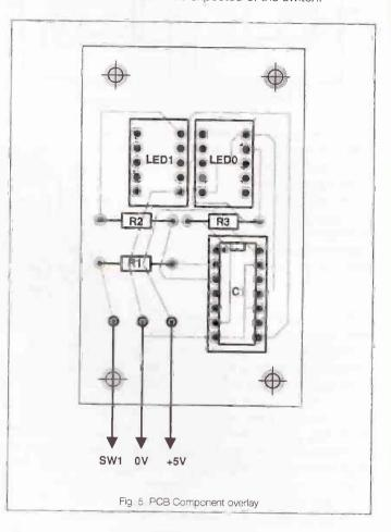
None of the components are difficult to obtain. Only the 7-segment displays are important in that they are low current, high brightness types.
