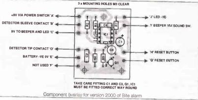
contacts close, switching 9V to R4. R4 and R5 produce a voltage divider and current limiter, essential to the safe operation of the thyristor.
