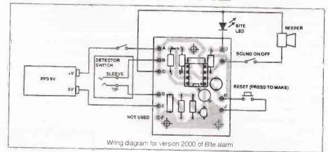
distinct parts, both of which use components commonly found in school projects - the latch, built around a thyristor and the oscillator, built around the 555 timer.
