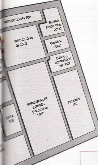
predictions. If the BTB prediction is wrong, then the pipeline is flushed and the correct instruction fetched, thereby causing a 3 clock cycle delay.
