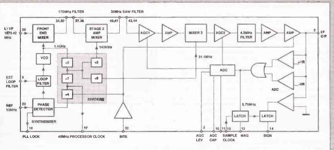
Block diagram of a GP1010 GPS chip
