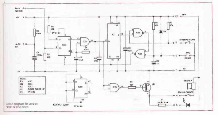
to drive the output transistor Q1 to power the LED and beeper. A transistor is required to amplify the current output of the CMOS IC which can only supply 1mA or so directly.
