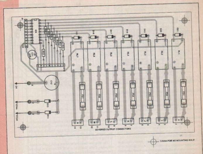
Fig.4 Component overlay for Relay board
