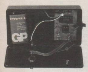
resistance mode (i.e. R3 selected), the audio alarm should be activated if a 4R7 resistor is connected across the prods. However, changing to a 22R resistor should not give a response from the unit. With the tester set to the low resistance mode (i.e. R2 selected), connecting the 4R7 or 22R test resistors across the test prods should fail to activate the audio tone generator. Using a 0R47
