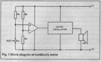
resistance across the test prods in order to activate the unit. The resistance here merely has to be low enough to take the potential at the non-inverting input below that at the inverting input. Just what constitutes a low enough resistance to achieve this depends on the values of R1 to R3.
