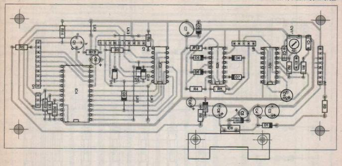
Fig.3 Component overlay for Main control board
