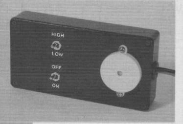
here are two common problems with continuity tester designs. One is simply that many testers indicate continuity when there is actually a significant resistance across the test prods. What is supposedly continuity can sometimes be resistances of up to a few hundred ohms. Also, many designs are 'fooled' by diode junctions. Such junctions are not just present in diodes, but also exist in transistors and integrated circuits. In fact modern circuits are liberally scattered with hidden semi-
