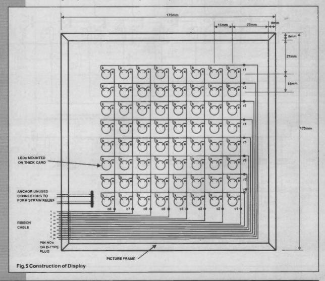
When the circuit has been tested and found to be correctly working, the back of the 'picture' can be coated in silicon rubber (the clear type used to seal sinks, windows, etc. works well). This will help to hold all the LEDs in place and will also stop accidental shorts.
