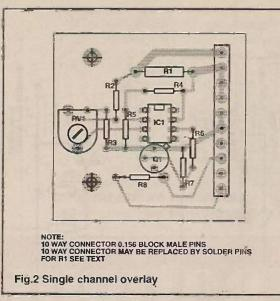
and, once the Lumitec has been fitted and the wiring checked, the RV is adjusted so that the buzzer sounds when the appropriate bulb is removed and the circuit powered.
