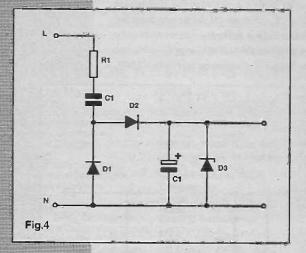
and, in order to calculate the average direct current available it is necessary to average the current in R1 over a whole mains cycle, even though the current is only flowing during positive halfcycles.
