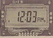
**Z5557** Clock module with timer and two alarms. Displays day, hour, min and AM/PM. Overall size 48x32x7mm; display 10mm.
