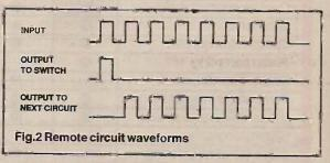
The last remote circuit of the chain is terminated by a fesistor, which acts as a permanently closed dummy switch. The corresponding LED is a green one which lights to indicate the closed condition. This is used to show that the monitor is operating when all the windows are closed and the red LEDs are therefore off, as well as to provide a continuity check for the chain.
