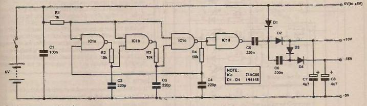
Fig.4 Battery powered supply
