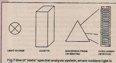
diffracted using a static diffraction grating and the output is detected by a stationary linear diode array
