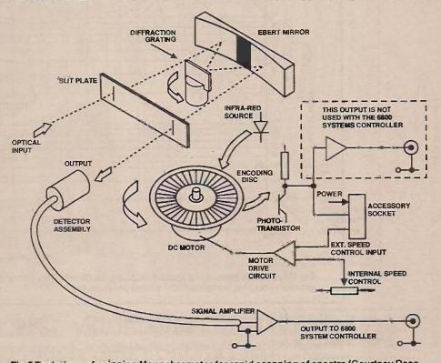
Fig.5 Technique of spinning Monochromator for rapid scanning of spectra (Courtesy Rees Instruments Ltd)
