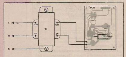
Fig.3 Transformer wiring diagram
