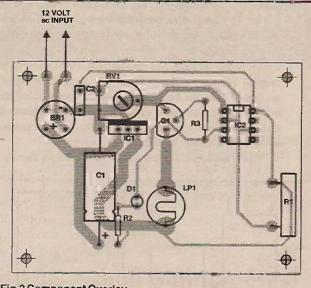
Fig.2 Component Overlay
