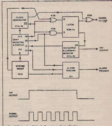
Fig.13 Main circuit block diagram and waveforms
