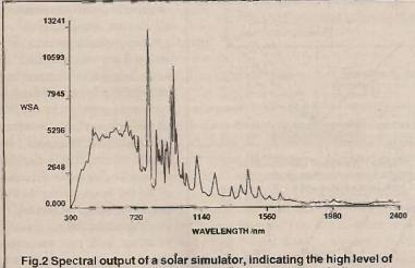
Fig.2 Spectral output of a solar simulator, indicating the high level o complexity of the spectrum (Courtesy Rees Instruments Ltd)
