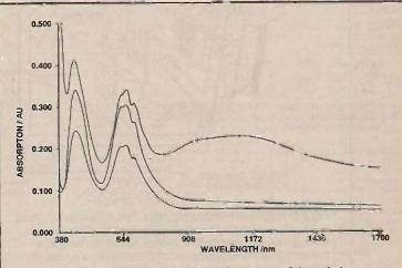
Fig.1 Values of absorption properties of samples of doped glass (Courtesy Rees Instruments Ltd)
