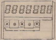
Z2658 LED module. An interesting little PCB 50x35mm that has mounted on It a 7 digit 7 segment red display, and a plastic mouiding under which are 3 surface mount LED's, one each red, yellow and green. On the back of the PCB is a SED5031M chip. Offered without info at present, although we are working on It. Ballayed to have been the display on a are working on it. Believed to have been the display on a mobile phone. Only  $\mathfrak{L}1$  each
