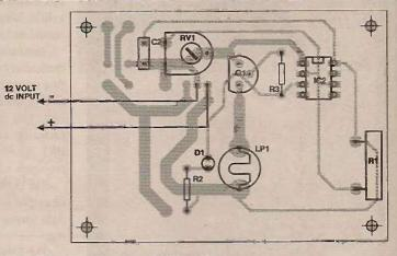
Fig.4 Component overlay of 12V version
