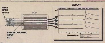
Fig.8 Use of a CCD to record four simultaneous spectra: in this example each spectrum is mapped to a specific region of the CCD surface
