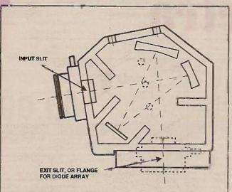
Fig.3 Principle of Monochromator. The diffraction grating is usually rotated by hand and the light output emerges through an output slit. The device shown is, in fact, a Spectrograph manufactured by Oriel where a complete spectrum can be passed to a long narrow exit slit (Spectrograph mode) or a single range of wavelengths can be selected (Monochromator mode).
