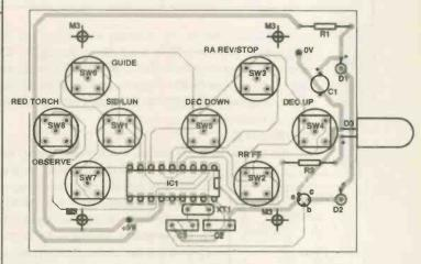
Fig.2 Component overlay of transmitter
