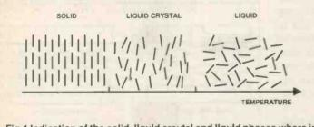
Fig.1 Indication of the solid, liquid crsytal and liquid phases where in the solid phase molecules are fixed relative to each other with high level of organisation, in the liquid crystal phase molecules are more loosely associated but still have some collective structure and in the liquid phase the molecules are free to wander around the liquid with no level of order between the molecules.
