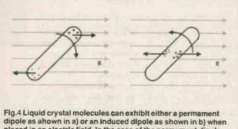
dipole as ahown in a) or an induced dipole as shown in b) when placed in an electric field. In the case of the permament dipole the molecule will tend to be aligned in the direction parallel to the field and in the case of the induced dipole at right angles to the field.
