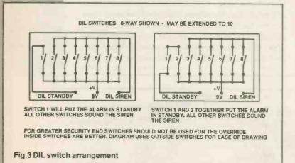
mode i.e. not functioning and this is done by setting the code on the DIL switch and leaving it set. When you need to use the alarm, the de-activate switch/switches are turned off. This enables the alarm after a time out period of several seconds - ample time to position it in a bag or locker (not forgetting to shut the bag and lock the locker to exclude light). is de-activated. Releasing the de-activate switches will activate the alarm all over again and the same sequence is initiated.
