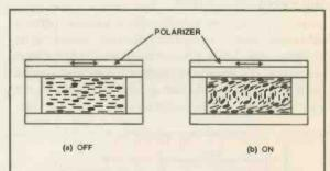
Fig.11 Utillsation of the 'guest-host' liquid crystal which includes a dichrotic dye which lines up with the liquid crystal molecules. The dye molecules are strongly absorbing of specific wavelengths of light when in a) the OFF state and the display appears brightly coloured. When the electric field is applied this property is lost as the molecules tend to align parallel to the electric field direction and the bright colour is lost.
