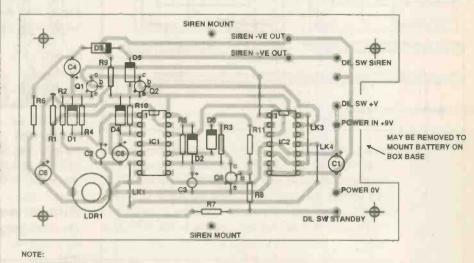
4 X CORNER FIXINGS M3 CLEAR SIREN MOUNT VIA LONG BOLTS TO HOLD SIREN CLEAR OF COMPONENTS - M3 CLEAR MOUNT LOR TO POINT TO MAXIMUM LIGHT INPUT
