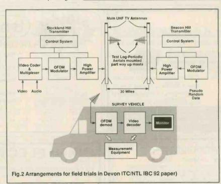
Frequency Division Multiplexing), the resulting signals can be inserted at low power into the existing gaps in the spectrum, so that they do not interfere with their neighbouring high-powered analogue TV signals and yet they are rugged enough for a digital receiver to be able to decode them into perfect pictures and sound.
