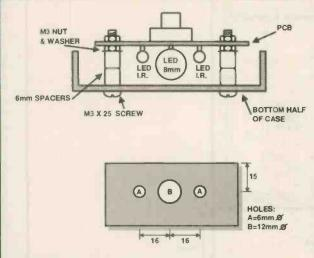
Fig.6 LED arrangement within handset (front view)
