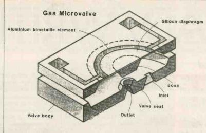
film deposited on the diaphragm forms the other element of the bimetallic structure. Varying the electrical power dissipated by resistors implanted in the diaphragm makes the temperature of the diaphragm change. As temperature increases, the difference in thermal expansion between the silicon and aluminium forces the boss away from the valve seat. The higher the temperature, the farther the valve opens.
