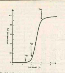
Fig.7 Details of the switching characteristics of a typical LCD display element. This curve determines the relative contrast of the display.
