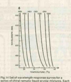
series of chiral nematic liquid crystal mixtures. Each set is designed to respond within a range of 2 degrees C.
