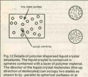
right angles to spherical surfaces or at right angles to spherical surfaces. When the director of the liquid crystal lines up with an applied field, the light which falls directly interacts primarily with these liquid crystals.
