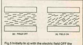
molecules align parallel with the electric held OFF the molecules align parallel with the glass plates. When the field is switched ON at a sufficiently high value the orientation of the molecules changes to try to align with the field.
