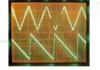
sweep timebase, which can be used to magnify a portion of a waveform, making possible, accurate time interval measurements and the study of short duration events. The sophisticated Type 7045, has a bandwidth of 40MHz and incorporates a 40ns delay line to enable the display of very short duration events in their entirety. Top-of-the-range is the Type 7046, a delayed sweep oscilloscope with increased magnification along with a 40MHz bandwidth and capable of displaying complex signals
