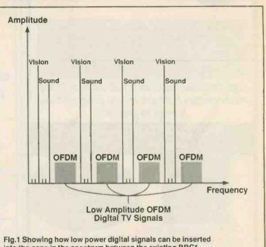
into the gaps in the spectrum between the existing BBC1, BBC2, Channel 3, and Channel 4 transmissions.
