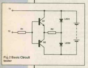
However, if one of the transistors is turned on its emitter-collector voltage is only about 0.1 volt. This would reduce the voltage across the LED with which it is in parallel to 0.1 also. As an example suppose Q1 is turned on then we have a circuit from the positive terminal of the battery, through Q1, R2 and LED2 to the negative terminal of the battery.
