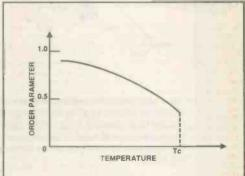
Fig.2 With increasing temperature within the liquid crystal phase the degree of orderliness decreases until it vanishes at the transition temperature to the liquid phase.
