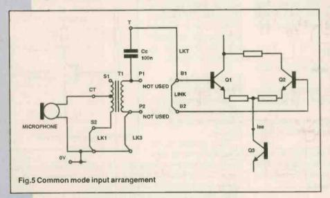
The circuit of the microphone amplifier employs a constant current source based around Q3, see Figure 6. This maintains the total emitter current (and thereby collector current) constant and will not allow common mode signals to increase this current. Because of this reluctance to change, current sources have a very high impedance. Replace Rt with a current source and wave goodbye to common-mode nasties!
