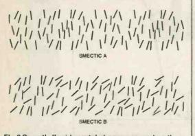
Fig.3 Smectic liquid crsytal phases occur when the liquid crsytals order themselves into layered structures as shown. Phases A and C are shown although up to eleven phases have been identified.
