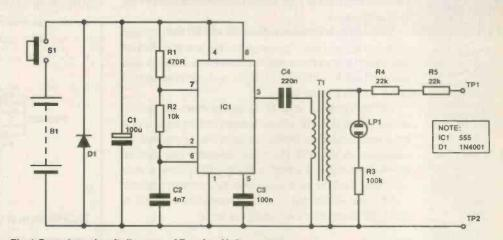
Fig.1 Complete circuit diagram of Proving Unit
