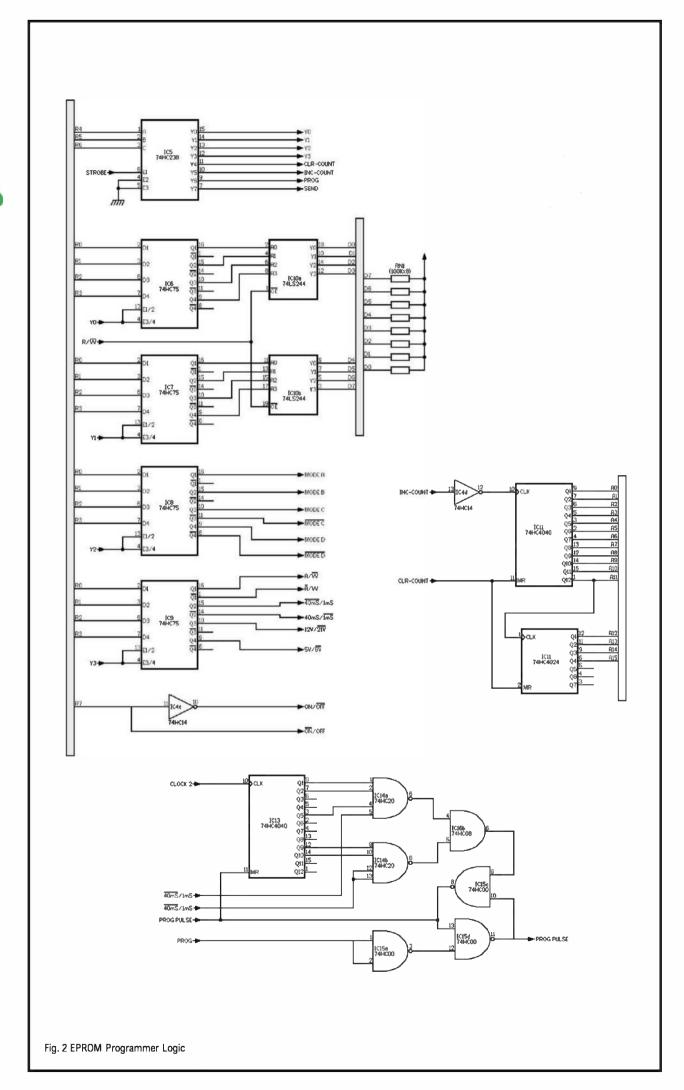
IC1 is the serial line driver/receiver, which converts RS232 standard serial signals to from standard 5V TTL levels. This IC contains voltage converters to produce the required transmission voltages (9V) from a single +5V supply.
