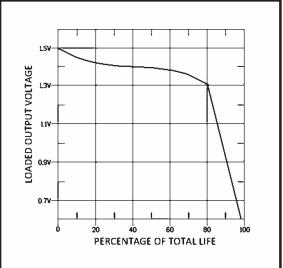
Fig.19 Chart showing how the output voltage of a lightly loaded 1.5 volt zinc carbon cell varies over its working life.
