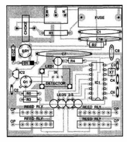
Fig.3 Component Overlay of receiver.
