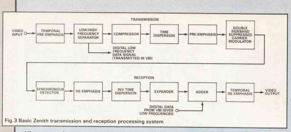
different types of processing it is possible to generate a signal for transmission with an even spread of energy over the spectrum, and a much lower average level of spectral energy.
