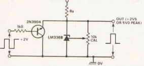
Fig. 16. LM336B-2.5 or -5.0 square wave calibrator circuit.
