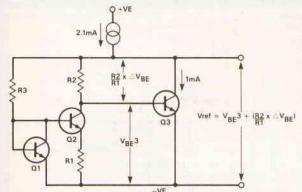
Fig. 8. Simple band-gap voltage-reference circuit.
