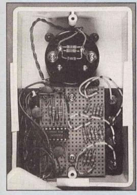
If all is well so far, the meter may be fitted and held in place with the 2.5 mm nuts and washers supplied.
