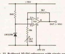
Fig. 11. Buffered 10.0V reference with single-ended supply.
