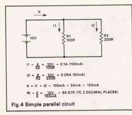
to calculate the total resistance, however. Figure 6 shows how Ohm's Law and Kirchoff's First Law can be used to develop a formula for calculating parallel resistance. This formula can be employed to calculate the total resistance of any number of parallel resistors. A useful point to remember is that if several resistors of the same value are connected in parallel, the total resistance is equal to the value of one resistor divided
