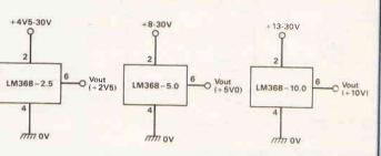
Fig. 17. Basic LM368 voltage-reference application circuits.
