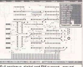
Full analogue, digital and SM support - ground and power planes - 45 degree, arced and any angle tracks with full net-based Design Rule
