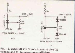
voltage and (b) temperature coefficient compensation.
