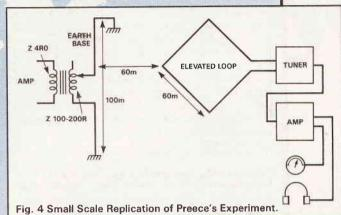
an earth loop will similarly respond to the changing magnetic field component of an electromagnetic wave, as is the case with a ferrite rod antenna.
