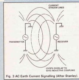
of the system, demonstrated in 1838 that a current does not take a direct route between two distant earth rods but that the stream lines spread out in a pattern similar to the lines of force of a bar magnet to form an infinite number of loops on each side of an imaginary line, connecting the two earth rods. The earth base of the distant receiver, aligned along a stream line provides an alternative path and thus intercept some of the current (Figure 2).
