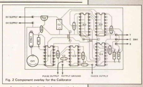
As mentioned earlier if a reference with a better accuracy than the crystal is available this should be used to set the crystal frequency using CV1. If this is not available the CV1 should be set to mid position with the vanes half meshed. The unit is now ready to be used to calibrate that receiver.
