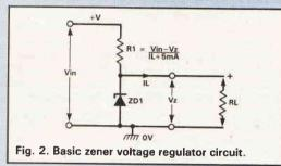
accuracy versions can be built by combining a zener diode with an op-amp and a constant-current generator. Alternatively, generators with very high accuracy and excellent long-term stability can be built by using a dedicated voltage-reference generator IC. This article looks at the various options, and shows practical versions of each type of circuit.
