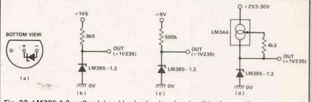
Fig. 23. LM385-1.2 outline (a) and basic circuits showing (b) reference from 1.5 V battery, (c) micropower reference from 9 V battery, and (d) reference from wide range supply.
