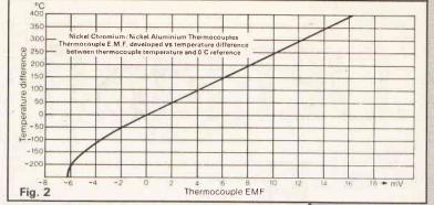
Figure 2 shows the typical response of a thermocouple. As can be seen, the output signal over the normal range of operation is 40V per °C. While measurable, this signal is too low for most electronic applications, so the first task is to amplify it. The circuit shown in Figure 3 incorporates on its input an amplifier which raises the signal level to approximately 2mV per °C.
