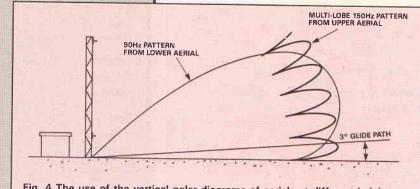
Fig. 4 The use of the vertical polar diagrams of aerials at different heights to achieve a straight line glide slope.
