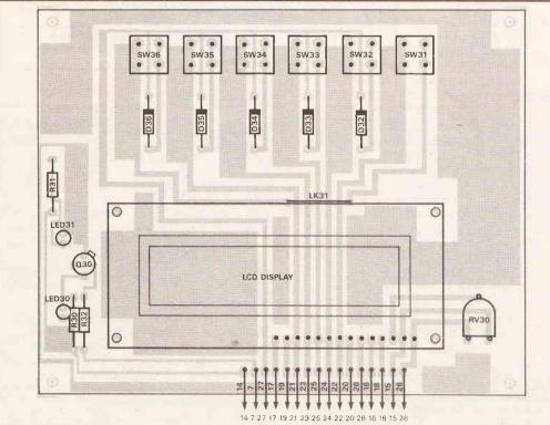
Fig.14 Display PCB Layout
