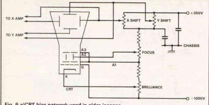
Fig. 6 a)CRT bias network used in older 'scopes
