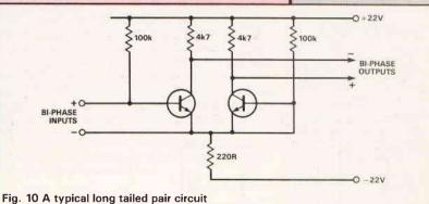
rig. To A typical long tailed pair circuit
