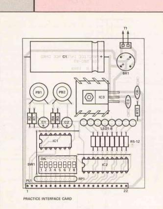
Fig.4 Component overlay for Practice Interface Card
