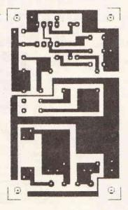
Remote Control Timeswitch Transmitter Board
