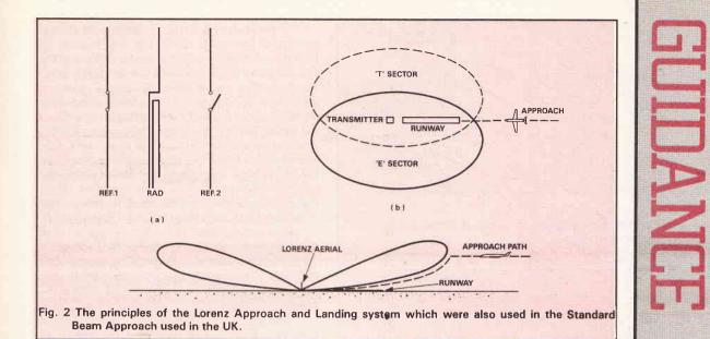
The aerial system was mounted at the downwind end of the landing ground at a height such that a single vertical lobe was radiated. The aircraft was equipped with a sensitive signal strength meter. Distance indication was given by two marker beacons, operating on 38MHz and located approximately 1000ft and 2 miles from the aerodrome boundary.
