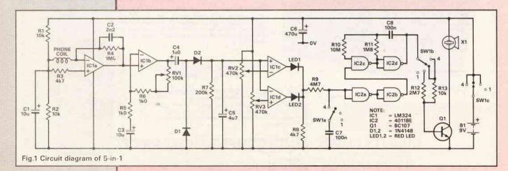
output as described earlier and adjust preset RV1 for a moderate hum. Turn RV2 and 3 so their associated LEDs are just off. Insert two tapes, press Play on either tape deck and LED1 should light. Set both decks to Play, re-adjust RV2 and 3 and stop one deck. LED2 should now light, and in both cases the alarm will sound.
