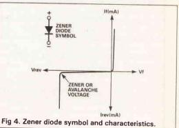
suddenly starts to increase. Any further increase in  $V_r$  causes a sharp rise in  $I_r$ , as shown in Figure 4. The voltage at which this action occurs is known as the avalanche or *zener* value of the device, and is sharply defined. Some silicon diodes are specially manufactured to exploit the zener effect, and can be used
