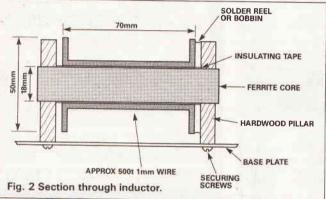
ince the original trials described in ETI over the last three months, further experiments have been carried out with a tuned, or *syntonized*, earth current receiver. This can best be described as a tuned radio frequency (TRF) receiver with a tuning coil and capacitor designed for very low frequencies. The only difference from a TRF receiver is that it does not rectify, but selectively amplifies the input signals.
