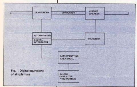
Brian Kendal shows there is more to fuses than meets the eye he fuse is probably the least understood component in common use today. Furthermore, the popular belief that it is merely a piece of wire which melts when the current passing exceeds the quoted rating is not only inaccurate but, under certain circumstances, a danger to the equipment which it is supposed to be protecting.
