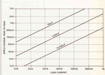
Fig 18. Filter capacitor selection chart, relating capacitor size to ripple voltage and load current in a full-wave rectified 50-60Hz powered circuit.
