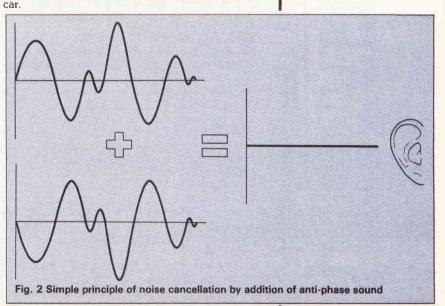
Fig. 2 provides a simplified illustration of how Adaptive Noise Cancellation works. Sound is a series of pressure waves which the ear can detect and the brain can interpret. If two sources of sound are in antiphase, the high-pressure peaks from one source coincide with the low-pressure troughs from the other, and vice versa. The peaks cancel out the troughs, and no sound is detected by the ear.
