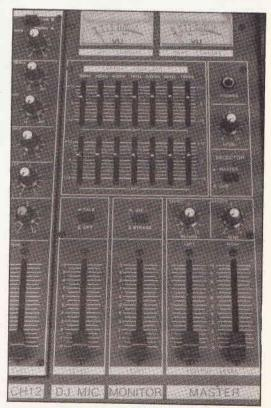
Just above the principal channel fader, an overload LED gives a handy and quick indication of overdrive to the input amplifier. The LED cuts in at around +4dB.
