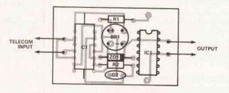
Fig. 9 Extension Bell Component Overlay
