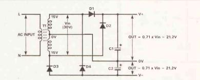
Fig 16. Dual (split) PSU using centre-tapped transformer and four rectifiers.
