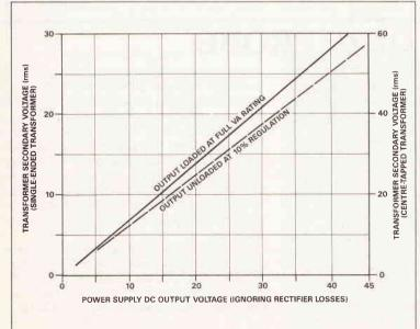
Fig 17. Transformer selection chart. Decide on the required loaded DC output voltage (say 21 volts), then read across to find the corresponding secondary voltage (15V single-ended or 30V centre-tapped).
