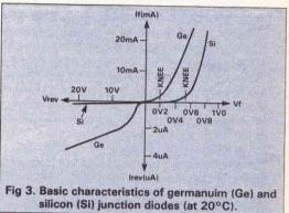
3. When a diode is reverse biased by more than one volt or so it passes a reverse leakage current  $(I_r)$  that is almost directly proportional to the reverse voltage  $(V_r)$  value. At normal room temperatures  $I_r$  values are measured in microamps in germanium devices and in nanoamps in silicon devices.  $I_r$  is highly temperature dependent, and typically doubles for each 8°C increase in junction temperature.
