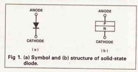
n junction. The *p* terminal is known as the *anode* and the *n* terminal as the *cathode*.
