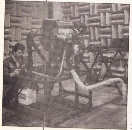
Reflected noise is removed by absorption at the walls and ceiling by the used of long, glass-fibre wedges. The depth of the wedges determines the lowest frequency level for which the absorbtion effect is valid — this is known as the cut-off frequency. Below this frequency, some reflection will occur, but at a dimished level.
