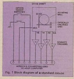
The ball mechanism of the mouse is subject to the ingress of dirt as well as wear and tear. Indeed, it has been known for the ball to become mysteriously detached and lost! In addition the proliferation of paperwork associated with computer use often doesn't leave the mouse enough room to move about.
