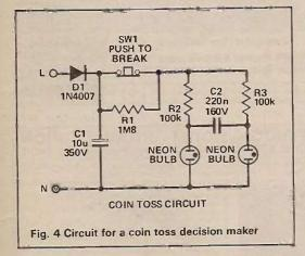
the main active components (Fig. 5). Suppose the lefthand neon of Fig. 4 is on and the right one isn't. C2 will charge via R3 until it eventually reaches the point where the right hand neon will strike. If we stick to the 80V and 50V I mentioned earlier as fairly typical for striking and extinguishing a neon, then just at the
