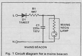
The circuit is shown in Fig. 1. On positive halfcycles of the mains, C1 charges up via D1 and R1. Eventually the voltage across C1 will be high enough for the neon to strike and glow. The current taken by the neon discharges C1 until the voltage is too low for the neon to continue glowing. It turns off, C1 begins to charge and the cycle repeats for ever more.
