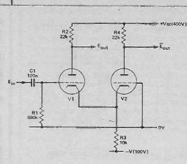
Fig. 15 'Long tailed pair' inverter stage
