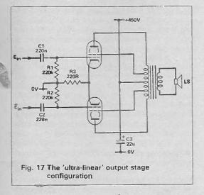
and this demands a very good output transformer — since this is the component which introduces the bulk of the end of passband phase shifts.
