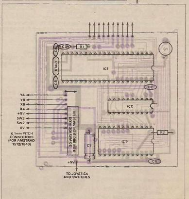
Fig. 4 Component overlay for the mouse-on-a-stick
