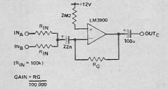
Fig. 4 Signal mixer using LM3900 Norton op-amp
