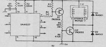
Fig. 8 Two circuits to boost the drive current (a) using independent phase windings and (b) coupled phase windings
