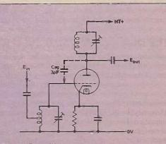
Fig. 4 HF amplifying stage
