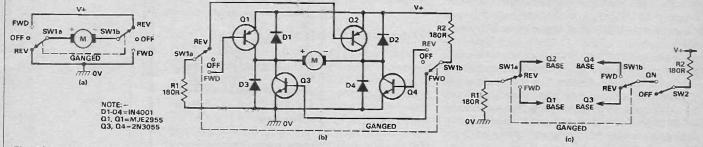
Fig. 12 Motor direction control with single-ended supply (a) simple switching (b) transistor switching (c) separate on/off switching
