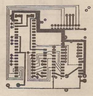
The digital joystick-to-mouse conversion foil pattern solderside
