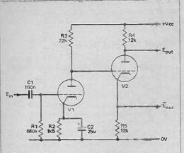
Fig. 16 Split-load phase splitter circuit
