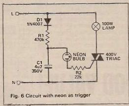
Yet another use for a neon bulb is as a trigger for triacs and SCRs. Figure 6 shows the general idea. This circuit will flash a mains lamp if you have an urge to do such a thing. Figure 7 shows a circuit for an electric fence energiser. These are more by way of tech tips than projects, although Fig. 6 will work perfectly well as it stands.
