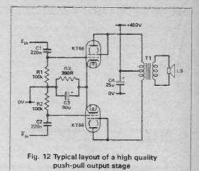
up to 400V, which would allow a peak-to-peak output voltage swing of some 250V before clipping.
