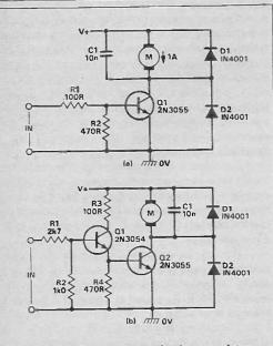
Fig. 10 On/off motor control using transistor switching and (b) increased sensitivity
