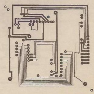
The digital joystick-to-mouse conversion foil pattern topside
