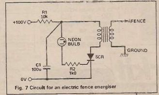
When you're experimenting with any of these circuits, do be careful — none are isolated from the mains. Also bear in mind that the caps can retain enough charge to give a shock even when the mains is disconnected, so discharge each one through a 100R resistor before making any mods to the circuit.
