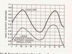
Fig.6 Annual output of a solar cell using a maximum power controller
