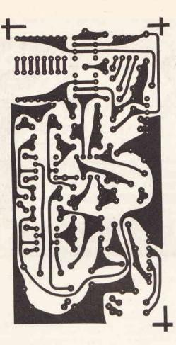
The modular pre-amp input stage solderside foil
