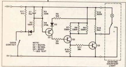
car (negative earth) to keep the light on for a few seconds after the doors have been closed, then fade out gently.
