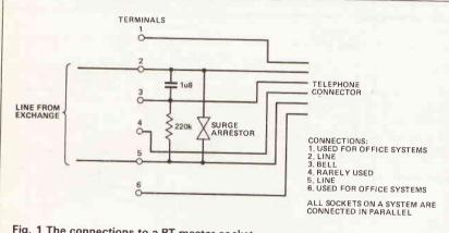
Fig. 1 The connections to a BT master socket
