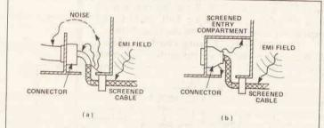
Fig.3 (a) Radiated EMI can enter a screened enclosure via a screened lead but (b) can be prevented with good practice
