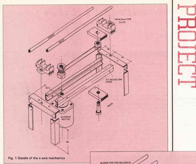
the details of the x-axis, Fig. 2 the y-axis, and Fig. 3 the details of the open solenoid carrier. Note that the x-axis carries the y-axis and motor, so care must be taken to ensure that adequate section sizes are used to prevent sagging of the support rails.
