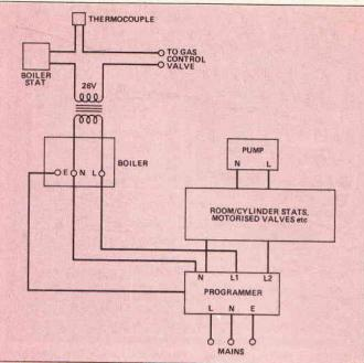
24V on the external circuits for safety reasons. It would certainly seem risky to use mains on a room thermostat unless its cover were made stronger than most I have seen in use.
