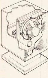
17in.). The Super PP kit includes drive units, high/ low pass crossovers, grille fabric, reflex port, binding post connectors, Flatpack cabinet kit(inc. stand) accurately machined from smooth MDF. Easy assembly - no woodworking or electronic skills required! Suitable for amplifiers of 40 - 200 watts per channel.
