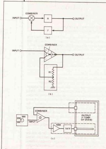
Fig.1 (a) The stripped bare diagram of the single loop feedback system (b) A practical version (c) Another
