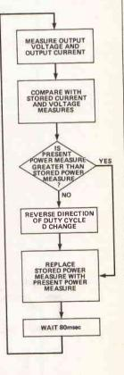
Fig.8 Operation of a switched mode optimum power controller
