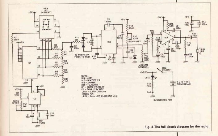
using the PCB. Build from the resistors up, sockets are recommended for ICs and for the display LED — the legs on this device are pretty fragile and it is also static sensitive so take the normal static precautions.
