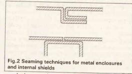
In the case of severe EMI radiation, use grid with perforation holes no greater than 2mm in diameter and ensure several copper jumpers are used, where the spaces between them never exceed one tenth the wavelength of the expected EMI. So if the potential EMI is known to be around a frequency of 27MHz (CB frequencies) then jumpers should be no further apart than about a metre. If the EMI is around 300MHz then jumpers should be less than 10cm apart.
