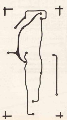
The modular pre-amp disc input stage topside foil
