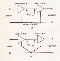
Fig.7 Earth loops can occur at PCB level (a) if separate earth points are used but (b) can be eliminated with a common earth
