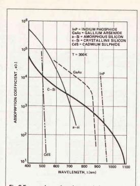
Fig.2 Energy absorption characteristics of various types of solar cell
