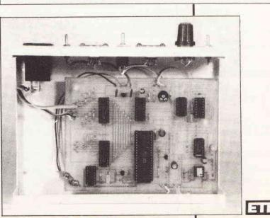
Ali Taalf keeps track of his extensions with this simple in-use signal for telephone circuits
