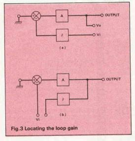
There's one more term I should introduce this month, and that's the *return difference*. In the equation for the gain of the network of Fig.2a, the 1 +  $A\beta$  term is called the return difference — don't ask me why. Calling the various parts of the gain formula by name, it becomes:
