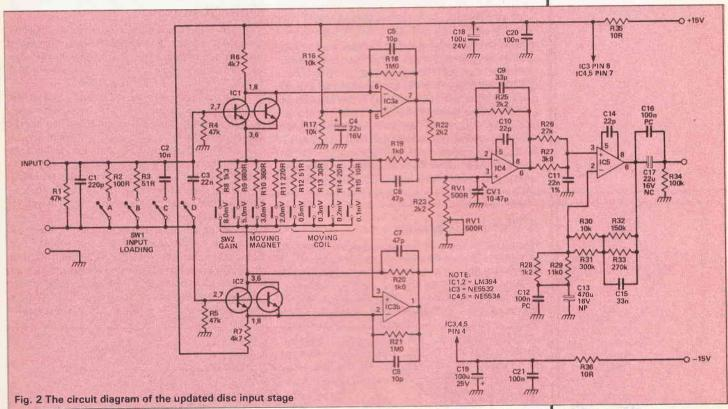
interconnecting cable between cartridge and preamplifier is rejected by the differential action of IC4. In order to fine tune this rejection, RV1 and CV1 are adjusted at low and high frequencies respectively, until the common mode signal is at a minimum. With care, it is possible to reduce the output level of any common mode signal within the audio band by 70dB or more, usually taking it below the noise floor of the amplifier. The method of adjusting the common mode rejection is as follows:
