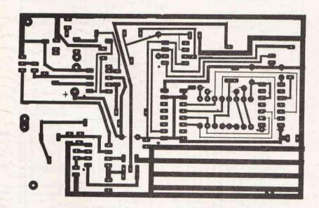
The digitally tuned radio PCB foil
