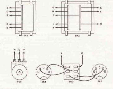
Fig. 5 Off-board wiring diagram
