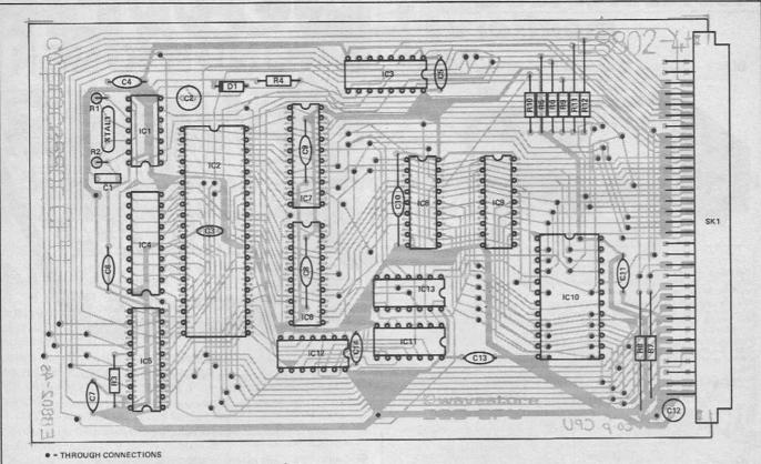
Fig. 4 The component overlay for the CPU board
