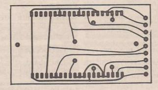
The Transistor Tester display board
