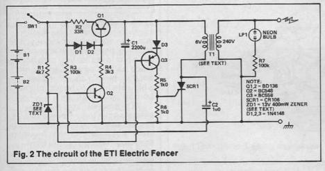
is discharged once every second or so through the transformer T1 which produces a high voltage pulse across its secondary windings.
