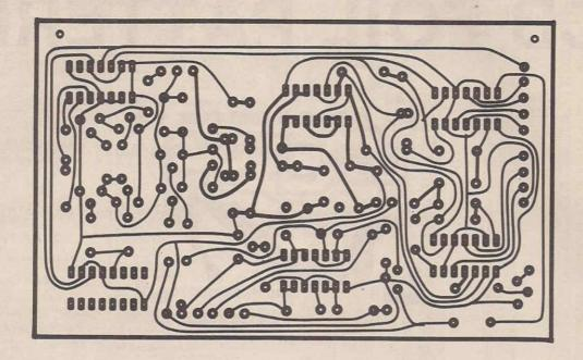
The Transistor Tester main board
