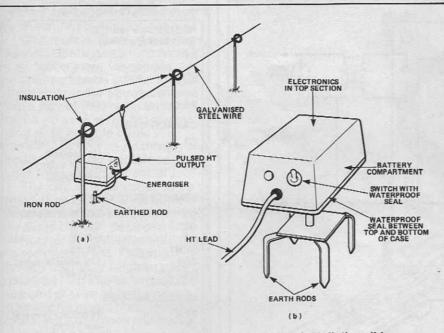
Fig. 1 (a) The main components of an electric fence installation. (b) Commercial fence energisers often have earth rods attached to the case. If you follow this idea for your own fencer, bear in mind that short earth rods won't make good contact in dry weather. When you water your plants, you may have to water your fencer too!
