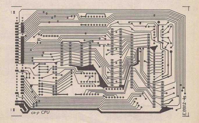
The Co-processor CPU board solderside foil
