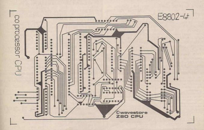
The Co-processor CPU board topside soil
