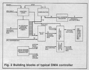
incremented write-fixed address mode or (if the system is configured with two fixed address registers) to read-incremented write-incremented (for memorymemory transfers) and then triggered.
