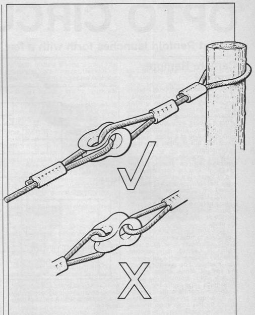
Fig. 5 The right and wrong way to use a 'figure eight' end insulator
