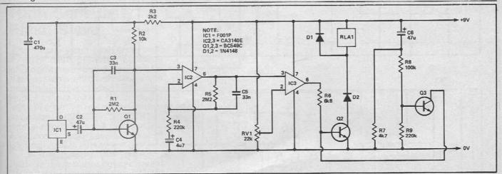
stand-by conditions the output of IC3 is in the low state and both Q2 and the relay are switched off. When the unit is activated, the output voltage of IC2 swings well outside its normal limits and on positive excursions it goes above the reference voltage. IC3's output then goes high, Q2 is switched on and the relay is activated.
