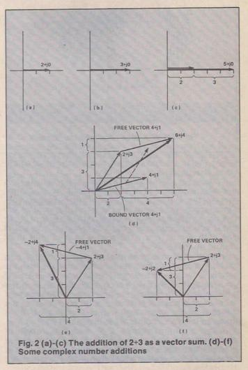
different position, it is said to be *free*. The rule for shunting vectors about is demonstrated in Fig. 2d. They keep the same length and direction at all times.
