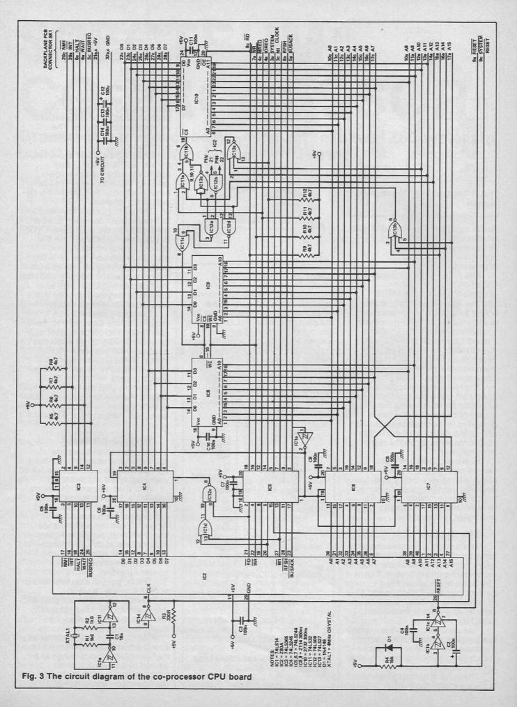
The CPU card consists of the Z80 microprocessor itself (IC2) along with the various buffers, memory devices and 'glue logic' required to make the Z80 run software.
