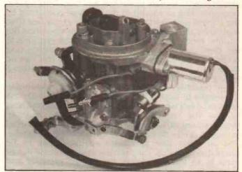
Prototype electronic carburettor designed by Weber for Fiat,
