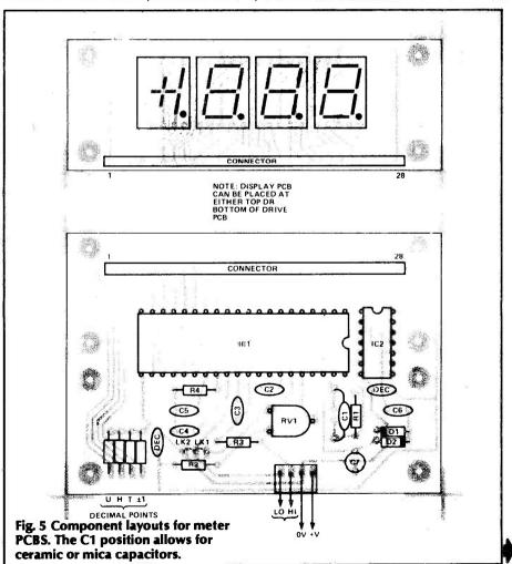
that the common mode voltage range will be roughly  $\pm 4.5 \text{V}$  to -2.5 V. If either meter input is taken beyond these limits, the readings will not be accurate, and if either input goes outside the range of  $\pm 5 \text{V}$  to  $\pm 3 \text{V}$ , IC1 may be permanently damaged.
