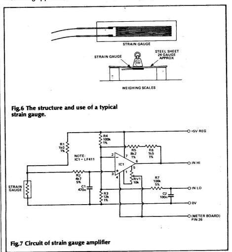
it can be picked up and placed in position by means of adhesive tape applied to the top surface. Hold the gauge firmly in place while the glue is curing, and make sure there are no air bubbles underneath.
