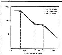
Fig. 1 The desired frequency response of an RIAA preamp.
