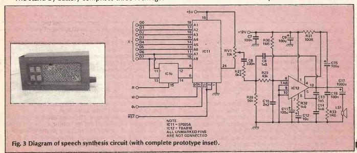
oscillator. The hand shake lines of IC11 are connected to the data bus so that the Z80 can recognize when to
