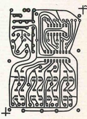
The foil pattern for last month's BBC Motor Interface board, reproduced here because the foil pattern in the July issue shows it at the wrong size!
