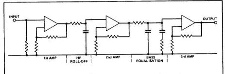
Fig. 6 Using three stages simplifies the component value calculations.
