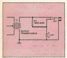
and a rating of a quarter of a watt. This is connected across the normally closed contacts of the
