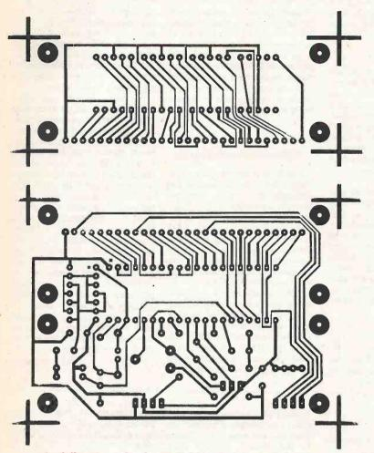
The foil patterns for the Digital Panel Meter boards.
