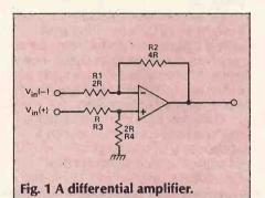
to put it another way, good common mode rejection, will greatly attenuate noise voltages. This is one good reason why balanced lines are often used in preference to single-ended ones for low-level signals. In instrumentation circuits, transducers are often incorporated in a bridge arrangement; common mode signals can arise from
