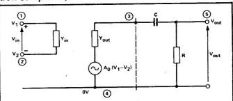
Fig. 6 Op-amp equivalent circuit with frequency compensation.
