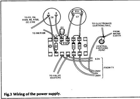
off pillars. If you do this, make sure the pillars are long enough to prevent the valveholder pins touching the case metalwork and use either nylon pillars and/or sleeved connections so that there is no risk of a pin shorting to the pillar. Bear in mind that the layouts in Figs. 2 and 3 show the underside of the valveholders and that the connections will run in reverse order if you are wiring them from above.
