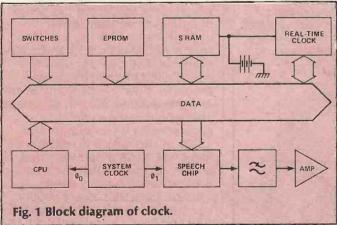
Clock signals for the Z80 and the SP0256 are provided by a common crystal oscillator and divider chain. The MSM5832 uses a second crystal oscillator as its time reference. Battery backup ensures the clock will keep and remember the alarm setting during power cuts.
