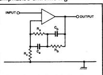
Fig. 2 A typical shunt-feedback equalisation arrangement.
