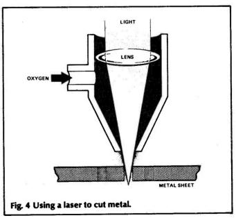
lasers an attractive proposition for critical metal cutting operations in the aircraft industry and elsewhere. The hot swarf produced during cutting can be burnt away using oxygen (Fig. 4).
