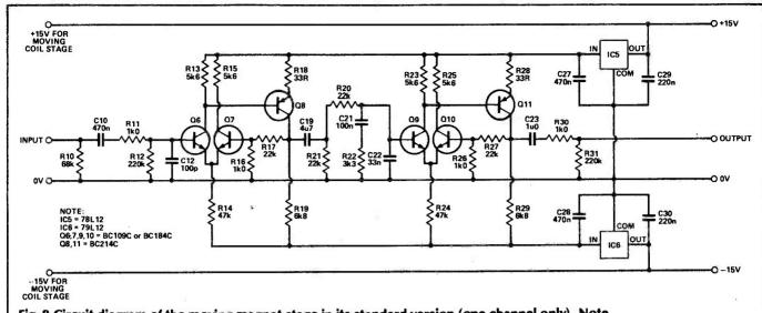
Fig. 8 Circuit diagram of the moving magnet stage in its standard version (one channel only). Note that the component numbering follows on from last month's moving coil stage.
