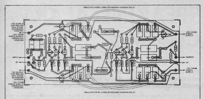
Fig. 10 Component overlay for the moving magnet stage PCB. Note that the supply rail connections at the left-hand end perform different functions in the two versions.
