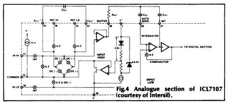
regulator which establishes a reference voltage 2.8V below the positive supply voltage, available to the internal circuit, and also to circuitry outside the IC via pin 32.
