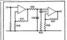
Fig. 7 The two-stage equaliser which forms the basis of this design.
