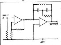
Fig. 4 Combined shunt and series feedback arrangement.
