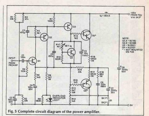
This helps give a good sound quality. The transistor used for Q3 should be capable of supporting some 80V collector-emitter potential and have a permitted dissipation in excess of 550mW. Apart from this, the type used isn't particularly critical.
