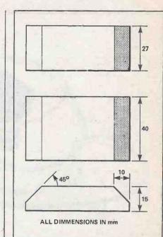
Fig. 4 Details of the foam rubber padding pieces. One of each size is required for each control box.
