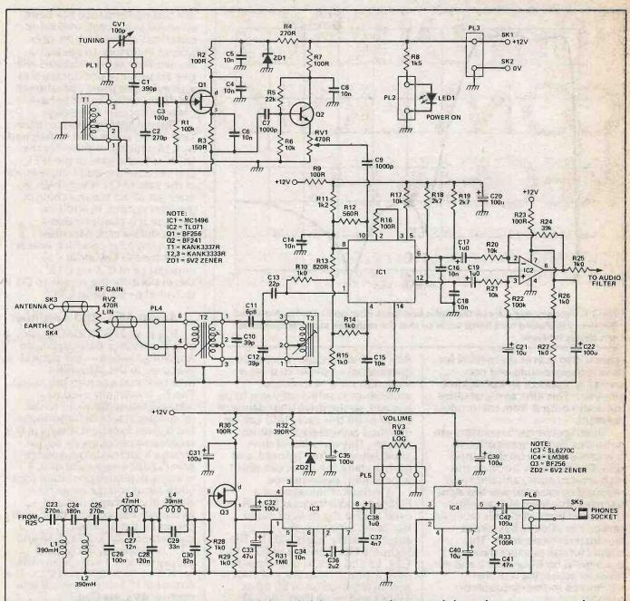
Fig. 2 Complete circuit diagram of the receiver. It is intended that an external 12V supply is used, so no power supply circuitry is shown here.
