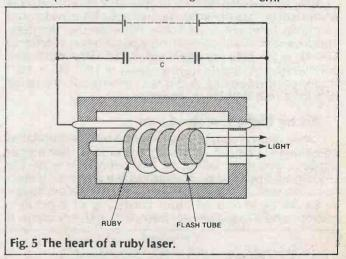
The end faces of the rod were silvered in order to amplify the light. One end acted as a perfect reflector but the other end was only a partial reflector so that the radiation could burst through. Ruby was ideal because it is easy to cut and shape.
