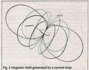
In contrast to the electric field of normal radio communications, which radiates in straight lines from the aerial, the magnetic field is made up of closed elliptical
