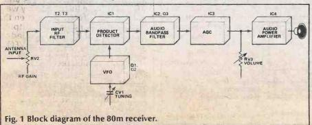
amplified, forming the audio output of the receiver. Since most amplification and filtering take place at audio frequencies, the performance of a direct conversion receiver depends on high audio amplification and a selective audio filter.
