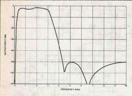
Fig. 3 Frequency response of the audio bandpass filter up to 10kHz. Note that frequency is plotted on a linear scale so that the response at low frequencies can clearly be seen.
