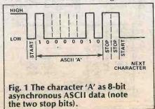
There are typically between five and eight of these data bits, each one being a high or low state of equal duration to that of the start bit. The least significant bit is transmitted first.
