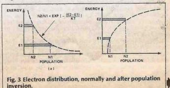
move to the outer orbits until there are more of them there than in the inner orbits, a situation known as a population inversion (Fig. 3b). The electrons will not be stable in this state and will fall back to their previous energy levels within a few nanoseconds producing a spontaneous emission of light. As a result, this system produces pulsed rather than continuous emission.
