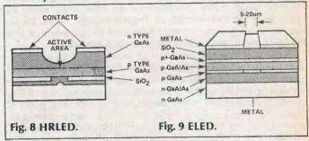
The important feature is the stripe etched on the top which helps concentrate the emission from a very small area. The reflex index of the stripe needs to be uniform so that the output characteristic is a straight line.
