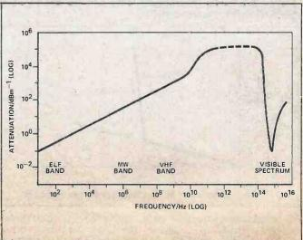
Fig. 1 Attenuation of electromagnetic waves in sea water.
