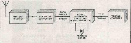
Fig. 8 Converting 50 baud RTTY signal to 300 baud for a computer.
