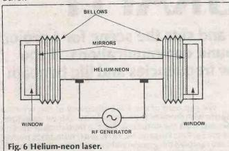
The object of using mirrors is to amplify the light by bouncing it back and forth. Nothing could be simpler, it's all done with mirrors and since weare dealing with light it seems logical to use mirrors. However since the gas is at low pressure, the mirrors have to be adjusted in a virtual vacuum which is not easy. This is now overcome by using external spherical mirrors.
