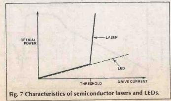
Stimulated emission is of higher fidelity than spontaneous emission because photons stimulate other photons of the same wavelength. Hence the linewidth of lasers is 1 nm  $(10^{-9} \text{ m})$  whereas the linewidth of LEDs is
