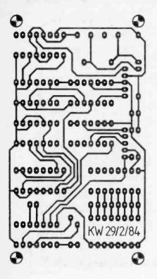
The top and bottom patterns for the scoreboard controller module.
