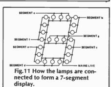
The displays themselves are pygmy bulbs in bulb holders, mounted on a wooden panel. 15W bulbs should give sufficient light for most applications. Three bulbs are used for each segment as shown in figure 11, but for larger
