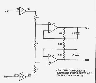
Fig.2 Block diagram of the circuit in pseudo-stereo mode.
