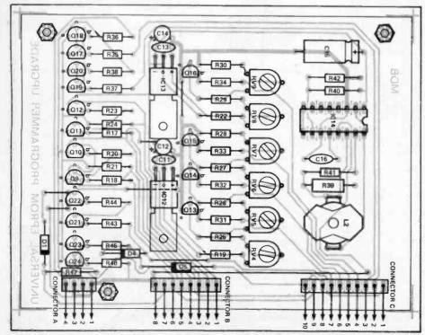
Fig. 2 Overlay diagram of the upgrade board.
