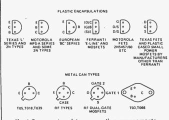
Fig. 1 Common transistor connection arrangements.
