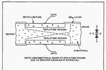
Fig. 4 Cross-sectional view of an N-channel FET, showing the depletion regions which result when the device is just biased to cut-off.
