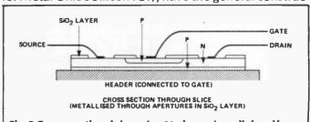
Fig. 5 Cross-sectional view of an N-channel small signal junc-
