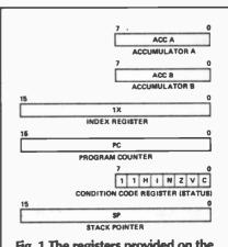
Fig. 1 The registers provided on the 6802.
