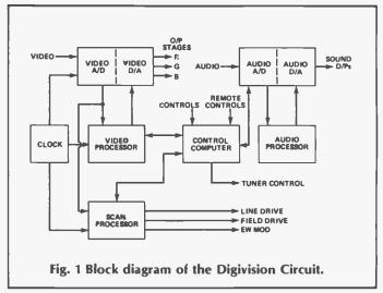
though the designers missed a trick here. If they had employed PWM (pulse width modulation) to drive the speakers there would have been no need of an analogue output stage which generates considerable distortion. In between the A/D and D/A conversions, another chip takes care of the sound signal processing. It includes the ability to deal with two-carrier TV stereo signals.
