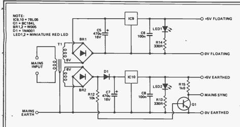
The power supply is in two sections, each of which has a bridge rectifier and a smoothing capacitor followed by a voltage regulator (ICs 9 & 10). C6 and C8 cut out any high frequency spikes and protect the regulators from oscillation. Each section is also fitted with a LED and current limiting resistor as a visual check of operation.
