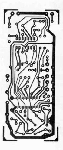
The mono-to-stereo simulator foil pattern.
