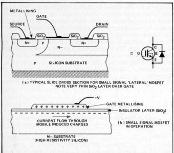
Fig. 6 Cross-sectional views showing the construction and operation of a MOSFET.
