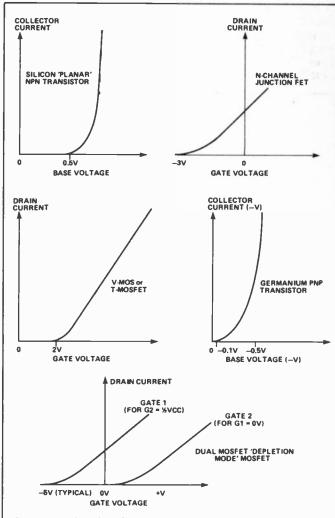
Fig. 9 Graphs showing the input voltage/output current characteristics of different types of transistor.
