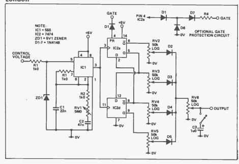
This simple circuit is quite useful for generating a number of functions. It can be used for trilling, vibrato or higher frequency modulation. It will also provide voltages for note sequences, gating, controlling filters, VCA's or any voltage controlled module.
