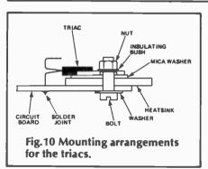
bent down to pass through the board, while the centre pin is bent up for a flying lead connection to the lamps. Only after the triac -heatsink assembly has been completed should the triacs be soldered to the board.
