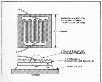
Fig. 10 Sectional views of a 2N3055 power transistor chip.
