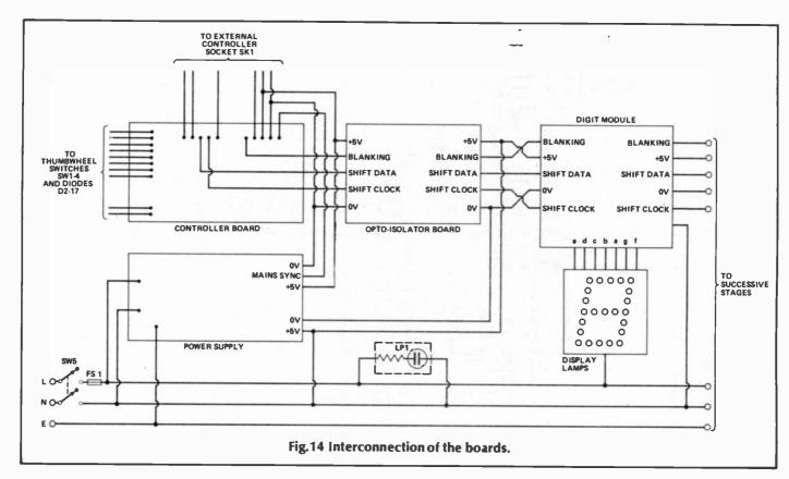
looms, or ribbon cable as appropriate. Make sure that suitable cable is used for the mains supply to the lamps, between the lamps and the triacs, and the returns from the digit driver boards.
