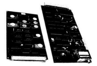
results. Amonochrome monitor or TV may also be used, in which case the colours appear as different shades of grey. Mousepacket provide, as part of the package, two EPROMs which replace TANBUG and one of the BASIC EPROMs, hence allowing the system to handle the new display in a way which will be transparent to the user. **Reference:**
