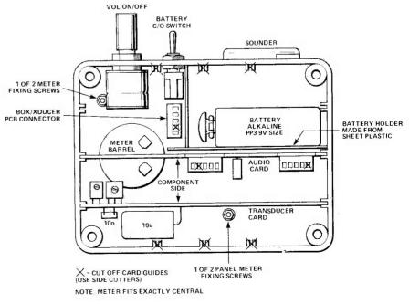
Fig. 5 Layout of the principal components in the case.
