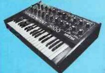
This professional quality 3-octave instru-ment is transposable 2 octaves up or down, giving an effective 7-octave range. There is portemento pitch bending,VCO with shape and pitch modulation, VCF with high and low pass outputs and separate dynamic sweep control, noise generator and an ADSR envelope shaper. Other features include special circuitry with precision components to ensure tuning stability.
