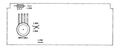
Fig. 8 Overlay diagram of the transducer PCB showing the modified arrangement to accommodate the MPX100A.
