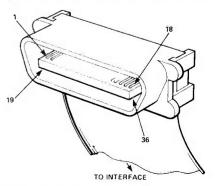
Fig. 1 Pin designation of the Amphenol connector.
