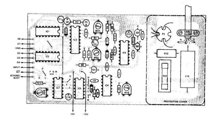
Fig. 2 Overlay diagram of the PCB.
