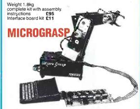
A real programmable robot for under £300! Micrograsp has an articulated arm jointed at shoulder, elbow and wrist positions. The entire arm rotates about its base and there is a motor driven gripper. All five axes are motor driven and four of these are serve controlled giving positive positioning. The robot can be controlled by any microcomputer with an expansion bus the Sinclair ZX81 being particularly suitable.
