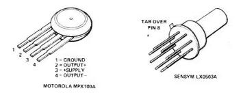
Fig. 9 The LX0503A and MPX100A packages.
