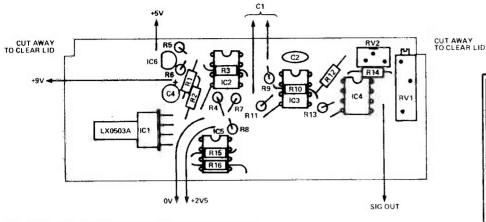
Fig. 6 Overlay diagram of the transducer PCB.
