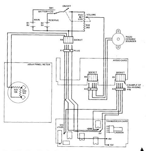
Fig. 10 Interwiring of the circuit boards and external components.
