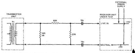
Fig. 4 Circuit for use in receiver test and alignment.
