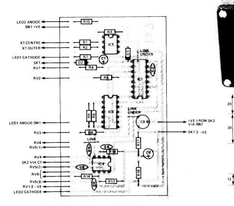
Fig. 2 Overlay diagram of the PCB.
