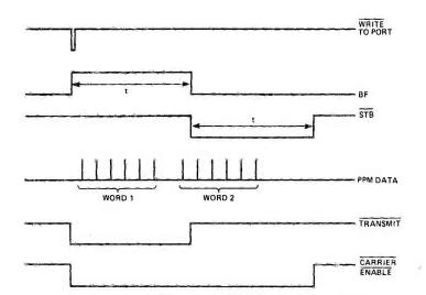
Fig. 7 Timing diagram for the logic used with 8155 and 8255 ports.
