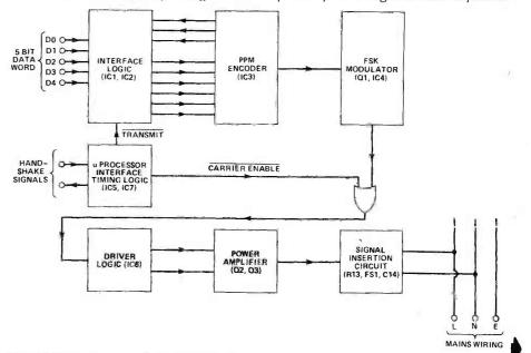
Fig. 1 Block diagram of the transmitter.
