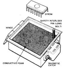
Fig. 3 Construction of the EPROM holder. 18
