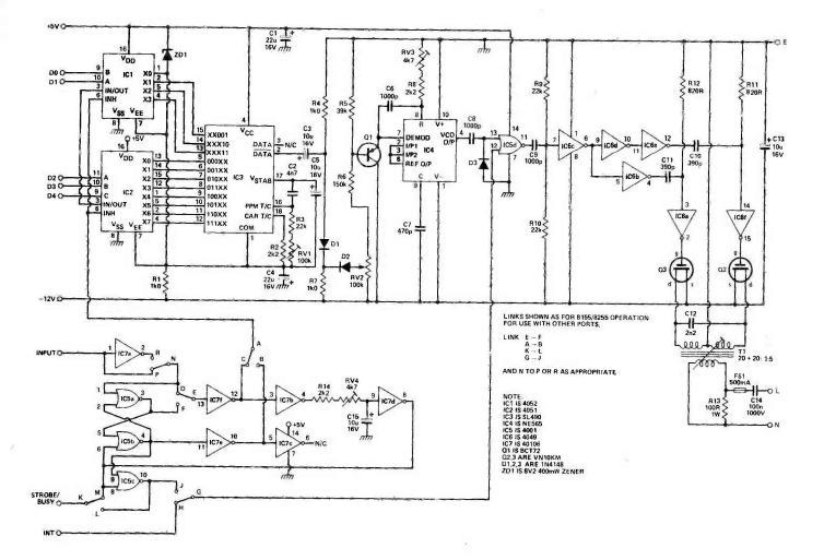
Fig. 5 Circuit diagram of the transmitter.
