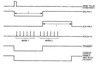
Fig. 8 Timing diagram for the logic used with other ports.
