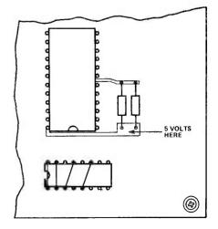
Fig. 4 Location of a suitable 5V tapping point on the MZ-80K PCB.
