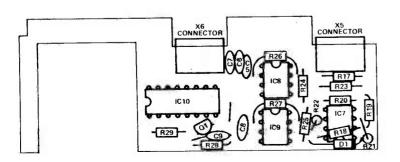
Fig. 7 Overlay diagram of the audio PCB.
