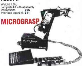
A real, programmable robot for a little over £200! Micrograsp has an articulated arm jointed at shoulder, elbow and wrist positions. The entire arm rotates about its base and there is a motor driven gripper. All five axes are motor driven and four of these are servo controlled giving positive positioning. The robot can be controlled by any microcomputer with an expansion bus—the Sinclair ZX81 being particularly suitable.
