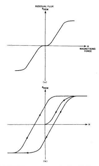
Fig. 9 Tape magnetisation characteristics: (a) for small magnetisations; (b) for large magnetisation.
