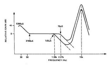
Fig. 12 Record pre-emphasis and de-emphasis for cassettes, showing additional compensation for head losses.
