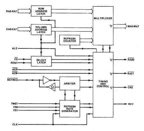
Fig. 7 Block diagram of the TMS 4500A DRAM controller.
