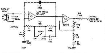
Fig. 13 A typical cassette replay amplifier giving the frequency response shown in Fig. 6.
