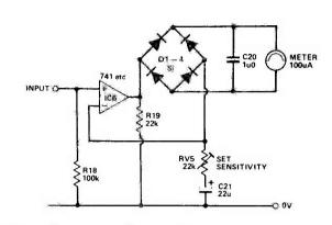
Fig. 16 A simple recording level meter circuit.
