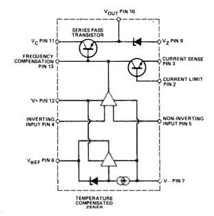
Fig. 2 (left) Equivalent internal circuit of the MC1723.
