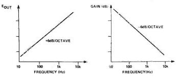
Fig. 2 (left) The theoretical AC output from a tape replay head. Fig. 3 (right) An idealised replay amplifier characteristic.
