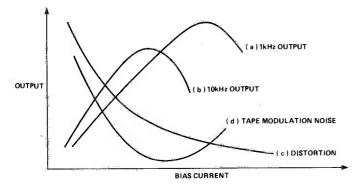
Fig. 11 How recording characteristics vary with bias current; note that only curves a) and b) are to the same scale.
