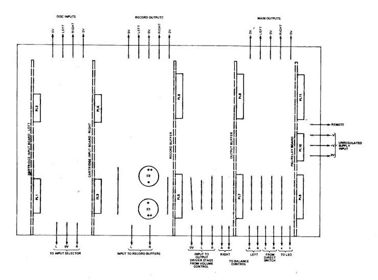
Fig. 4 Here is the overlay diagram for the mother'board of the preamp as featured in the first part of the description in December '83; this board will be available through the PCB service. However, we have not reproduced a lay-out for the mother board of the extended system because the whole idea is for it to be adaptable to your needs — so everyone can make up their own, customised preamp using the same basic blocks.
