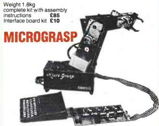
A real, programmable robot for under £200! Micrograsp has an articulated arm jointed at shoulder, elbow and wrist positions. The entire arm rotates about its base and there is a motor driven gripper. All five axes are motor driven and four of these are servo controlled giving positive position into the robot can be controlled by any microcomputer with an expansion bus – the Sinclair ZX81 being particularly suitable.
