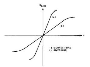
Fig. 10 The effect of HF bias on tape magnetisation linearity.
