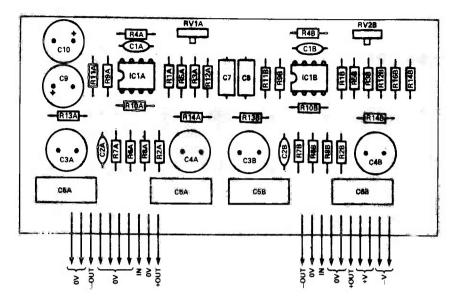
Fig. 2 Overlay of the PCB for the balanced output driver — this is a stereo board, so only one is required, but note the components that you have to obtain two of.
