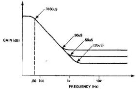
Fig. 6 A practical replay equalisation characteristic for reelto-reel tape-recorders which conforms to NAB recommendations (cassette replay to BSI/DIN specifications would use 70/120 us).
