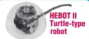
For under £100, Hebot II takes programming off the VDU and into the real world. Each wheel is independently controlled by a computer, enabling the robot to perform an almost infinite number of moves. It has blinking eyes, a two-tone bleep and a solenoidoperated pen to chart its moves. Touch sensors coupled to its shell return data about its environment to the computer enabling evasive or exploratory action to be calculated.
