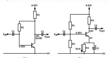
Fig. 3 (a) and (b) single transistor amplifier stages. Both these employ feedback in the setting of the operating point, but not in the signal path (assuming that the source output impedance is much lower than the value of R1 in (a).
