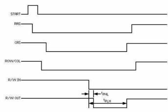
Fig. 4 Normal read-modify-write mode.
