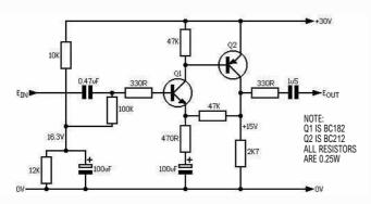
Fig. 4 A two stage transistor amplifier with a gain of 100.
