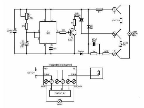
The usual precautions with mains wiring must be observed. In particular, remember that, although the 555 is on a 12V supply, that supply is
