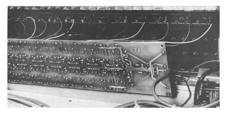
This photograph shows the connections between the slider pots on the front panel and the PCB - and the mounting of the front panel using struts and spacers. Note that we couldn't fit the prototype PCB into our equipment and had to make it in two sections - hence the join!
