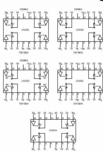
Fig. 7 Pin outs: LF1331 is four normally open switches with disable; LF13333 is two normally closed and two normally open with disable; LF13201/2 are as LF13331/2 but without disable.
