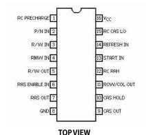
Fig. 1 Pin out of the 74LS608.
