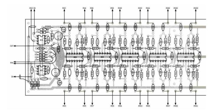
Fig 1 Overlay diagram for the PCB.
