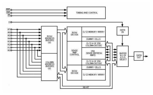
Fig.1 Internal architecture of the TMS4164 DRAMs used in the project.
