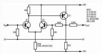
Fig. 5 DC amplifier (with a gain of 10) using an input iong-tailed pair, Q1 and  $\Omega$ 2
