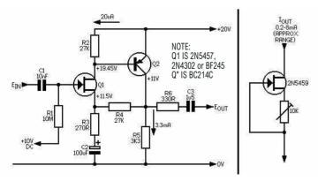
Fig. 11 (Left) Two stage FET amplifier with overall negative feedback gain will be 100 and input impedance will be 10 Megohms. Fig. 12 (right) Use of a junction FET as an adjustable constant current source.
