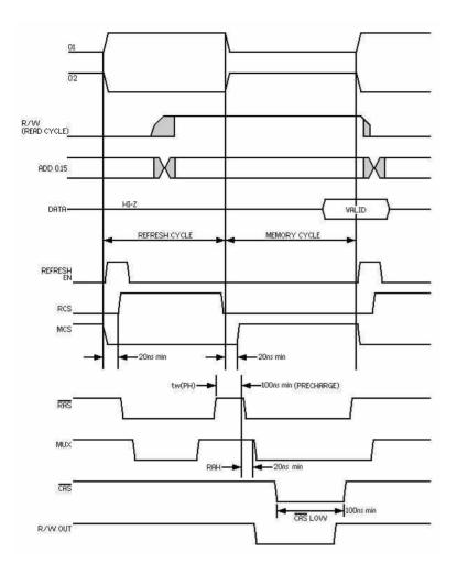
Fig. 2 Processor and memory cycle controller timing.
