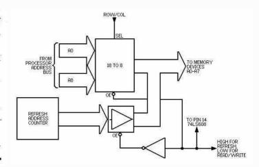
Fig. 6 Typical circuit for use with 64K by 1 DRAMs; for refresh, pin 14 is taken high, pin 13 is pulsed high, and refresh address is placed on the memory devices address pins.
