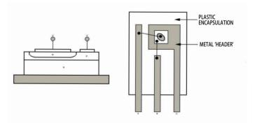
Fig. 1 (a) Cross section of a die; (b) a complete small-signal transistor.
