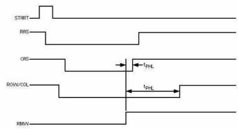
Fig. 5 Normal read-modify-write with abort after read.
