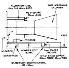
Fig. 7 The internal construction of the oscilloscope
