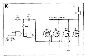
Fig. 10 Paralleling output VMOS FETs can be done simply because they are inherently thermally stable.
