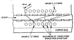
Fig. 3 Plan view of Roadrunner wiring. No more than than three pins should be wired from each break in the strip.
