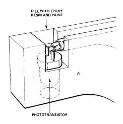
Fig. 2 Constructional details of our sensor. Using different sized jack plugs will prevent incorrect connection.
