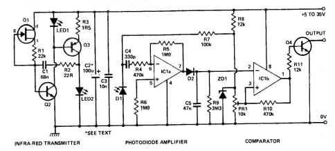
Fig. 2 Circuit diagram for the sensor.
