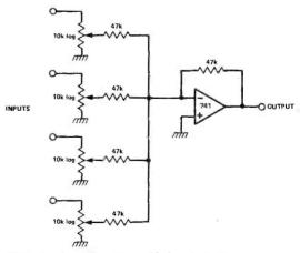
Fig. 10 A simple audio mixer with four inputs.
