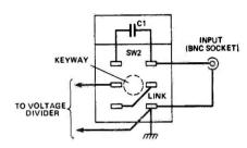
Fig. 8 The wiring details for SW2.
