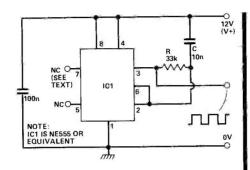
(R in ohms, C in microfarads), mark/space ratio of typically 3:2, and voltage swing of 1 to 11 V. These figures were found using a load impedance of 330k; the frequency is affected if load impedance is less than about 10 x R, but if low impedances are to be driven, pin 7 can be used and the load wired from pin 7 to power: alternatively, a 1k5 reistor can be taken from pin 7 to power and the load put between pin 7 and ground, though this reduces the available voltage swing at pin 7.
