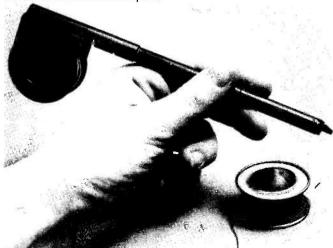
The Quick/Connect wiring pen and bobbin.
