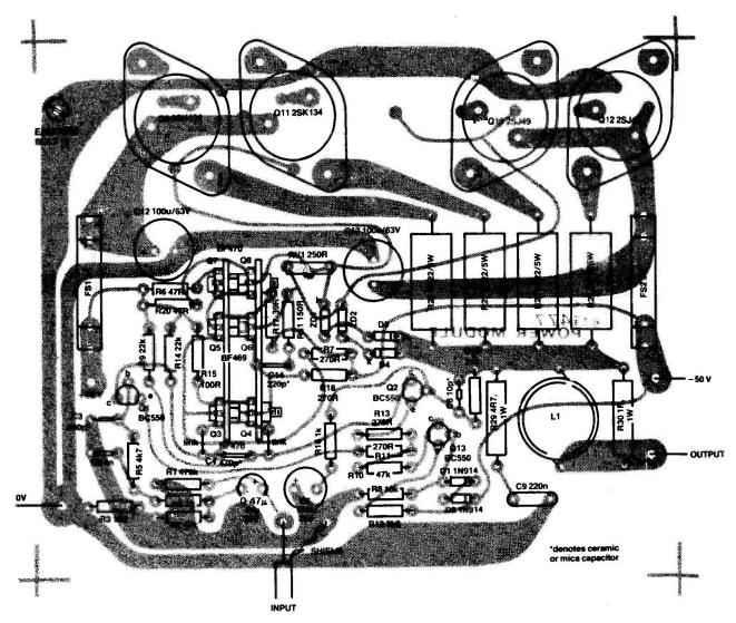
Fig. 2 Component overlay of the MOSFET amp module.
