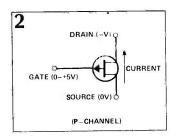
Fig. 1 A field effect transistor (FET) is a doped-silicon resistor, the resistance of which can be varied by changing the electric field through it.
