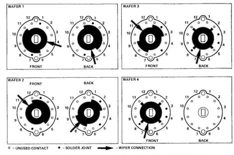
Fig. 2 SW1 contact wafer arrangement. Use in conjunction with the circuit diagram published last month.
