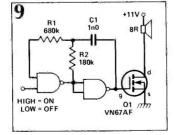
Fig. 8 TTL gate logic can be used to control VMOS FETs but a gate pull-up resistor must be used to ensure that the FET gate reaches a high enough voltage to allow sufficient current flow through the FET.
