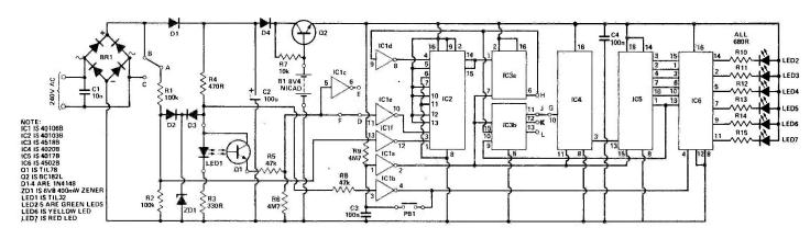
Fig. 1 Circuit diagram of the ETI Stylus Timer. The various lettered links are used to select the timing period (see text).
