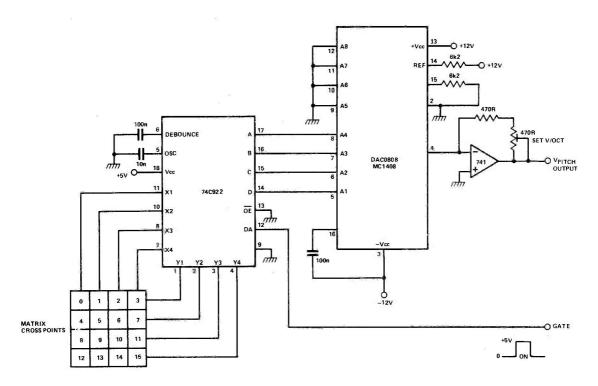
Fig. 6 A digital keyboard, in this case for a 16-note range.
