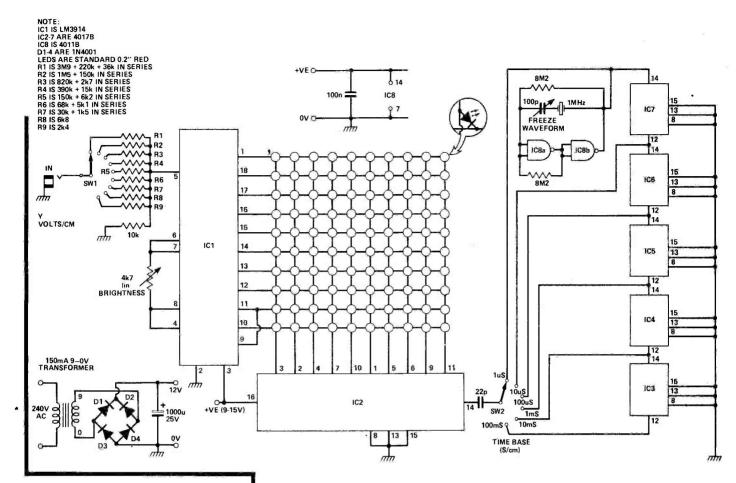
10 Hz, causing IC1 and IC2 to scan the keyboard (each one clocks on by one alternately). IC4 is held off by IC3a. If the stylus is placed on one of the drawing pins, nothing will happen until the counters get to that pin. At this point they stop and IC4 turns on, producing a note. The pitch of the note depends on which preset is driving pin 7 of IC4. The note stays on until the probe is removed from the pin, whereupon everything carries on as before.
