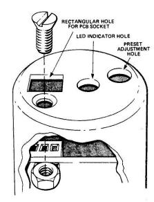
Fig. 3 This is how we mounted the PCB in the aluminium tube. The nut is soldered to the ground track under
