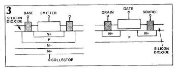
Fig. 3 Cross-sections through a) a bipolar transistor; b) a field effect transistor.
