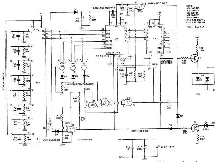
Fig. 1 The complete circuit diagram for the ETI Logic Lock. A general-purpose output is provided; next month several application circuits are given to suit mains or DC solenoids.
