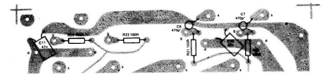
Fig. 3. This overlay shows the components which are mounted directly on the copper side of the PCB.
