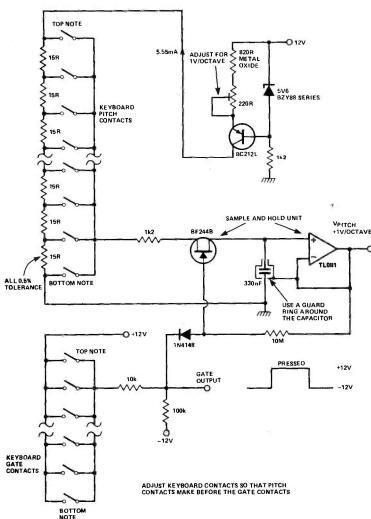
Fig. 5 Typical monophonic synthesiser keyboard unit.
