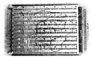
This photo shows the underside of a Quick/Connect Eurocard. Interwiring of the components is done between the tines and a data bus, for example, is easily wired (left of board). At the top of the page you can see the component side of this board; ICs are especially suited to the system.
