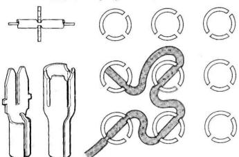
Fig. 1 Working anticlockwise from the top left, we have the IDC principle, the Quick/Connect and Speedwire pins, and a diagram showing the Speedwire termination technique.
