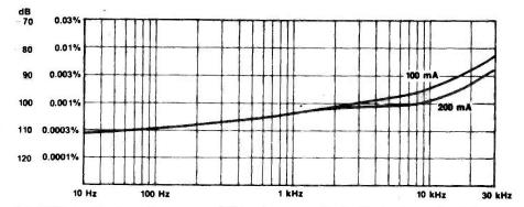
Fig. 4 This graph shows the measured distortion versus frequency for two values of quiescent current in the output stage.
