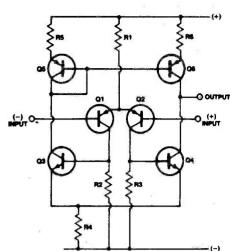
Fig. 1 The basic voltage gain stage of the ETI-5000 MOSFET amplifier.
