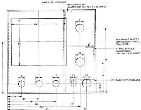
Fig. 6 The front panel drilling details.
