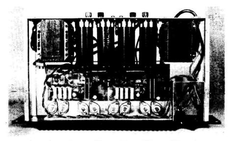
A general view showing the internal layout of the amplifier. Toroidal transformers can be used instead.
