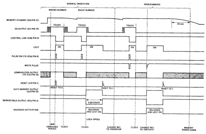
Fig. 2 Timing diagram for the Logic Lock logic! It will repay careful study in conjunction with the circuit diagram and How It Works section.
