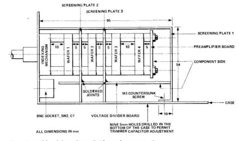
Fig. 1 Assembly of the voltage divider and preamp unit.
