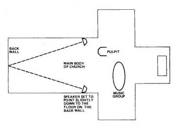
Fig. 8 The working layout of the speakers in the church.
