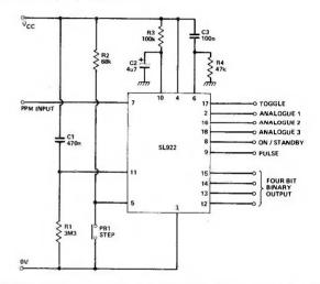
Fig. 6 Circuit diagram of a remote control receiver using the SL922. A preamplifier is required at its input.
