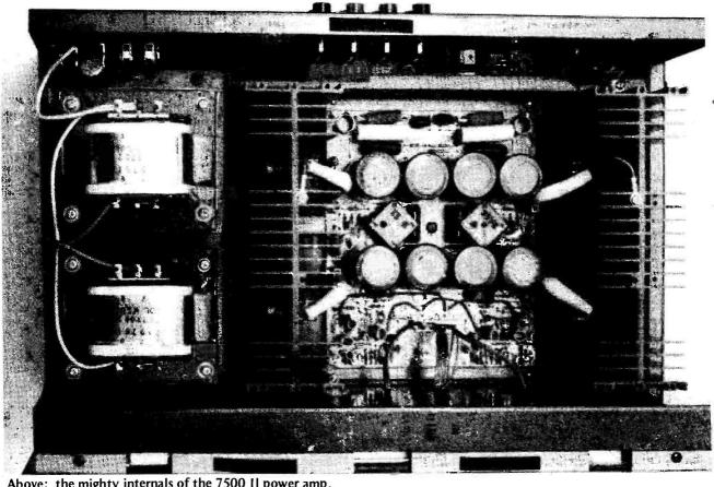
Above: the mighty internals of the 7500 II power amp. Those huge transformers endow the machine with excellent separation and good power delivery.
