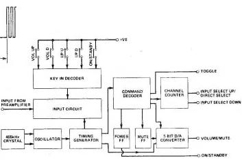
Fig. 10 Block diagram of the uPD1937C remote control receiver.
