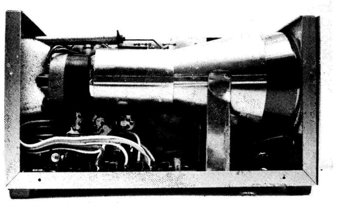
The tube is supported by its metal screen and cushioned by foam draught excluder. The power supply is mounted beneath it.
