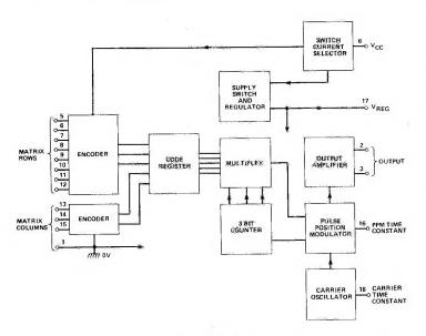
Fig. 1 Block diagram of the SL490 remote control encoder.
