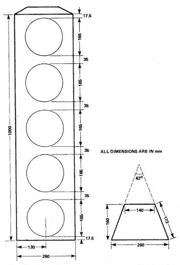
Fig. 7 Cabinet details — all dimensions are in millimetres. The total cabinet volume is 0.324 cubic metres. A suitable material to use is  $\frac{34}{}$  chipboard and this thickness needs to be added to the dimensions shown where appropriate.
