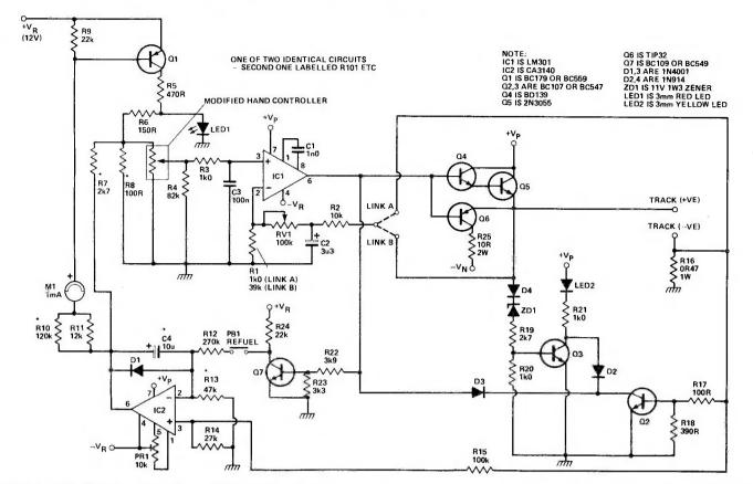
Fig. 1 Circuit diagram of one channel of the controller.
