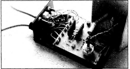
With the lid off, the general layout of the project should be clear. With the large currents involved, the mains wiring is secured to the PCB with nuts and bolts.
