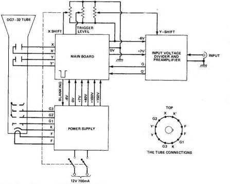
Fig. 4 Block diagram of the oscilloscope.
