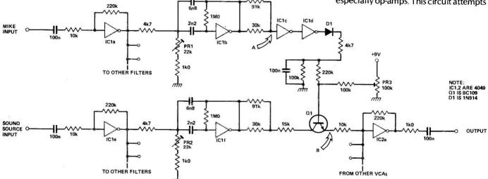
Fig. 1 Circuit of one channel of the CMOS vocoder.
