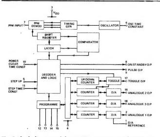
Fig. 5 Block diagram of the SL922 remote control receiver.
