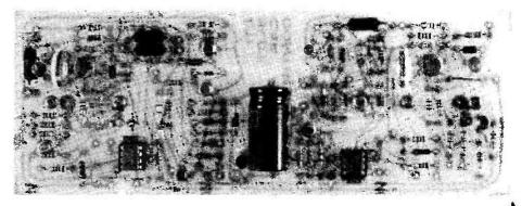
The slot car controller board before interwiring.
