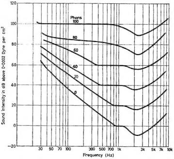
Fig. 1 Above: the Fletcher-Munson graphs of equal loudness. The curves plot the amount of energy required to produce a sound of equal intensity at the ear, for varying frequencies.
