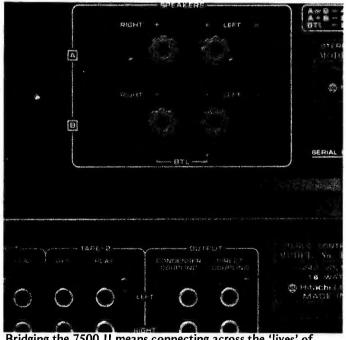
Bridging the 7500 II means connecting across the 'lives' of the two sets of speaker terminals. This is denoted by the obscure legend BTL. It actually stands for "Bridge Transformer Less"! I kid you not.
