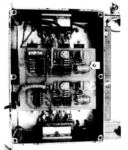
The analogue PWM board installed above the dual motor driver.
