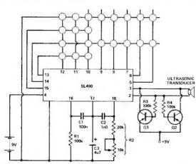
Fig. 4 The addition of transistors Q1 and Q2 increase the range of the transmitter to about 10 m.
