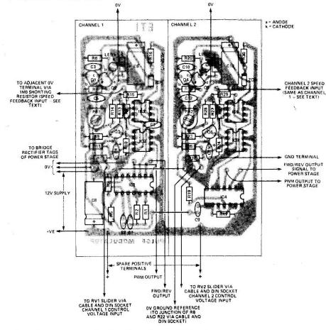
Fig. 2 Component overlay for the analogue PWM unit.
