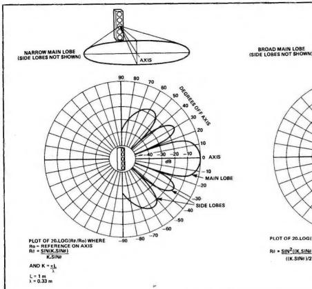
Fig. 3 Polar diagram of a column loudspeaker at 1 kHz.
