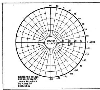
Fig. 1 Polar diagram of a sound source which radiates equally in all directions (approximated by an unmounted loudspeaker). The sound source is at the centre of the diagram.
