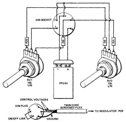
Fig. 1 Wiring diagram for the manual control unit.
