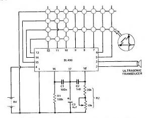
Fig. 2 Circuit of a 21-facility remote control transmitter using the SL490 encoder with an ultrasonic transducer.
