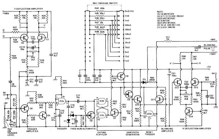
Fig. 2 Circuit diagram of the main board. The two dotted capacitors in parallel with C19 and C20 may be required for trimming purposes - this is covered next month.
