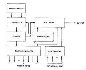
Fig. 7 Block diagram of NEC's remote control encoder — the uPD1986C.
