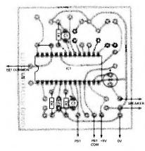
Fig. 2 Component overlay for the gunshot, using the same PCB as all the other sound effect projects. Don't forget to insert the link on the board.
