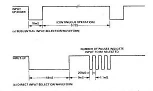
Fig. 12 (a) Sequential input select waveform, and (b) direct input select waveform of the uPD1937C remote control receiver.
