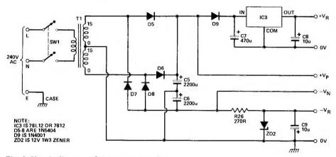
Fig. 2 Circuit diagram of the power supply.
