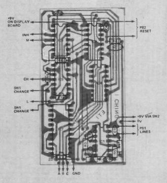
Fig. 4 (Above) Component overlay for the main board.
