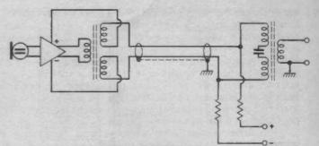
Fig. 8 A-B powering. Both signal wires ares used by means of capacitively-coupled split transformer windings. This avoids using the screen to conduct current.
