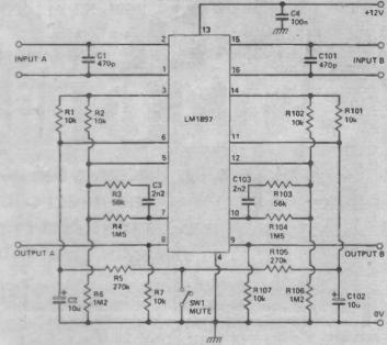
Fig. 5 Circuit of a typical stereo tape (ferric) playback system. To adjust circuit equalisation to suit chromium dioxide tape, see text.
