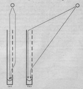
Fig. 10 (a) Sound enters gun microphone from the end and side to arrive at the diaphragm simultaneously when the source is the front. (b) With a source at the side, sound paths differ in length. When the difference is half a wavelength cancellation occurs. This happens over a range of frequencies due to the different spacing of the holes.
