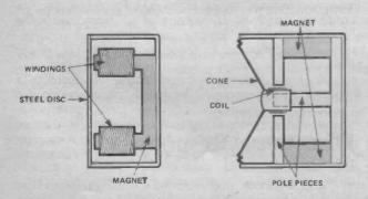
Fig. 3 (Left) Diagram of a moving-iron, or magnetic, microphone.
