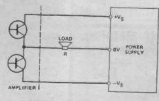
Fig. 1 Split rail power supply configuration.
