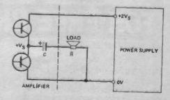
Fig. 2 Single rail configuration.
