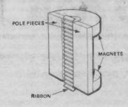
Fig. 5 Dlagram of a ribbon microphone.
