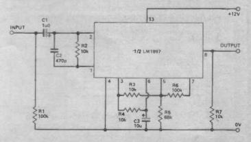
Fig. 6 A capacitively-coupled microphone preamplifier. The flat frequency response of the circuit means that low-frequency noise is not such an important consideration as in a tape playback system.
