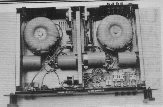
HUAD R R AMPLIFIER Most of the space in this 100 W power amplifier is taken up by the power supply components - and quite right tool
