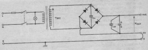
Fig. 4 Power supply for single rail and bridge amplifiers.
