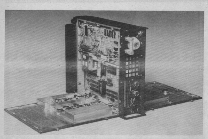
Edge hinges on each side of the case render the Philips Calipac radio exceptionally accessible for servicing and repair. When closed, the unit is nonetheless hermetically sealed and can withstand water immersion to a depth of one metre.
