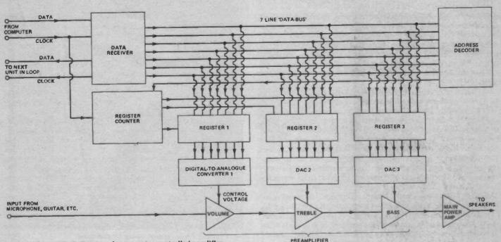
Fig. 2 (Above) Block diagram of a computer-controlled amplifier.
