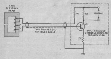
Fig. 3 Simplified details of a direct-coupled tape playback system. The transistor bias resistor is now coupled to the transistor base via the playback head. With a low bias current the DC voltage across the head is low (<1 mV) and the input stage is virtually balanced.
