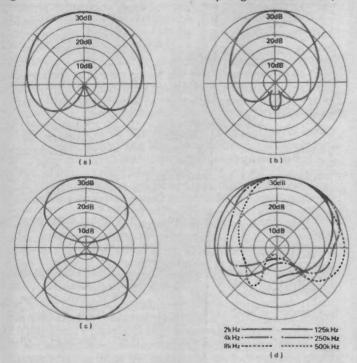
Fig. 9 Polar diagrams of nominal directional response. (a) cardioid; (b) hypercarioid; (c) figure eight; (d) polar response varies with frequency; plots are given for six different frequencies.
