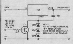
on a 2716/2732 EPROM, selected by a TTL level signal on an output port. After trying various sorts of transistor switches (all of which suffered from an unacceptable voltage loss), the following simple circuit was evolved. The transistor shorts out the zener diodes when it is turned on by a high level (greater than 2V4) signal at the input. Under these conditions, the regulator has its common lead virtually at ground, so it produces + 5 V at its output.
