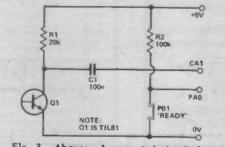
Fig. 3 Above: A suggested circuit for a light-pen for use with the expansion.
