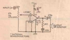
Voltage gain (fixed) = x 50 (34 dB)+ V<sub>CC</sub> range = +8 V to +22 V Typical quiescent current = 7 mA Output power = 2W5 (with speaker = 8R, heatsink fitted)
