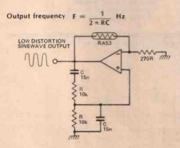
The RA53 is a negative temperature coefficient thermistor; it sets  $A_{\rm V}\,$  to 3 for stable oscillation.
