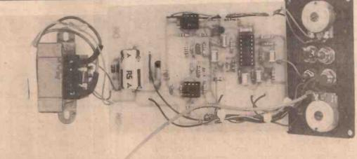
We've pulled everything out of the Sink Box for this photograph, which shows how the interwiring is made.
