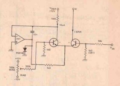
\*Matched transistors in thermal contact
