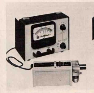
Fig. 3. The Yellow Springs Instrument Co. aspirated psychrometer. The righthand view shows the unit packed for transportation. Thermistors are used as temperature sensors.
