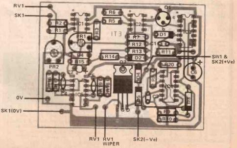
Fig. 1 Component overlay.
