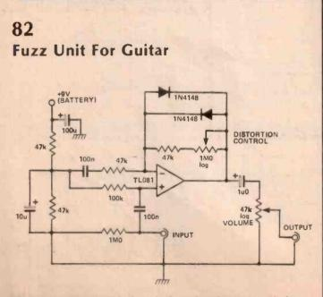
The battery can be switched on via the jack socket (a stereo jack can be used).
