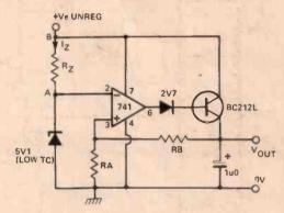
A very low dropout voltage can be obtained by allowing Q1 to saturate. This gives maximum lifetime on battery power.
