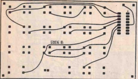
Above: The underside of the keypad PCB for last month's FM Mains Remote Control system.
