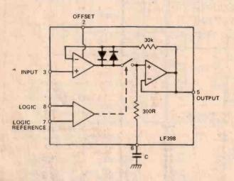
Use a printed circuit guard ring (connected to the output voltage) around the hold capacitor
