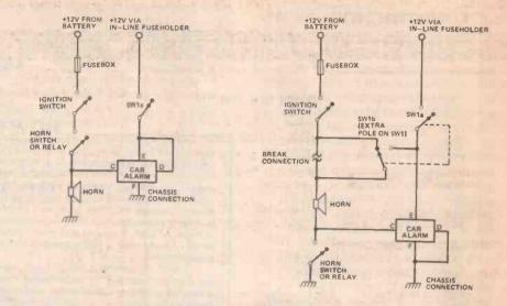
Fig. 2 Common horn circuits and how to connect the alarm to them. The circuit on the left will have only one wire from the horn. The one on the right is found in cars such as the Leyland Mini LS and is rather more complex.
