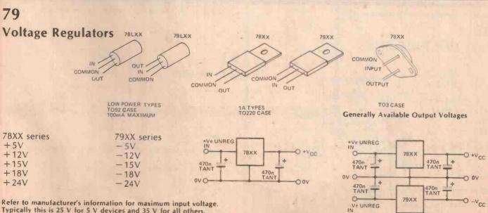
Refer to manufacturer's information for maximum input voltage. Typically this is 25 V for 5 V devices and 35 V for all others. Regulators need about 2 V difference between the unregulated rail and the output rail. Less than this, and the output rail will collapse. Note that the power dissipated in the regulator  $= l_{vac}(V_{vac} = V_{vac})$
