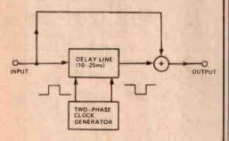
Fig. 1 Block diagram of the double-tracking or echo circuit.
