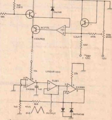
An exponential current source can be used to drive a linear VCO. The VCO then has a 1 V/octave response Devices all powered from  $\pm$  12 V \*Matched transistors in thermal contact
