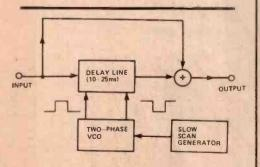
Fig. 2 Block diagram of the auto-doubletracking or mini-chorus circuit.
