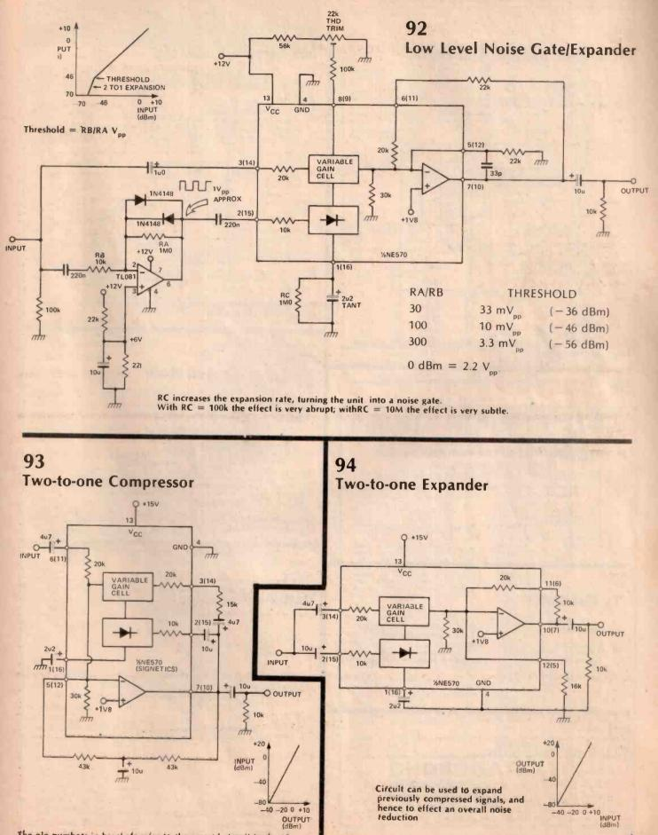
The pln numbers in brackets refer to the second circuit in the IC. Circuit can be used as a preconditioner in a noise reduction system.
