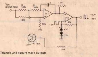
Output frequency  $\mathbf{F} = (1.667 \text{ x } 10^{-7} \text{ x } V_{IN})/C \text{ Hz}$
