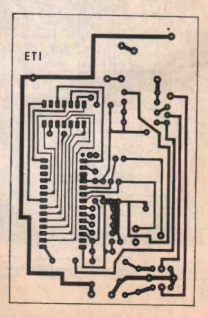
The Remote Control Transmitter PCB.
