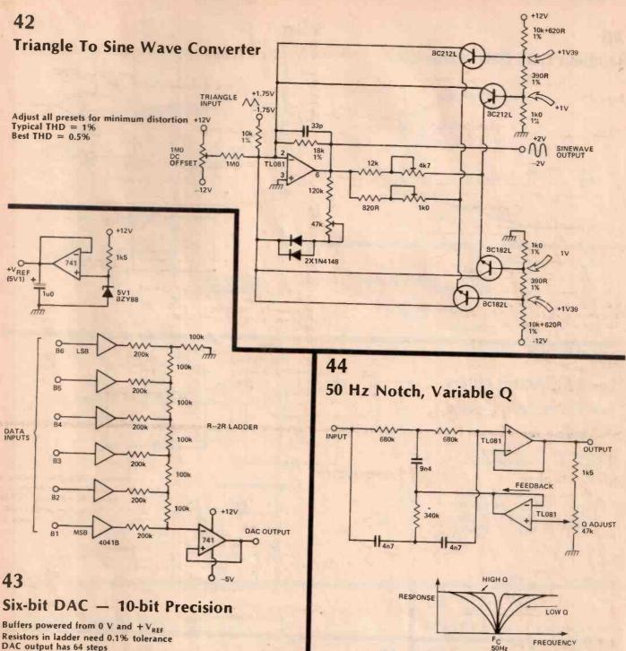
Resistors in ladder need 0.1% tolerance DAC output has 64 steps
