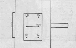
Fig. 1 Motor wiring diagram. Note that both the centre terminals are connected to 12 V.
