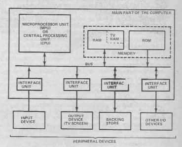
Fig. 1 Block diagram showing the hardware of a microcomputer.
