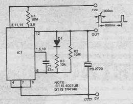
Fig. 11 This transducer-driving version of the Fig. 10 circuit acts as a ticktick generator or acoustic object-finder. It consumes 2 uA at 6 V, or 4.5 uA at 10 V.
