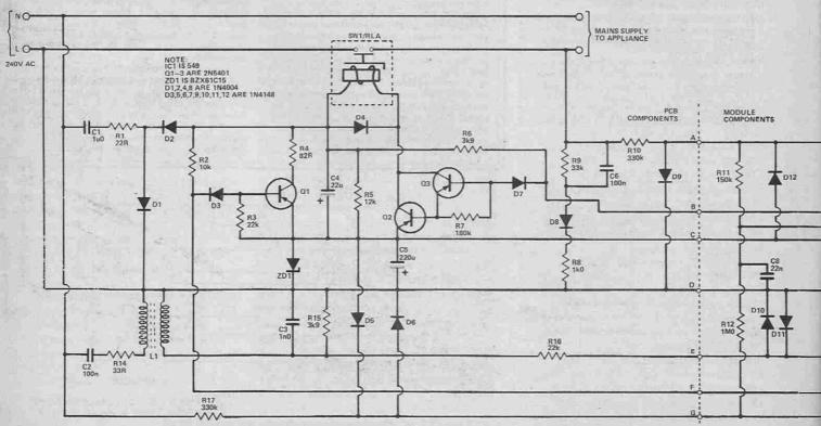
Fig. 4 Circuit diagram of the receiver. Components to the right of the dotted line are supplied ready-mounted on the appliance module. 58 ETI OCTOBER 1981
