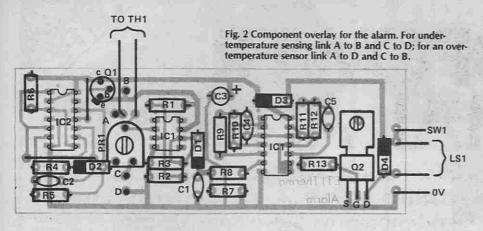
practical use, the thermistor is mounted remote from the PCB.
