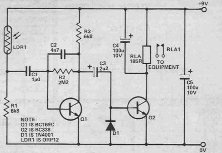
This gives a series of pulses across the relay coil, and these are integrated by C4 so that the relay is closed continuously, not pulsed on and off. A normally-open relay contact is used to control the external equipment (or a normally-closed type if it is necessary for the controlled equipment to switch on when the mains lighting is switched off). Avoid strong natural lighting on LDR1 as this will greatly reduce the sensitivity of the circuit
