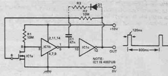
Fig. 10 This asymmetrical ring-of-three astable consumes 5 uA at 10 V, 2 uA at 6 V.
