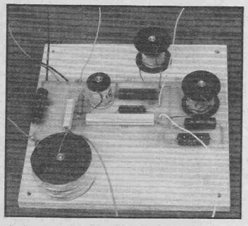
After the components have been soldered to the PCB, the crossover board is secured to a plywood panel using the choke fixing bolts. To get the choke connecting leads the right length, you'll have to cut access holes beneath the PCB pads so you can solder the wires last.
