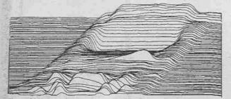
Fig. 2 This FRESP plot pinpoints regions which may benefit from a more detailed SCALP analysis. For example, the odd hump at about 500 Hz is probably worth investigating.
