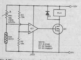
Fig. 1 This over-temperature alarm consumes a quiescent current of about 5 mA and will flatten a PP9 battery in under two days.
