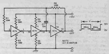
Fig. 9 This micropower ring-of-three symmetrical astable consumes 8 uA at 10 V, or 1.5 uA at 6 V.
