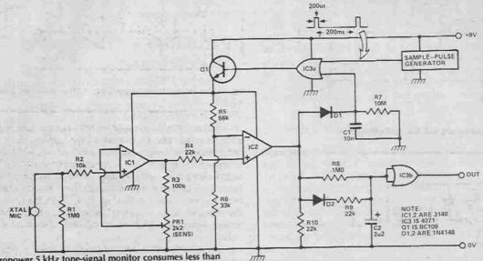
Fig. 3 This micropower 5 kHz tone-signal monitor consumes less than 10 uA of stand-by current.
