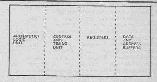
Fig. 2 The functional elements contained in the block marked Microprocessor Unit in Fig. 1.
