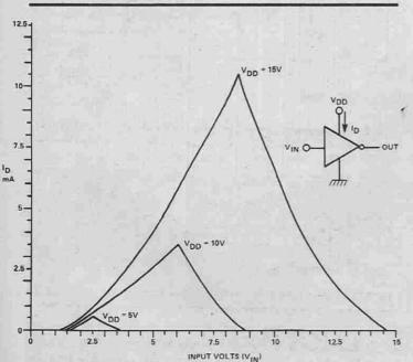
Fig. 7 This 'unbuffered' version of the ring-of-three astable consumes 280 uA at 6 V, 1.6 mA at 10 V.
