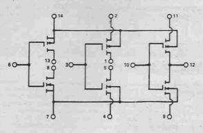
Fig. 6 Functional diagram of the 4007UB dual complementary pair and inverter.
