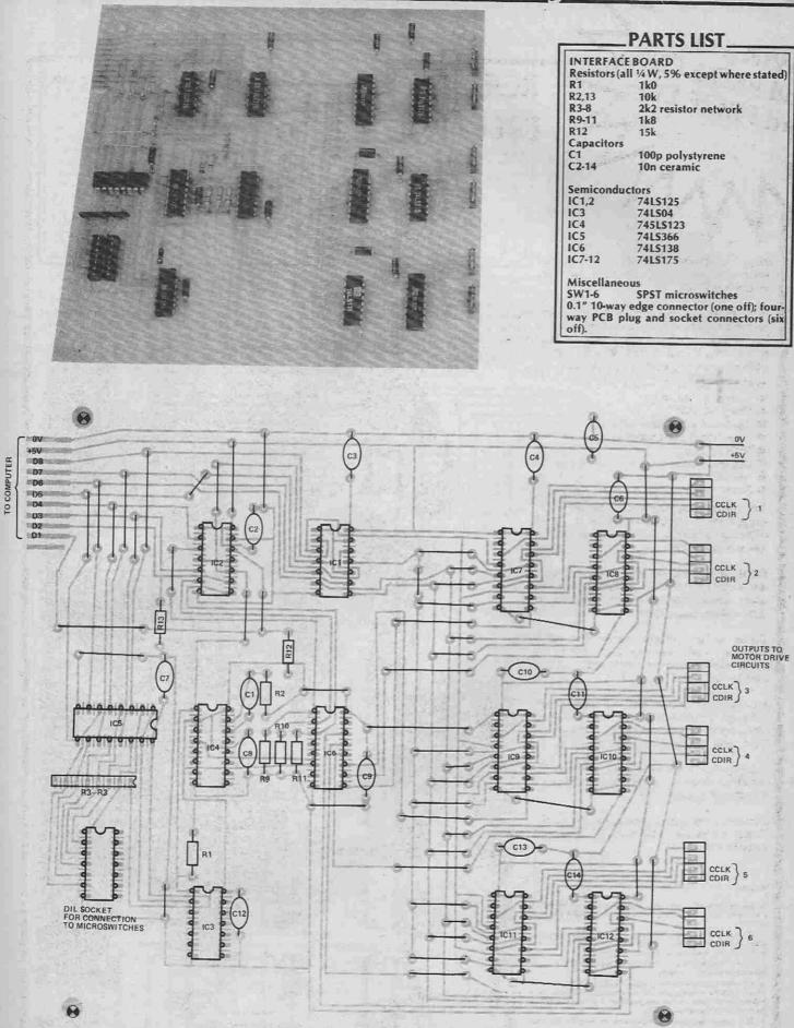
Fig. 3 Interface board overlay. The connection to the computer port will depend on your particular machine.
