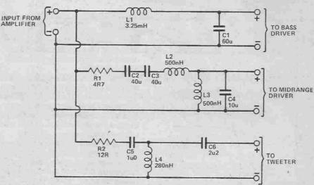
Fig. 6 Circuit diagram of the crossover.
