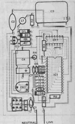
Fig. 6 Overlay for the transmitter board. Make links A,B,C,D as shown in Fig. 3.
