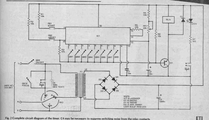
Fig. 2 Complete circuit diagram of the timer. C4 may be necessary to suppress switching noise from the relay contacts. ETI OCTOBER 1981
