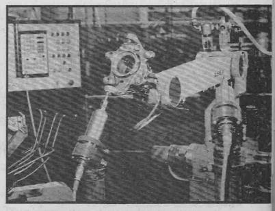
De-burring a guide-spindle housing after machining. The IRb-6 robot picks up the items and guides them against rotary files.
