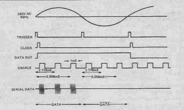
Fig. 2 The timing diagram for the transmitter signals.
