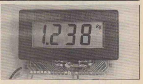
easily wound inductive displacement transducer and the associated drive electronics on a small PCB, all supplied from a 9 V battery. An analogue voltage proportional to weight is obtained, which is then displayed on a 3½ digit LCD panel meter module. Up to 2 kg can be displayed on the scales, but a zero-offset control allows a given weight to be re-zeroed. This provides the useful facility of weighing and mixing ingredients simultaneously – when preparing cake mixture, for example.
