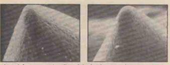
Above left: a conventionally polished stylus tip under extreme magnification. Above right: the V15V MASAR polish under the same power magnification. Note how much smoother the contact area appears. This could lead to lower surface noise and reduced record wear.
