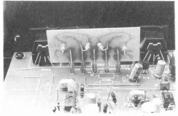
Above: the matching board for the pickup input in close-up. Note the nicely worked up edge connections. This particular board is for a Shure V15 IV pickup, I think. Trouble was I tried so many it is now impossible to remember which one was in when the camera went off!
