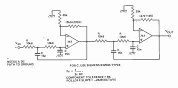
Fig.8c. Fourth order low pass filter, 1 kHz.
