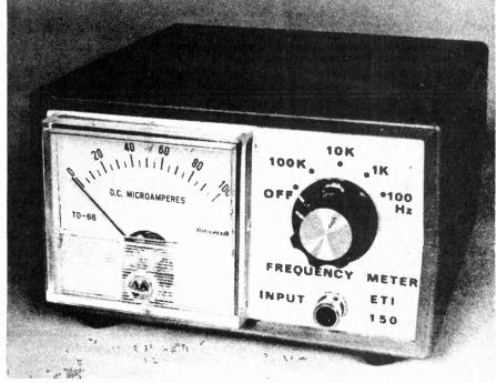
here are many applications in the home workshop where simple audio frequency measurements are required. When experimenting with oscillators, building or repairing function generators etc, it is often handy to have some means of measuring frequency accuracy tò the last Hertz is not always required and thus a full-blown digital counter is not warranted.
