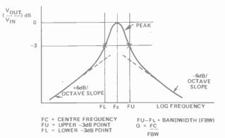
Fig.14. Band pass response (single pole).
