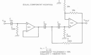
Fig.13b. Third order Butterworth 1 kHz high pass filter.
