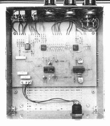
Fig.2. The voltage controlled state variable filter can be built into this Teko Alba case (see Buylines) as a 'stand alone' project.
