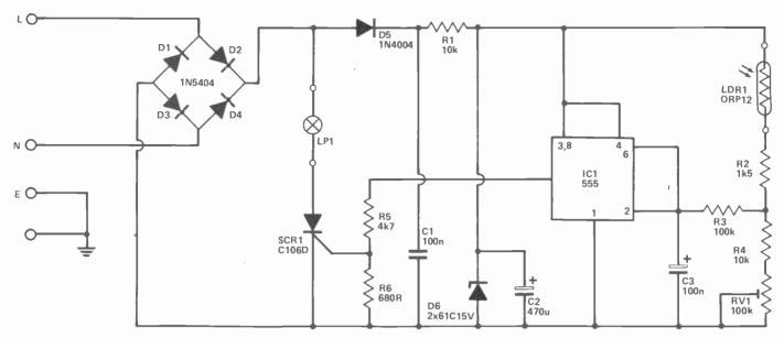
Fig.3. Circuit diagram. A common or garden 555 is at the heart of the unit.
