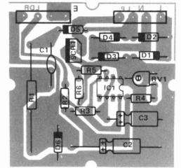
Fig.4. Component overlay. THERE IS MAINS AND RECTIFIED MAINS ON THIS BOARD.
