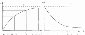
Fig.3 Plotting graphs of output voltage against multiples of time constant.
