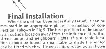
in Fig.2. This completes the construction of the unit. If the completed unit is mounted externally, some form of weather proof seal must be made between the box and the blanking plate. The best type of sealer to use is silicone bath sealer. Spread a small amount on the mating surfaces of the box and tighten down the plate. The sealer will harden and prevent water entering.
