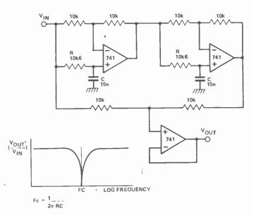
Fig.19. Notch filter using all pass sections.
