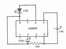
Fig.5. Fast 1V5 blinker. Flash rate is 2.6 Hz and drain current is 1.2 mA.
