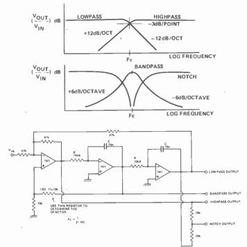
Fig.17. State variable filter.
