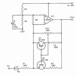
increases due to the shunting effect of R2 and R3.
