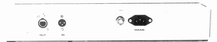
The simple layout of the rear panel -- mains in, signal in, signal out.
