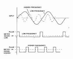
Above: waveform diagrams which indicate two possible sources of incorrect reading using a DFM. The drawings are selfexplanatory on the whole.
