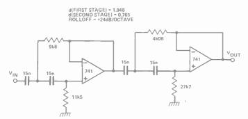
Fig.12c. Fourth order Butterworth 1 kHz high pass filter.
