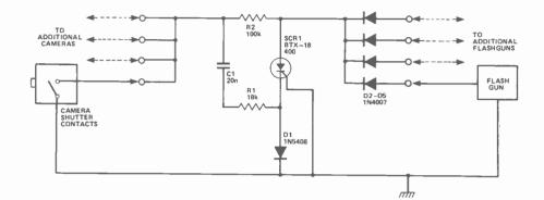
When one or more flashguns are connected to the unit, the cathodes of D2-D5 rise to a high positive value, say +200 V.
