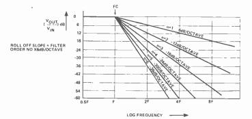
Fig.2. Filter roll-off slopes. As n increases so does the roll-off.
