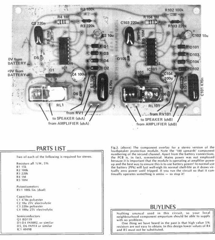
When the power to the loudspeakers exceeds that set by the potentiometer the protector should trip in and disconnect the loudspeakers.
