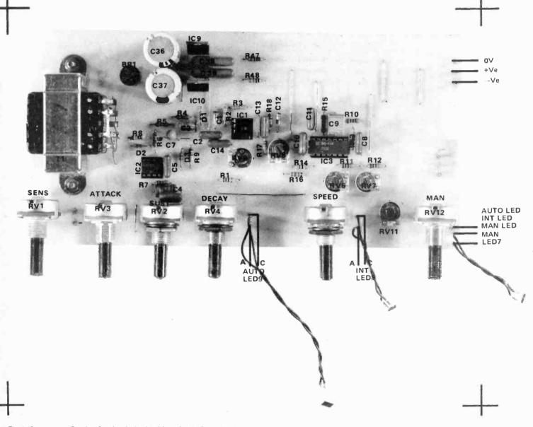
Fig.4. Component Overlay for the single sided board, which carries the power supply.
