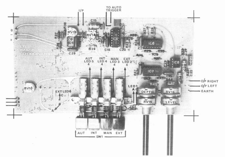
Fig.5. Component Overlay of the double sided board.
