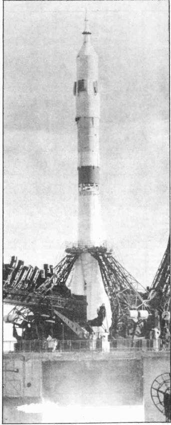
The Russian end of the Apollo/Soyuz Test Project – Soyuz, still clamped down to the launch pad.
