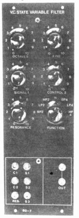
If you wish to build all of the Project 80 modules and install them in a single case with keyboard, mount the PCB on this front panel. At the end of the series you'll have a matching set.
