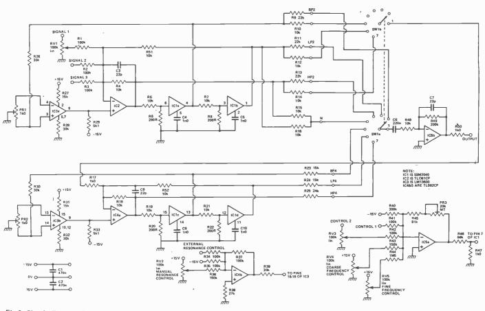
Fig.2. Circuit diagram of the state variable filter.
