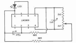
Fig.6. Variable rate flasher. The rate is variable from zero to 20 Hz.
