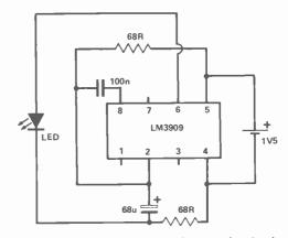
Fig.7. High efficiency 'continuous' 1V5 LED indicator. The circuit provides a steady but dim illumination by pulsing the LED at 2 kHz. Drain current is 4 mA.
