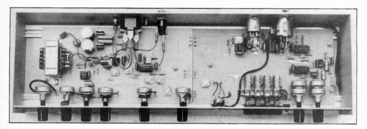
Construction should pose no problems. The two PCBs hold almost all of the components and controls.
