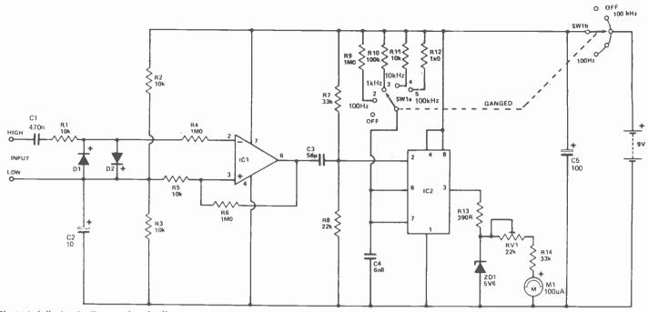
Fig.1. A full circuit diagram for the linear frequency meter.
