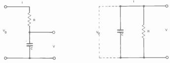
Fig.1 Series and parallel RC networks.
