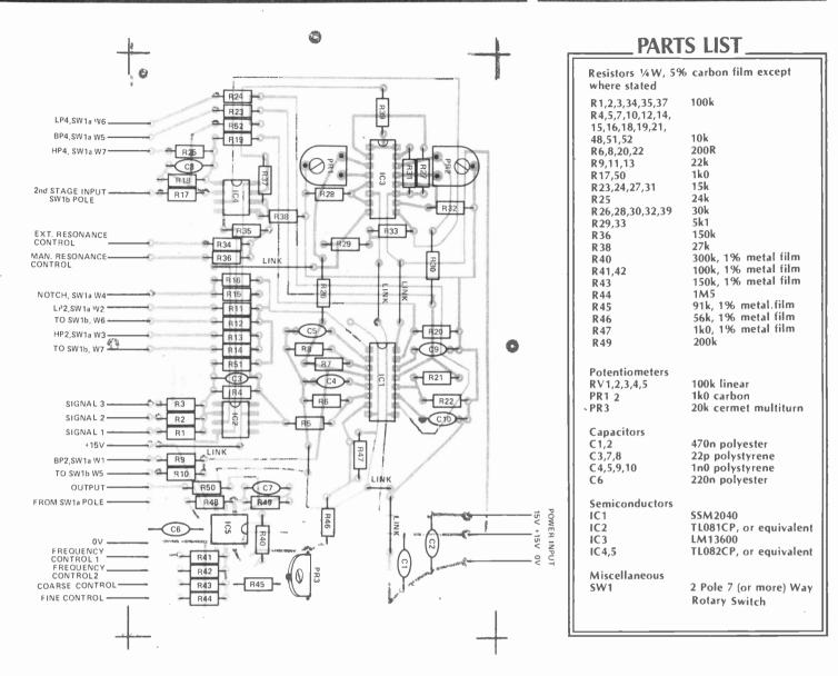
should be left at the setting where the low pass output commences. The selector switch can then be turned through its seven outputs to check that the appropriate response is present and these can be clearly identified by ear. If an oscilloscope is available then switching to BP2, LP4 and HP4 outputs and making minor adjustments to both PR1 and PR2 may result in some improvement to the filter responses.
