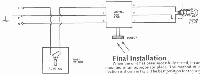
Fig.5. Method of connection of the unit to the house mains wiring.
