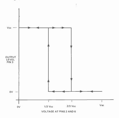
Fig.1. IC1 is used as a level dectector with hysteresis.
