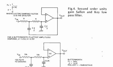
Fig.5a. Second order low pass filter, 1 kHz.
