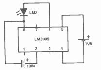
Fig.3. Minimum power 1V5 flasher. Nominal flash rate is 1.1 Hz and average drain current is 0.32 mA.
