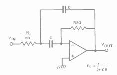
Fig.15. Single pole multiple feedback bank pass filter.
