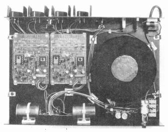
Above: the 204 power amp revealed. Note the huge toroidal mains transformer and pre-amp PSU board away to the left. Separate heatsinks are used for each power output device.
