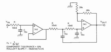
Fig.8b. Third order low pass filter, 1 kHz.
