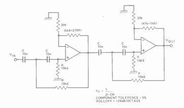
Fig.13c. Fourth order Butterworth 1 kHz high pass filter.
