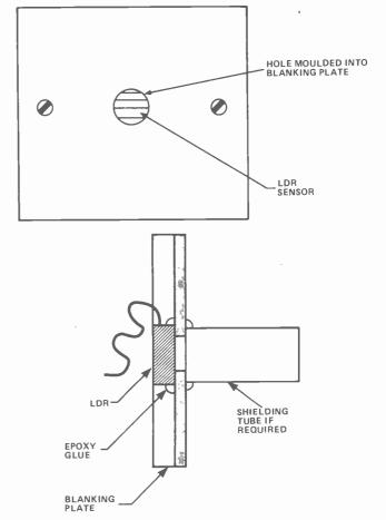
Fig.2. The LDR is mounted in the blanking plate (top). A shielding tube may be fitted if necessary (above).
