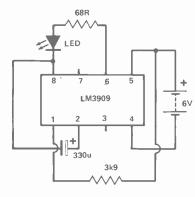
Fig.9. This 6 V flasher operates at about 1 Hz.
