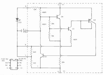
Fig.1. The internal circuit and practical connections of the LM3909 low voltage LED flasher/oscillator IC. The IC outline is also shown.
