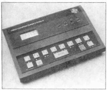
Above: the Chess Champion master unit with its clock-type display. To the right is shown the bus connection for the slave printer-board units.
