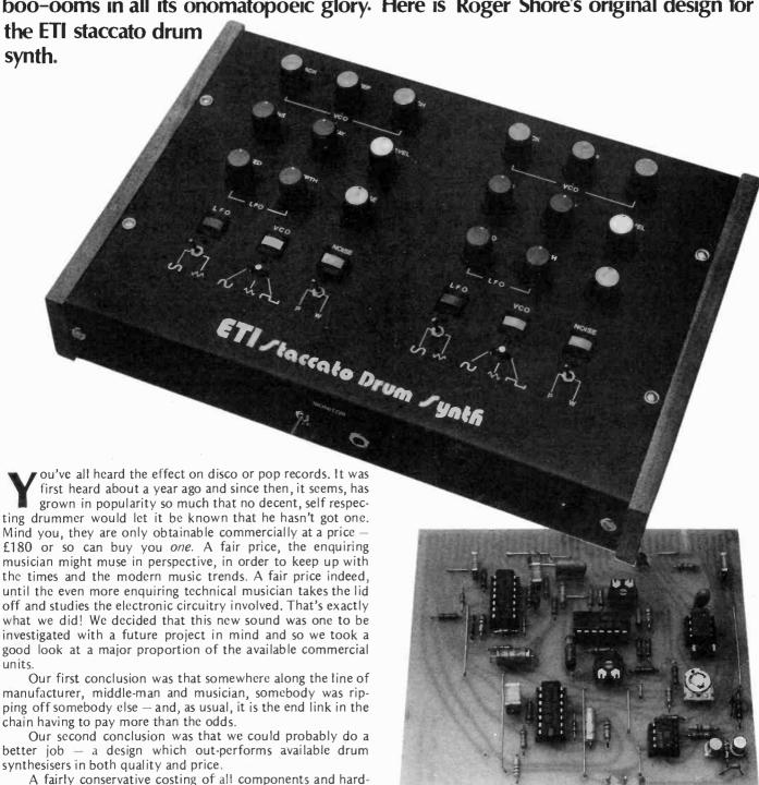
All 42 ways of the control board (above) are used. Cut a slot at pin 37 for identification.
