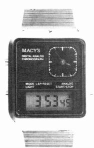
The above watch is a new style digital analogue featuring complete up-to-date modern technology. The watch basically constitutes a traditional hand watch plus a modern digital watch, both battery powered.
