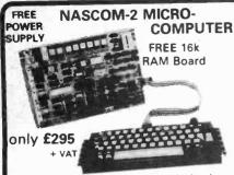
Z80A 8 bit. This will run at 4 Mhz but is selected between 1/2/4/Mhz On-board, addressable memory. 2K 2K Monitor - Nas-sys 1. 1K Video RAM (MK 4118). 1K work space/User RAM (MK 4118), 8K Microsoft Basic (MK 3600 ROM). 8K Static RAM/2708E Pr.
