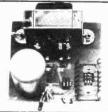
Need a one amp power supply at five valts or twelve volts? Fed up with lash ups? Here is a basic 'na frills' 1 amp P.S.U. kit, based on the well known uor800 series three terminal regulators. When assembled, all components, including the transformes are mounted on the printed circuit board. Use the module as a bench power supply, or as part of a piece of equipment.
