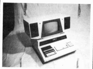
The U.K. designed and manufactured Novapac disk system for Commodore's PET\*, first seen at Compec '78, is (after extensive industrial evaluation), now available to the domestic user. Its unique saddle configuration continues the integrated design concept of your PET, with no trailing wires or bulky desktop modules.
