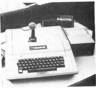
The familiar Apple II with a speech recognition board installed. It worked remarkably well and 'echoed' back your word through a synthesizer.
