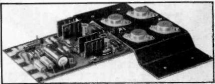
Designated the AL250, a new 125W rms amplifier rose to our notice recently from Bi-Pak Semiconductors, 63a High Street, Ware, Herts. Retailing at under £16 the amplifier has a very good specification, (see below) that would suit it perfectly for use as a guitar amplifier, assuming a suitable pre-amp.
