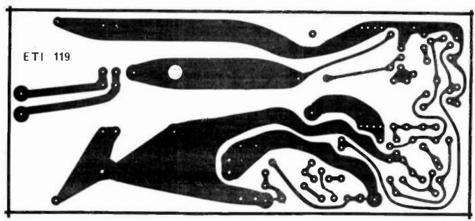
Fig. 4. Printed circuit-board layout. Full size. 178 x 78 mm.
