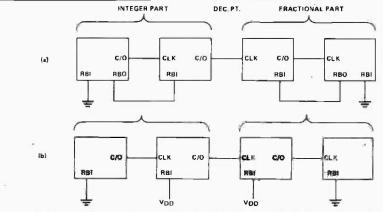
Fig. 16. Four digit counters using the 4033A with non-significant zero supression (a) in all positions (b) in first and last position only.
