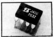
J406 offer a high performance for Op Amp front ends. The J401 features CMRR >95dB; offset 5mV (max) and drift  $10\mu$ V/OC (max): Details from Siliconix Ltd, 30A High Street, Thatcham, Newbury, Berks RG13 4JG.
