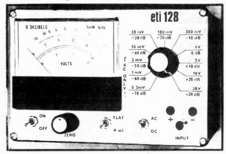
The meter used in the prototype measured 100 x B2mm but required to be rescaled. Any similar meter may be used as long as it has 100 microamp sensitivity.
