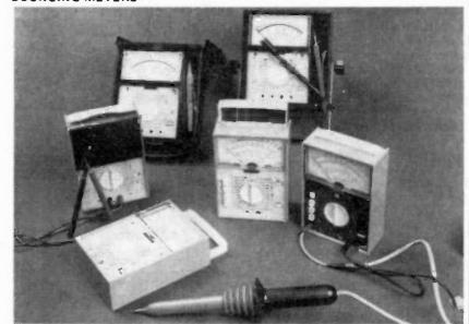
Western Instruments have released a new VOM series, one major feature of which is their 'invunerability'. All five models in the 660 series are drop-proof and feature a custom rugged self-shielded taut-band mechanism, diode-protected meter movement, temperature compensation, pluggable circuit board assemblies,
