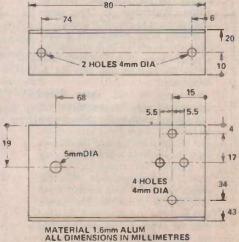
ALL DIMENSIONS IN MILLIMETRE Fig. 2, Transistor/diode mounting bracket.
