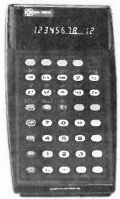
rechargeable cassette. The machine uses algebraic logic and is fully guaranteed for 1 year. A 12-digit green display gives 8-digit mantissa and 2-digit exponent plus signs. The functions of the calculator are:
