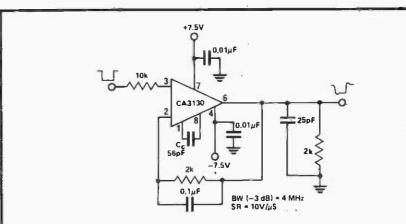
Fig. 4. Voltage follower circuit with split supply of plus and minus 7.5 volts. This circuit allows low impedance loads to be driven from a high impedance source.
