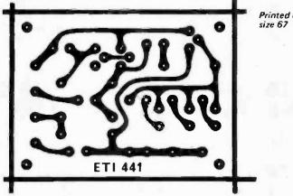
Printed circuit layout, Full size 67 x 49 mm.
