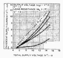
Fig. 2. Supply current against total supply voltage.
