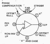
Fig. 1. Functional diagram of the CA3130.
