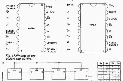
Fig. 18. Circuit diagram and counting sequence for a four stage Johnson or "twisted ring" counter.
