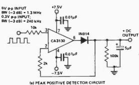
Fig. 5. Peak positive detector circuit. Detectors such as this are ideal for building accurate ac voltmeters.
