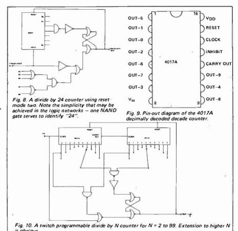
7. The circuit dissipation of both the counters would be very low (less than 1mW) at this low operating frequency and the only note of caution to be sounded is that the counter and flip-flop should not both be triggered from the same edge of the clock pulse (i.e. one should be positive and the other negative edge-triggered).
