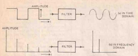
Fig. 1(a). A filter alters the frequency content of a signal. This means the wave shape is changed when displayed as an amplitude-time graph. (b). Using the frequency spectrum form of display the filter removes (or enhances) certain frequencies.
