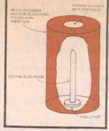
Fig. 3. Basic arrangement of ionisation kinds of radioactivity sensors - the G-M tube, ionisation and proportional detectors.
