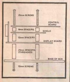
ig. 8. The best way to assemble the counter ind display boards.
