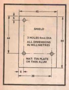
Fig. 7. Drilling details of the shield plate.
