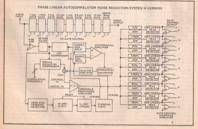
push-pull control voltage for each bandpass region. These control signals control associated notch filters in the programme signal path.
