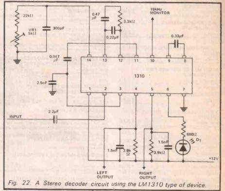
signal from the device has a frequency of 19kHz. (The amplitude of the signal is about 3V peak).
