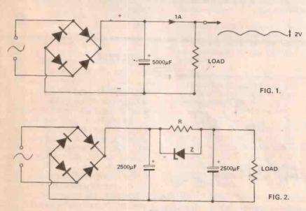
In the normal circuit (Fig. 1) the ripple at 1 amp is at least 2 volts. Cheap power amps use this circuit (with low supply ripple rejection) and produce annoying amounts of hum at low signal levels.
