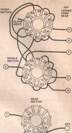
Fig. 3. Wiring of the range switch.
