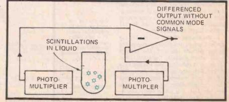
Fig. 6. Differential detection provides common-mode signal rejection in the liquid scintillation spectrometer.
