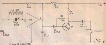
Fig. 1. Circuit of the miniature receiver.
