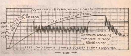
The graph compares a controlled temperature tool with a conventional tool. Note that the heat up time is only a fraction of that required for the fixed temperature tool, which also cools down progressively under identical load conditions.
