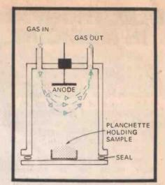
Fig. 7. In the gas flow detector gamma and beta radiation is monitored without the attenuation of windows.
