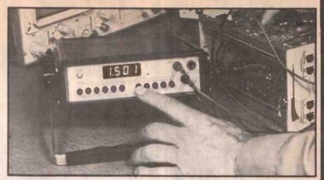
A new 3½ digit, 5-function digital multimeter from Gould Advance, the DMM7, is aimed at the general-purpose medium-accuracy market. It features very high stability and accuracy, and includes an automatic zeroing feature to eliminate offset errors. Polarity and decimal points are automatically displayed, and overrange is indicated by the display flashing. The DMM7 uses p-MOS LSI for both analogue and digital functions, and is housed in a metal case measuring 63 x 272 x 216 mm.
