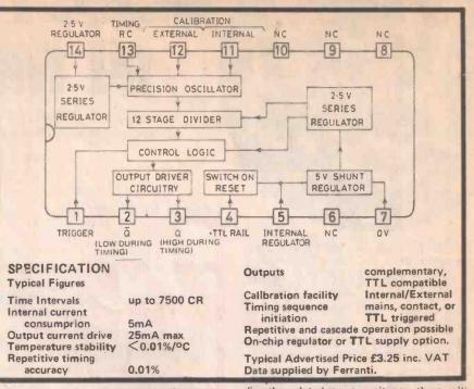
between the timing C and R. Adjustment to the time period is then carried out by inspection of the oscillator frequency at 13 (T=4095 x oscillator frequency).
