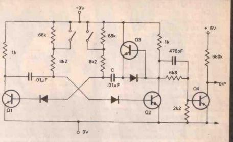
output is used for driving TTL the collector load must be returned to a voltage no greater than +5V.
