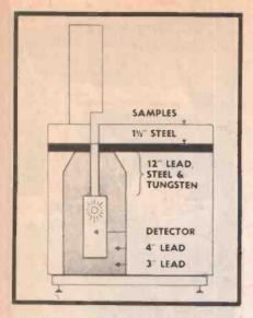
Fig. 5. The use of shielding is vital to obtain Correct measurements in the gamma Counting system.
