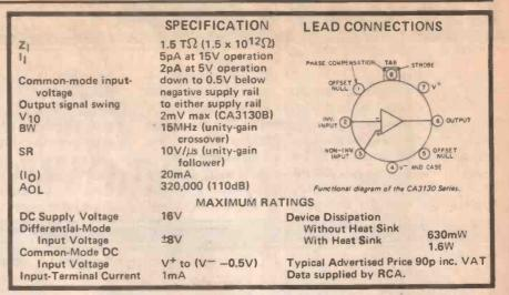
provide the total gain of the CA3130. Care should be taken in handling the CA3130 - see "Handling CMOS' in ETI November 1974.
