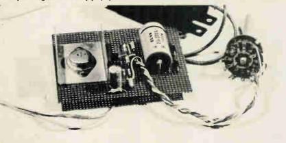
The power supply shown unmounted. Note the aluminium heat sink for the power transistor.
