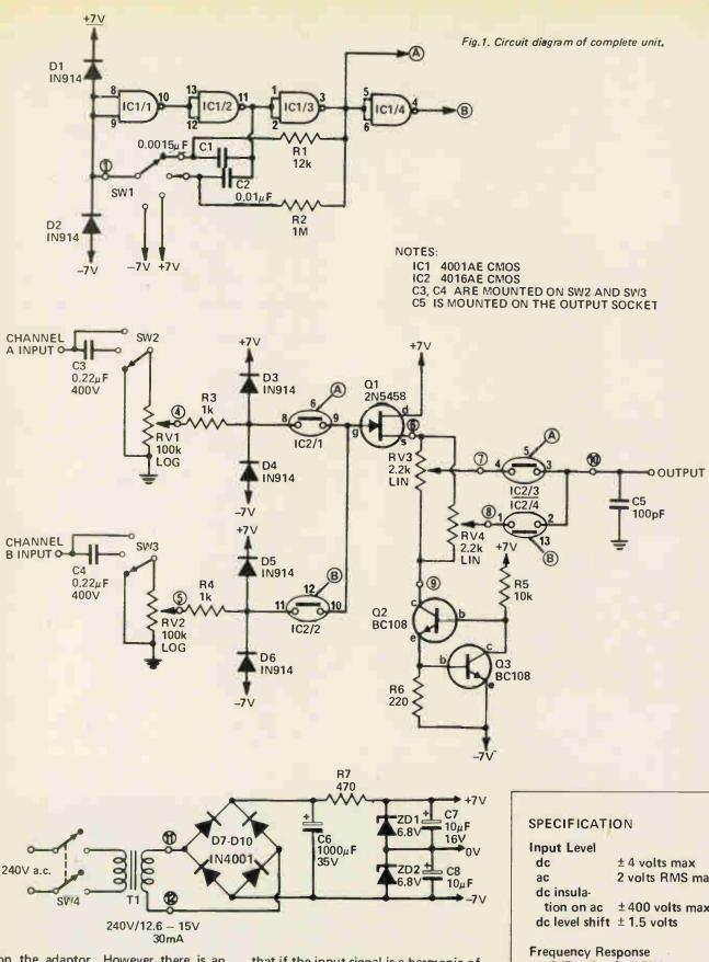
on the adaptor. However there is an attenuator provided on each input so that some adjustment may be made.
