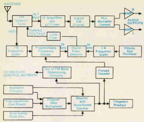
Block diagram (preating a mplified) of the circuit.
