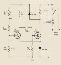
A negative temperature coefficient (NTC) resistor is used to sense temperature. Transistors Q1 and Q2 form a Schmitt trigger which switches when the voltage at the base of Q1 increases above 1.4 volts. Thus when the temperature falls below that set by RV1 the Schmitt changes state and the relay opens switching the heater 'ON'. Regulation accuracy is 1° to 2°C.
