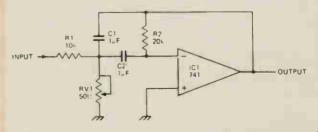
This active filter has a gain of unity (0 dB) and is useful over the range 0.01 Hz to 3 kHz. The centre frequency of the passband is set by potentiometer RV1 and the bandwidth is determined by the values of R1, C1 and C2. The values shown in the circuit provide a bandwidth of about 15 Hz. With RV1 set to mid-position the centre frequency is approximately 220 Hz.
