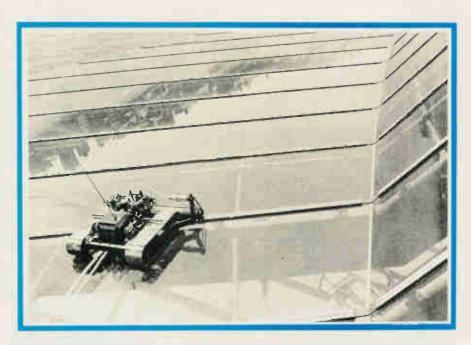
The tractor is driven by compressed air motors controlled by pneumatic air valves via the radio link. A further air motor drives the cleaning roller — mounted on the front of the device.
