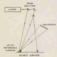
Fig.8. Local reference beam for object
