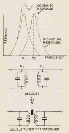
Fig. 15. (a) Two tuned circuits may be used to obtain a better bandwidth/ selectivity compromise. (b) The two separate-tuned circuits may be combined into a single transformer. This construction is used extensively in radio receivers.
