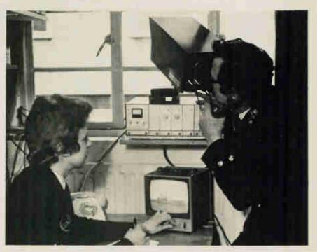
The picture shows the setting up of an audio-video linkage between buildings at HMS Mercury, the navy's signal school near Petersfield. This new opto-electronic linkage transmits across obstacles such as roads, railways and waterways using modulated infrared radiation (900 nanometers). It carries picture and sound with a duplex telephone service channel.
