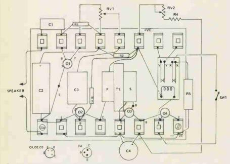
Fig. 2. The tag-board wiring.
