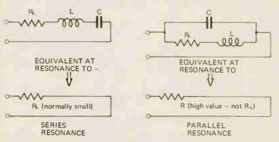
Fig.12. At resonance the two types of tuned circuit become purely resistive. The series circuit becomes a very small resistance and the parallel circuit becomes a very high resistance.
