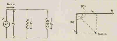
Fig.1. (a) The parallel resistor and inductor. (b). Vector diagram of circuit in Fig. 1 a.
