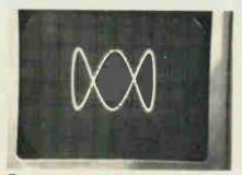
Three to one Lissajous pattern using the X·Y mode inputs and display. The 0.8cm/ division graticule can be seen in this photo.
