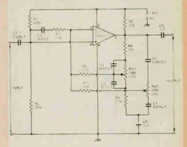
The input signal is applied to the non-inverting input of the IC which is a Siemens TAA861 operational amplifier. Bass and treble boost and cut are controlled by the potentiometers RV1 and RV2 respectively.
