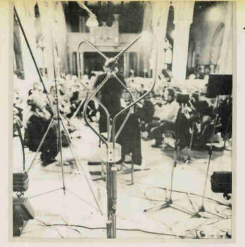
Here the tetrahedral microphone array used for ambisonic recording is used to capture the direct and reverberant sound field in St. Giles' Church, in the city of London.
