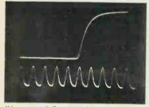
(Upper trace). Step waveform at approximately 0.3µS. (Lower trace). Waveform at 10MHz.
