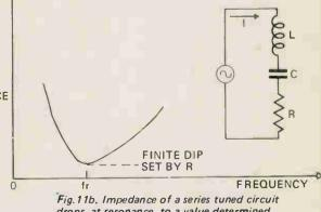
drops, at resonance, to a value determined by the dynamic resistance.
