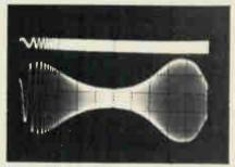
(Upper trace). Output from an audio frequency sweep generator L to R, 10 to 100Hz 0.1dB. (lower trace) Output from amplifier under test with bass and treble controls at maximum.
