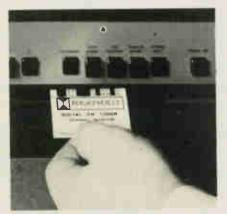
Inserting one of preprogrammed cards into its holder. This one represents 97.3MHz.
