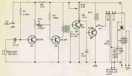
Fig. 1. Complete circuit of the Hear-and-Tell.
