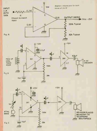
The LM381N dual op-amp has appeared several times in its usual guise as a low noise stereo audio preamplifier device. Indeed, it requires the very barest minimum of external components, since the function of the feedback resistors and capacitors is simply to determine the audio frequency response and gain.
