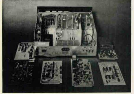
Rear view of the tuner with six of the circuit boards removed.
