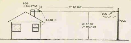
This simple antenna is suitable for the crystal radio and may be used for the one transistor radio if required.
