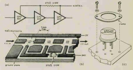
This wideband r.f. amplifier will provide a gain (within 2dB) of 35dB from 5 to 400MHz. The noise figure will be about 4.7dB and the power output (into  $50\Omega$ ) will be +14dBm.
