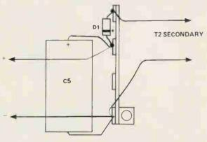
Fig. 3. Connection of the power supply components.
