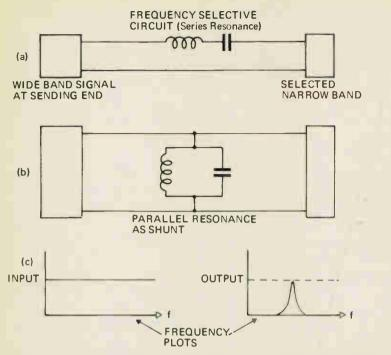
Fig.13. How coupling black boxes with tuned circuits provides frequency selection. (a) coupling by series tuned circuit. (b) coupling by parallel tuned circuit. (c) the input versus frequency compared to the output versus frequency.
