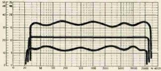
Graph shows degree of control throughout frequency range with Sound Effect Controllers in maximum and minimum positions.
