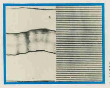
Fig. 1. Photomicrograph compares grooves of (left) standard long-play audio record, and, (right) Teldec video disc. of groove space. The grooves terminate some 5 cm from the centre.
