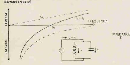
Fig 9b. Currents in the parallel tuned circuit as the frequency is varied.
