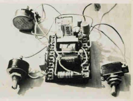
The tag-board, switches and controls.
