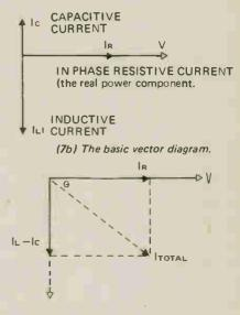
(7c) The vector solution – the reactive components having been subtracted.
