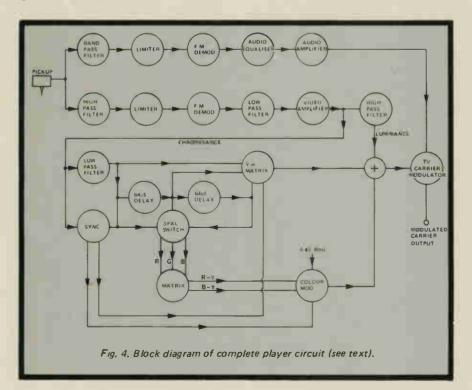
1 MHz carrier, and the audio response extends up to 15 kHz. The sound carrier amplitude is -30 dB compared with that of the vision signal, yet a signal-to-noise ratio of -50 dB is maintained.
