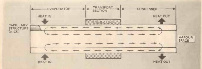
Fig. 14 Schematic of a two-phase heat pipe.
