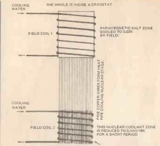
ASSES) Fig. 4. Arrangement used in magnetic cooling. The salt and gas-surround are allowed to cool to liquid helium temperature. Magnetic field is applied aligning the electron spins. The gas is evacuated to remove excess heat. The field is then removed. ENDS TURNED OVER AND OVER TO IMPROVE HEAT TRANSFER.
