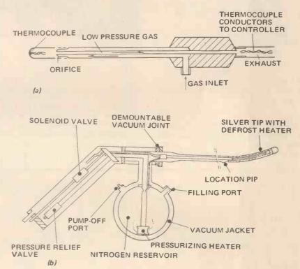
Fig. 13 Cryosurgical instruments by Spembly Products: (a) Neurological probe having a small active volume. (b) Urological probe for the removal of tumours.
