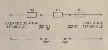
Fig. 8. Circuit used in a Zener barrier.
