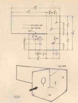
Fig. 2. Construction of the sub-chassis. Any solerable sheet can be used (even a tin canl)
