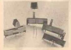
A dual wiper system on the carbon tracks gives good electrical contact and low noise operation. Mounting for these 45mm slider potentiometer can be via threaded fixing holes in metal case or by the P.C. solder tags.
