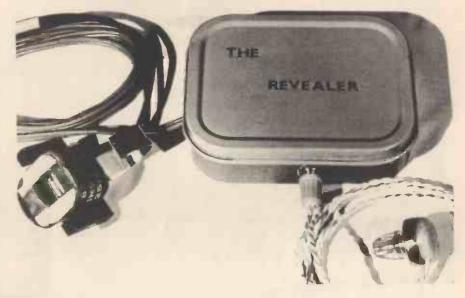
Fig 1. The completed unit together with earpiece and search coil.
