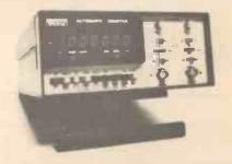
The new 2600 series of frequency counter timers are built on a basic unit with one 50MHz module allowing direct frequency and multiple period measurements with 30mV sensitivity. With the addition of a further 50M11z module time interval measurements can be taken with 100nS resolution. The third variation uses a 50MHz module plus a 520MHz module to give high frequency measurement with 50mV sensitivity.
