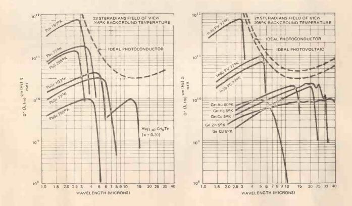
Fig. 10. Sensitivity of infrared detectors depends upon the temperature of the element as shown by these curves
