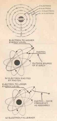
Fig. 3. (a) Simplified diagram (not typical of any particular element) of orbital levels of an atom. These levels are known as shells and are the only possible orbits.
