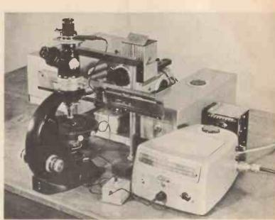
Fig. 3. EEL apparatus for measuring the reflectivity of ore minerals (using microphotometry).
