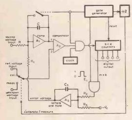
Fig. 1. Block diagram of A-to-D converter
