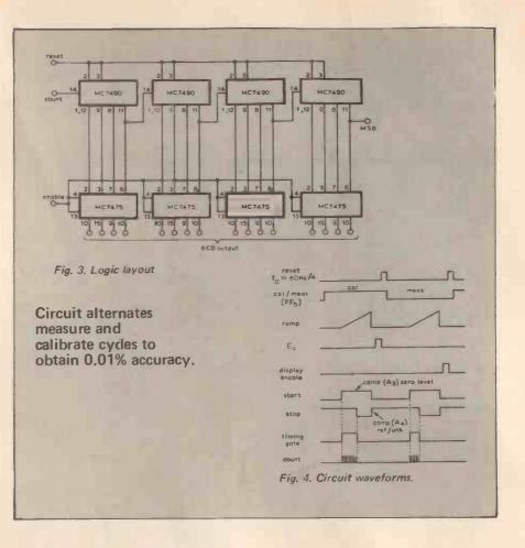
shallow slope, no more than 10 000 clock pulses can reach the counter during the calibrate cycle before the ramp reaches the eight volt reference. The error signal will hence always be of the correct polarity to drive the ramp up until the proper 8000 pulses are reached when the ramp crosses the eight volt reference, at which point the loop locks.
