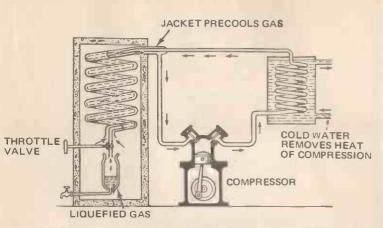
Fig. 2. Liquefaction obtained by the cooling of the release of pressure in the Linde-Hampson process is based on a principle devised by Joule and Thomson. They used a wad of silk instead of the modern expansion valve shown.
