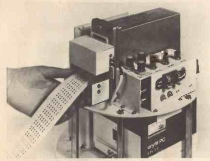
The output is printed in real values upon a paper tape which is stored within the instrument. Each pair of readings represents the Dissolved Oxygen and Temperature in the water at sampling rates which are variable from 1 minute to 2 hours.
