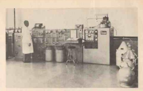
Fig. 6. Helium liquefier plant. Helium is recovered from experiments. Note the dewars on the right.
