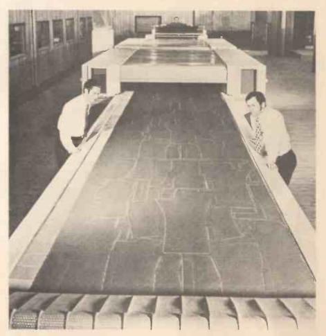
Cloth being cut at high speed to complex patterns by a computer controlled laser beam.
