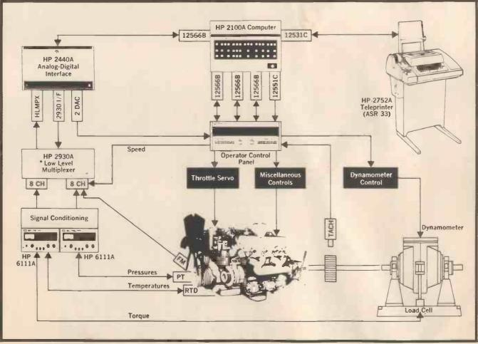
Fig. 7. HP9600 data acquisition and control system applied to engine testing.
