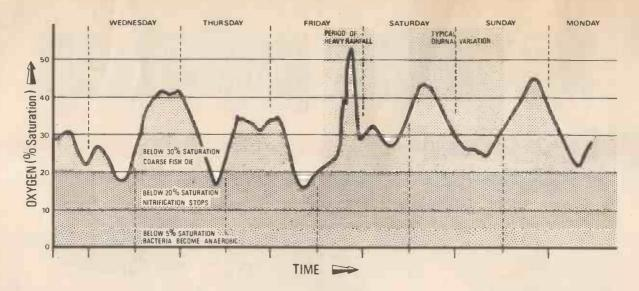
Analogue plot of digital recordings on paper tape of dissolved oxygen level during a six-day period in a small river containing a high proportion of treated sewage. This graph contains the data obtained from 500 discrete samples. The Model 8050 clearly shows that there are periods when the sewage load is more than either the sewage plant or the river itself can purify. There is an obvious difference between the amount of pollution during the week and that at the weekend.
