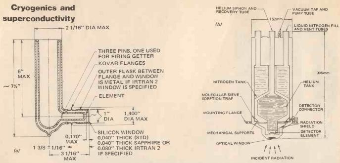
Fig. 11. Dewars used to cool infrared detectors: (a) A style 60A glass dewar (b) Cross section of a Mullard stainless steel unit using helium
