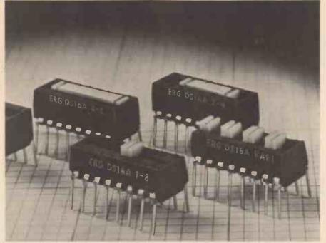
Erg Dilswitches. These high quality miniature switches are made to fit into standard DIL sockets, PCBs and Veroboard. They are rated as: Maximum voltage 28V d.c. at 250mA; Life (minimum) 20,000 contact wipes. They are available in the following types: DIL 1-8, 1-pole 8-way at 75p; DIL 2-4 2-pole 4-way at 80p; DIL 4-2 4-pole 2-way at 85p; DILVARI 4 times 1-pole 2-way at 90p; DILI-6 1-pole 6-way (To Order).
