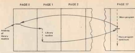
Fig. 3 Illustrates how access is gained to library routines from the main program – a method employed in a number of popular small machines
