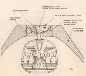
Fig. 17 Superconducting suspension arrangements of proposed maglev vehicles. (a) A highspeed rocket at 5000 m/s. (b) The Stanford concept for a 600 km/hr train. (c) University of Warwick proposal.
