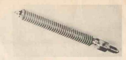
Fig. 12b A Joule-Thomson cryostat head. Cooling is by pressure release of argon or nitrogen gas.
