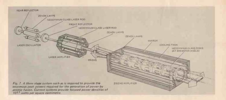
base material in rod form containing up to 2% of another impurity material which produces the laser action.
