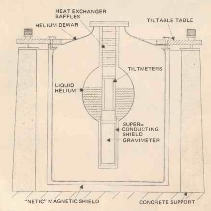
Fig. 18 Cross-section of a superconducting gravity meter installation. The tilt meters are used to correct records for inclination
