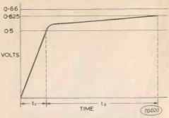
Fig. 5 Charging characteristic, time plotted against voltage. Linear portion up to 0.5V is used for timing and similar applications, for storage purposes 10 times more energy can be stored if the voltage is taken up to 0.625V, due to longer charging time above 0.5V.
