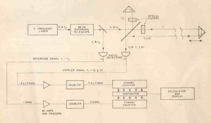
An important application of helium-neon lasers is in distance and velocity measurements by interferometric techniques. This system, the Hewlett Packard model 5525A is capable measuring length with an accuracy of  $\pm 0.000\ 001$  inch over 200 feet.
