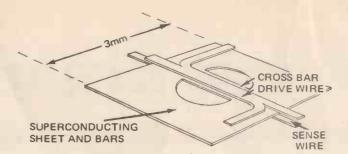
Fig. 19 The Crowe superconducting memory cell. The main disc is lead and all elements are superconductors.
