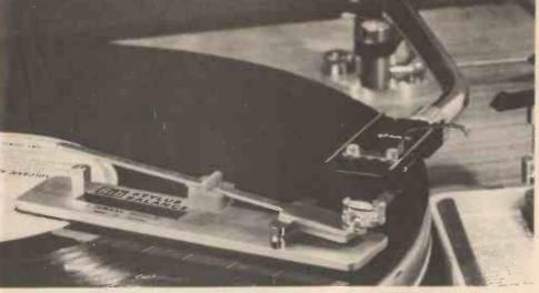
Tracking weight may be set very accurately using a stylus balance.
