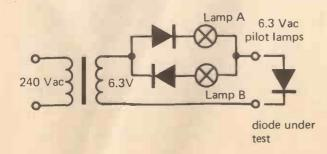
If lamp A or lamp B is illuminated the diode is serviceable. If both light the diode is short circuit. If neither light, diode is open circuit.
