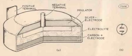
Fig. 1 (a) Cross-section showing construction of the Solid Electrolyte Device. (b) Circuit symbol
