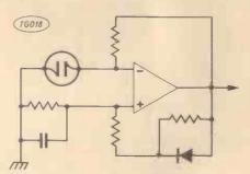
Fig. 3. Circuit of multivibrator for long timing cycles using the device with an operational IC amplifier.
