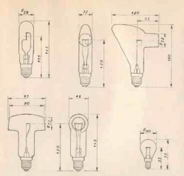
Fig. 2. Tungsten ribbon lamps especially designed to produce a uniformly radiating surface. The windows are ground plane-parallel from quartz or heat-resisting glass and must have their spectral energy transmission calibrated before manufacture.
