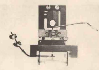
Fig. 20 (a) This niobium point contact is used to determine emf by the ac Josephson method (b) Voltage-current signal at 1m V levels
