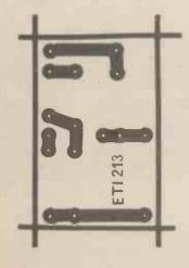
Fig. 5. A printed circuit board may be used (foil pattern shown here full size), or the unit may be assembled on tag strips or Veroboard.
