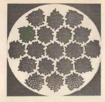
Fig. 15 Cross section of Imperial Metals Industries superconducting cable. It has 1045 filaments held in a copper matrix.
