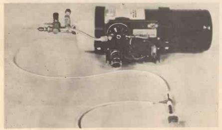
Fig. 12a Liquid nitrogen transfer system. The standby time is 60 hr enabling a detector to be used virtually on demand.
