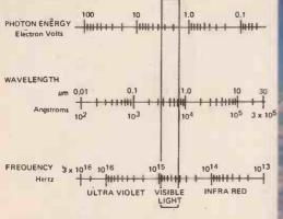
Fig. 1. Comparison of units used for electromagnetic radiation at optical frequencies. For example an energy change of 10 electron volts (ie  $V = 10^{-19}$  joules) produces radiation at 0.1 µmetres or 1000 angstrom, which is equivalent to a frequency of 2 x 10<sup>15</sup> Hertz. Another SI preferred unit of wavelength is the nanometre = 1000 micrometres.
