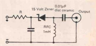
Zener diodes generate substantial amounts of internal noise. The level of this is typically 30 dB above thermal noise at frequencies up to 150 MHz.
