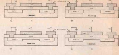
Fig. 6. (A) N-channel MOSFET in the "OFF" condition. (B) channel MOSFET in the "OFF" condition. (C) N-channel MOSFET in the "ON" condition. (D) P-channel MOSFET in the "ON" condition.
