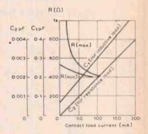
Experience has shown that contact failure is often due to transient overloads of which the designer may be unaware. It is good engineering practice to connect a series CR network across the contacts to prolong contact life as shown in Figure 1 (a). Such a network will protect the contacts against damage which may otherwise occur when the current through resistive or inductive loads is interrupted. Figure 1 (b) gives the values of both C and R for various currents and loads.
