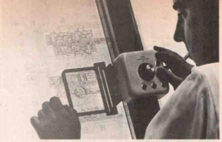
Layout of CMOS process masks is considerably enhanced by this coordinate digitizer machine, It is a convenient, efficient method for converting the designer's signal routing plan into data that a computer can understand and follow.
