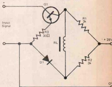
Accurate relay trip-point operation can be obtained over an ambient temperature range from -50°C to +90°C using this simple circuit.
