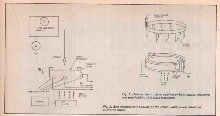
specimens were placed horizontally over a hot plate and surrounded by heat insulating bricks. The Irtran specimen was heated and then maintained at a constant 270°F. When the probe was energized — at 25 kV — the temperature of the speciment was reduced to 130°F.
