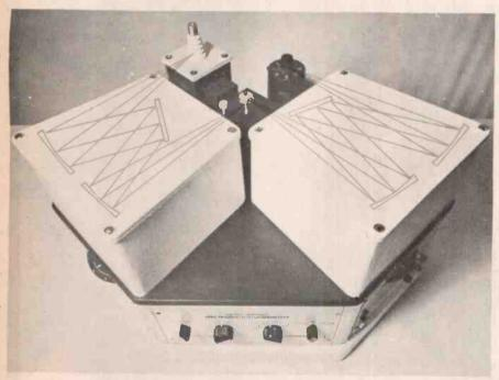
Fig. 7. The Aminco-Bowman spectrophotofluorometer. Lines superimposed show the optical paths of the excitation grating monochromator (on the left) that illuminates the sample placed in the centre and the emission dispersing grating monochromator (on the right) that is used to analyse the spectrum of the luminescence. The source is a Xenon lamp and the detector, a photo-multiplier of appropriate wavelength sensitivity.
