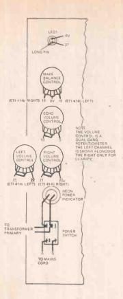
Fig. 7. Wiring to rear of main control panel.
