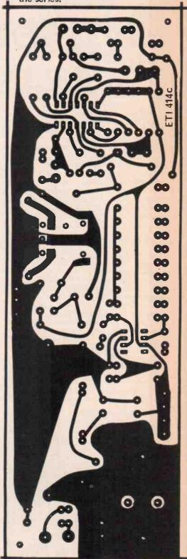
Fig. 2. Foil pattern for power supply board
