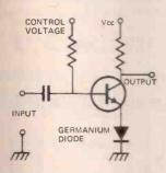
In this circuit a germanium diode is used to effect gain control of a common-emitter amplifier.
