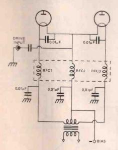
High power linear amplifiers using twin valves in the grounded grid configuration are quite commonly used.
