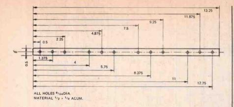
Fig. 13. Slide potentiometer support bars (two required)
