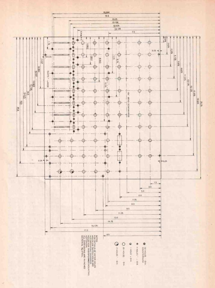
Fig. 11 Drilling details of front panel. The holes for the meters and slide switches should be cut to suit the type used.
