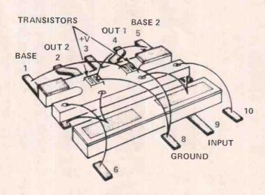
Fig. 1. The first integrated circuit developed by Texas instruments in 1959 used the "mesa" process. The device is a flip-flop and was the forerunner of the Resistor Transistor Logic family.
