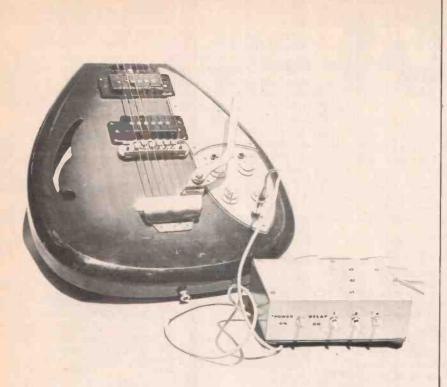
Completed prototype unit connected to guitar.
