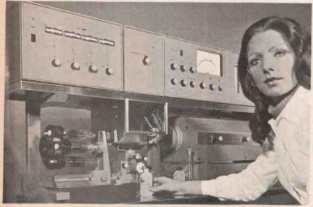
Fig. 8. An atomic-absorption flame spectrophotometer.
